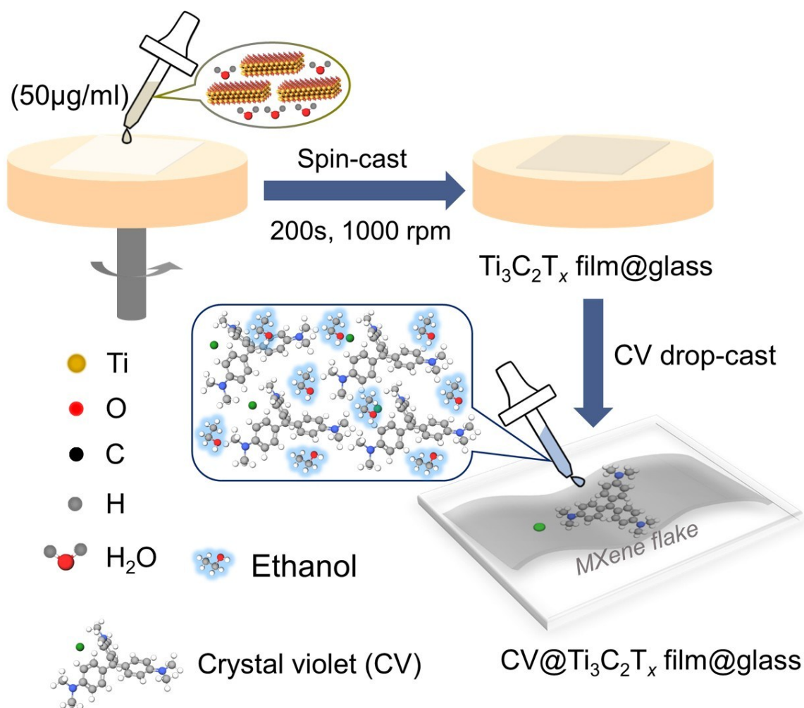
Figure S1. The graphical representation on fabrication of transparent SERS substrate based on thin film of \text{Ti}_3\text{C}_2\text{T}_x prepared onto the glass by spin-coating. An aqueous solution of delaminated \text{Ti}_3\text{C}_2\text{T}_x -MXene ( d\text{-Ti}_3\text{C}_2\text{T}_x ) flakes was used for the fabrication of SERS substrate and subsequent drop-casting of both resonant (dyes: Crystal violet–CV; Rhodamine 6G–R6G and Rose Bengal–RB) and non-resonant Raman probe molecules (para Nitrothiophenol– p\text{NTP} , para Amino thiophenol– p\text{ATP} , para hydroxy thiophenol– p\text{HTP} and para Mercapto benzoic acid– p\text{MBA} ).
