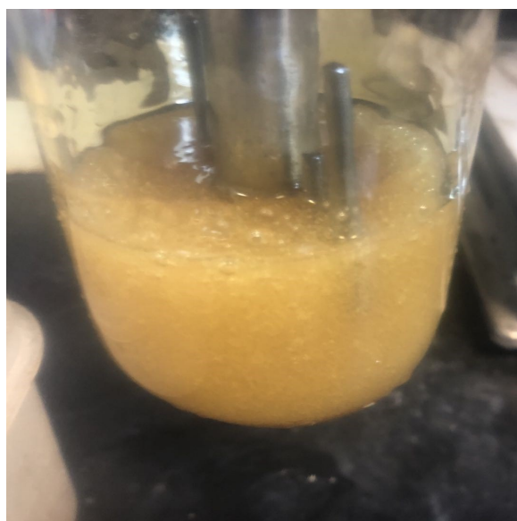
Fig. S1 Heterocyclic aromatic polyamide gel in reaction
