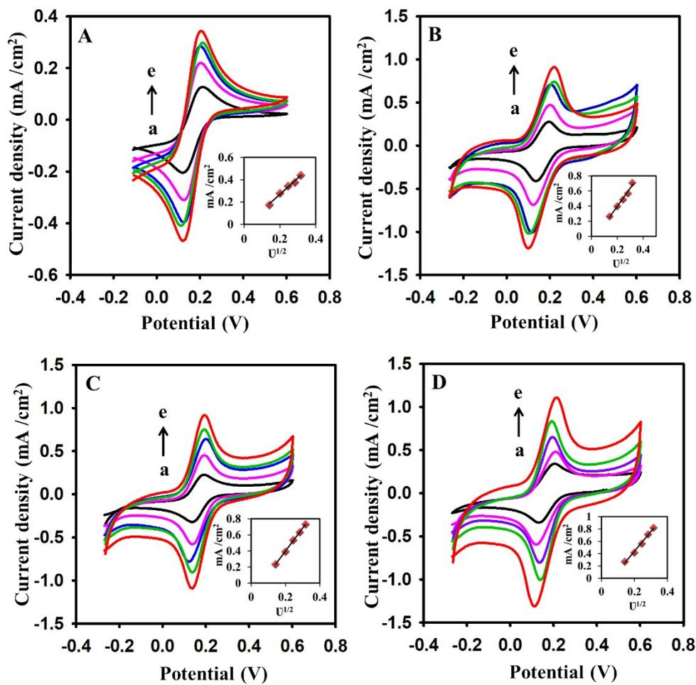
**Figure S2** Cyclic voltammograms of 2 mM  $K_3Fe(CN)_6/K_4Fe(CN)_6$  in 0.1 M KCl solution using (A) w-rGO/GPE, (B) pc-rGO/GPE, (C) pb-rGO/GPE, and (D) ac-rGO/GPE at scan rates of (a) 20, (b) 40, (c) 60, (d) 80, and (e) 100 mV/s. The insets in (A), (B), (C), and (D) show the linear relationship between current and the square root of the scan rates ( $v^{1/2}$ ).
