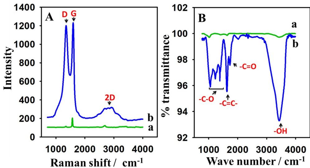
Figure S1 (A) Raman and (B) FTIR spectra of (a) graphite and (b) graphene oxide
