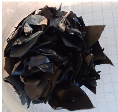
Figure S1. Scrapped electrode material from a HTC phone battery
