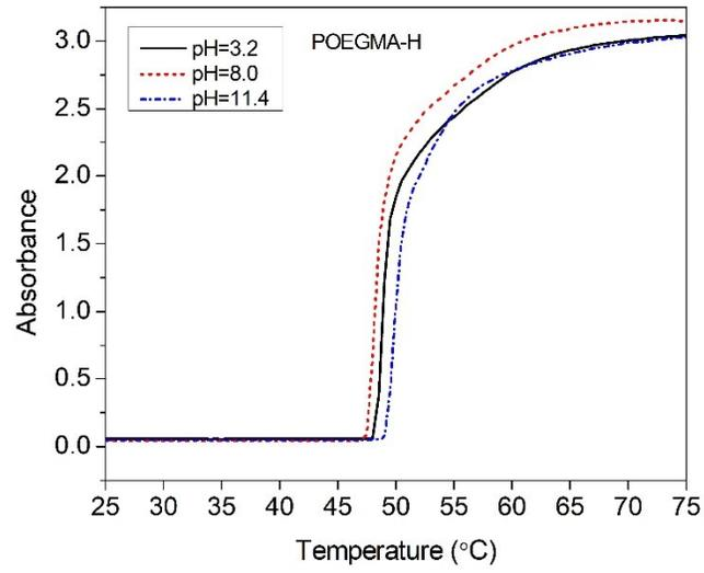
Figure S3. Effect of pH on phase transition of POEGMA-H aqueous solution (5 mg L<sup>-1</sup>).
