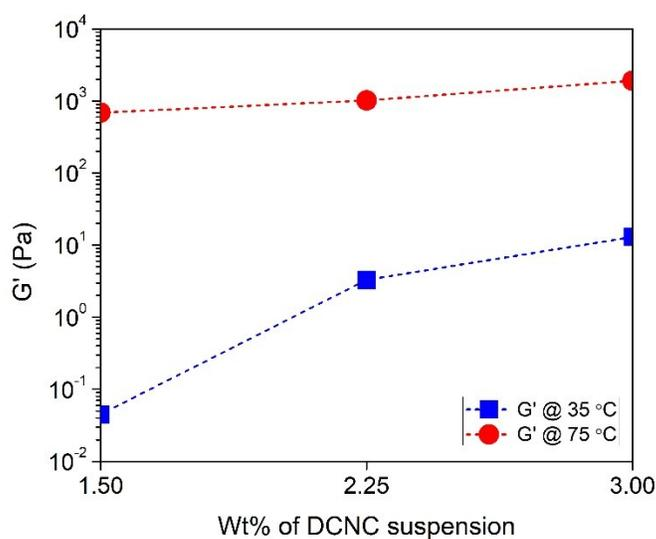
Figure S2. Effect of concentration of DACNC on the storage modulus of hydrogel before and after phase transitions.
