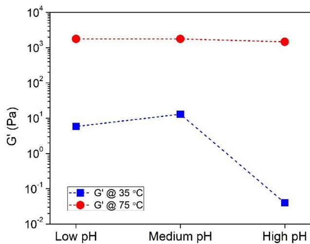
Figure S5. Effect of pH on the storage modulus of hydrogel before and after phase transitions.
