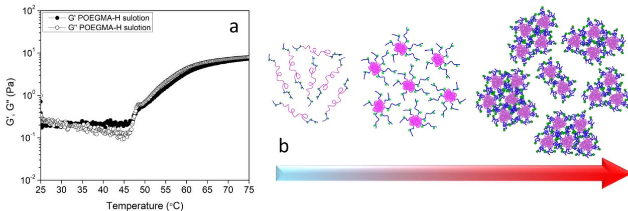
Figure S1. (a) Temperature sweep test of 20 wt % POEGMA-H aqueous solution at 1 Hz and 1 % strain. (b) Schematic representation of coil to globule transitions for middle and end blocks of POEGMA-H chains. Number of collapsed micelles presented in one cluster is more than what is shown here.
