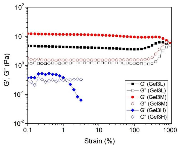
Figure S4. Linear viscoelastic region of Gel3L, Gel3M, and Gel3H at room temperature and 1Hz.
