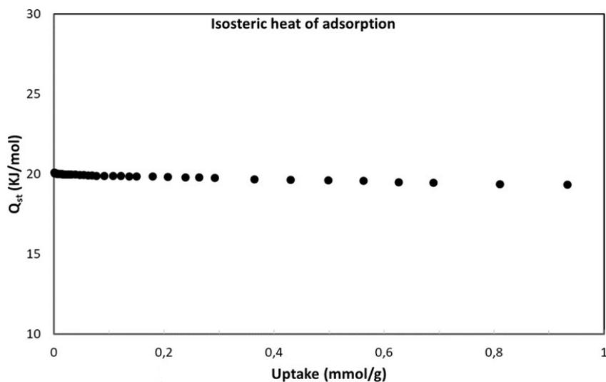
Figure S14: Isosteric heat of adsorption of NO at the MOF of this study at 298 K
