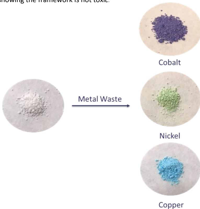
Figure S9: Picture showing the colour change of **NUIG1** (white) upon metal encapsulation.
