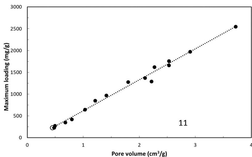
Figure S15: Maximum loading capacity of ibuprofen at different MOF structures as a function of Pore volume of the MOF.
