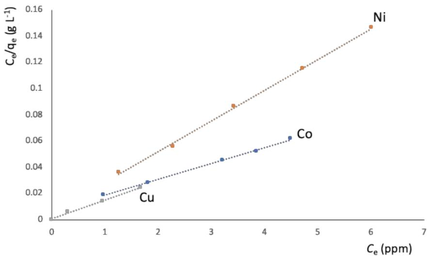
Figure S11: Fitting of the metal adsorption data to the Langmuir model.
