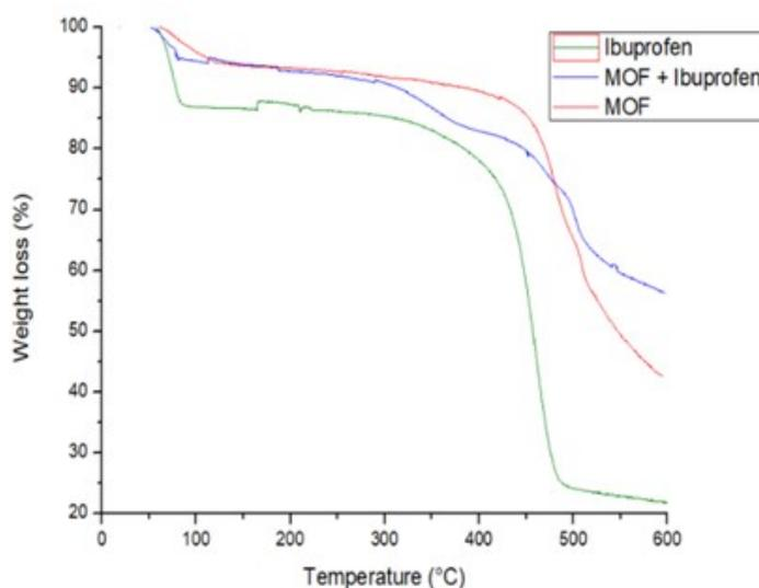
Figure S4: TGA showing the encapsulation of Ibu (in green), Ibu@**NUIG1** (in blue) and **NUIG1** (in red). The TGA plot of Ibu@**NUIG1** reveals an additional two-step mass loss between ca. 300 and 400°C, attributed to the decomposition of the drug. The drug uptake based on the TGA is
