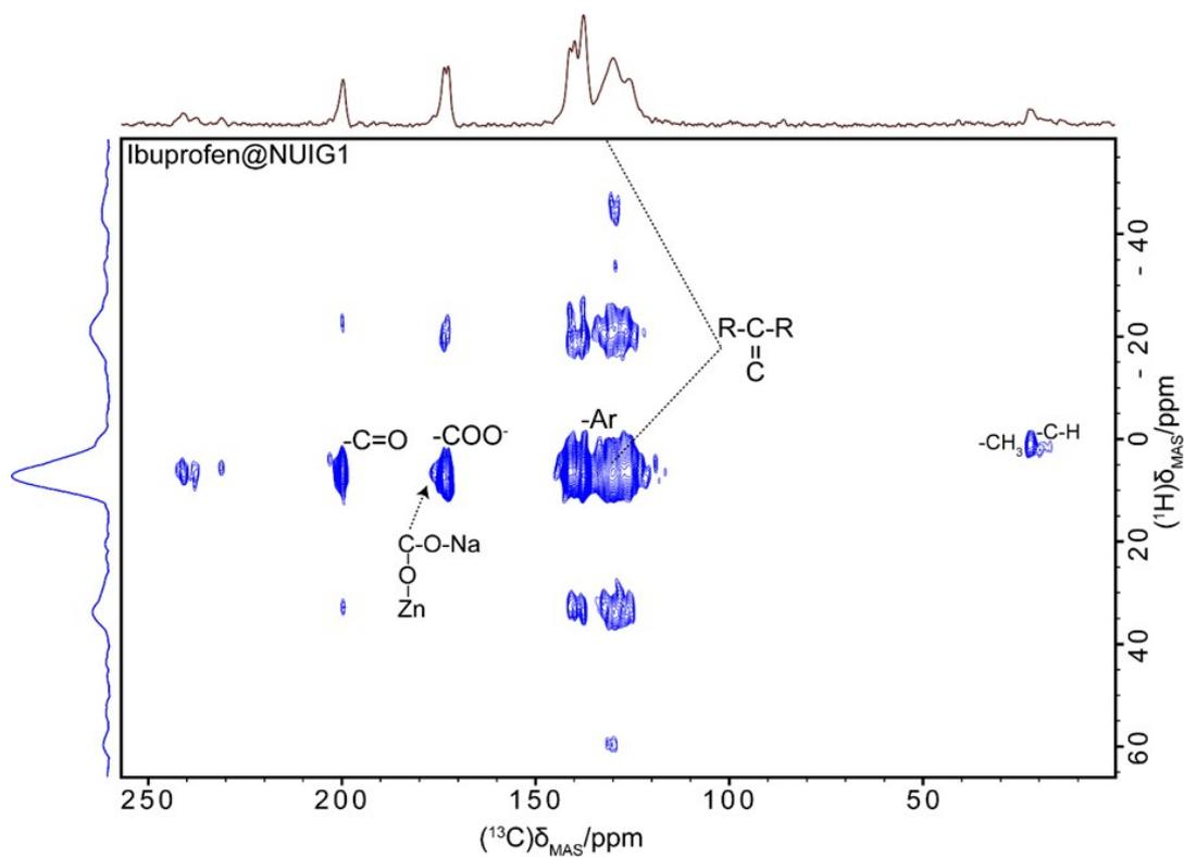
Figure S5: The 2-D  $^1\text{H} \rightarrow ^{13}\text{C}$  HETCOR spectrum for the Ibuprofen loaded **NUIG1** sample, correlating carbon shifts in the direct dimension to proton shifts in the indirect dimension. Not marked peaks are attributed to the spinning sideband manifold.
