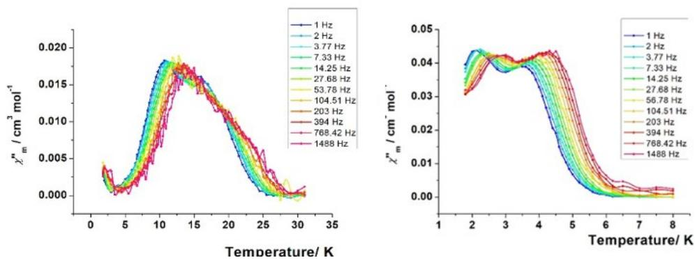
Figure S13: Representation of the  $\chi''_m$  for Co@NUIG1 (left), and Ni@NUIG1 (right) under 0 dc applied magnetic field.
