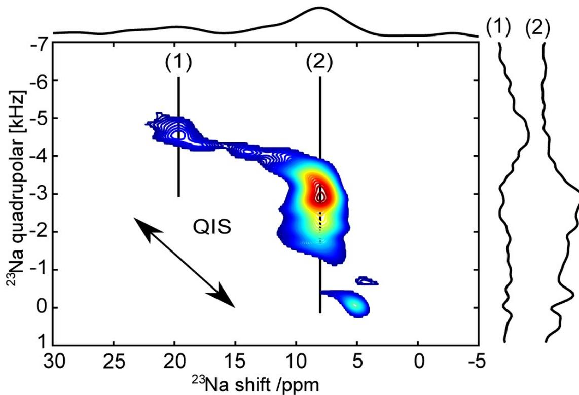
Figure S6: DQF-TOP-STMAS  $^{23}\text{Na}$  spectra of unloaded MOF. Similarly, to the loaded MOF, two separate resonances (1) and (2) can be identified. It is also possible to identify the sharp peak arising from the impurity signal which is not shifted by the QIS. The horizontal extracted slices of resonances (1) and (2) are also represented. The arrow indicates the direction of the QIS.
