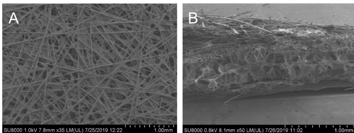
**Figure S5.** SEM images corresponding to the top (A) and cross-section (B) views of the CGDL material and the CGDL/biohydrogel/CGDL electrochemical cell respectively.
