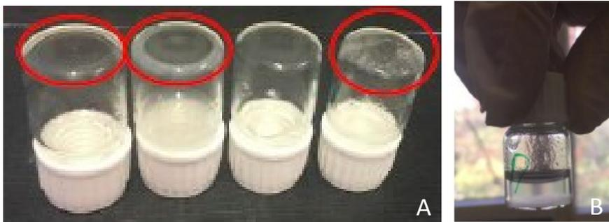
**Figure S3.** Results from the precipitation study. A) From left to right: samples A, B, C and D. B) Detail on precipitate formation in sample D identified as the product of the interactions between ChS and gelatin.
