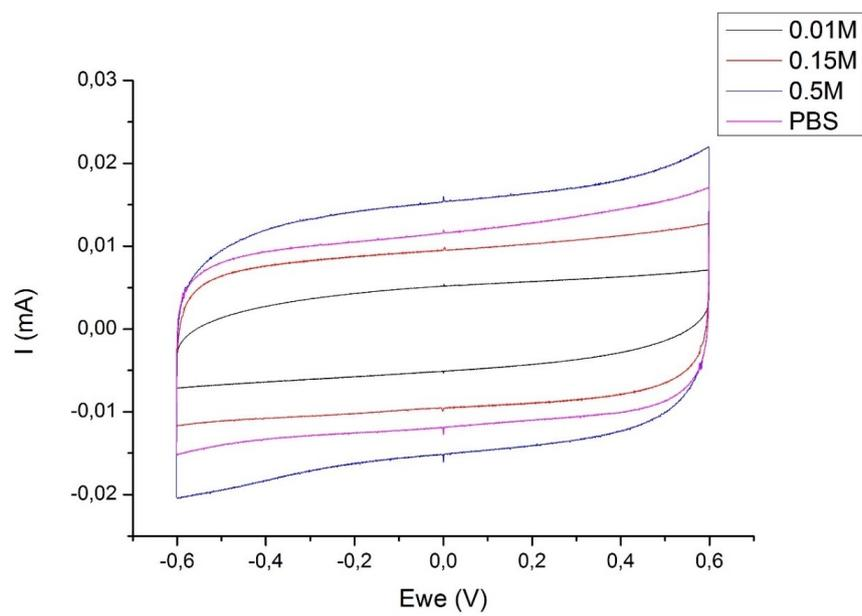
**Figure S8.** CVs of CGDL/biohydrogel/CGDL cell measured at 100 mV.s<sup>-1</sup> in a symmetric configuration.
