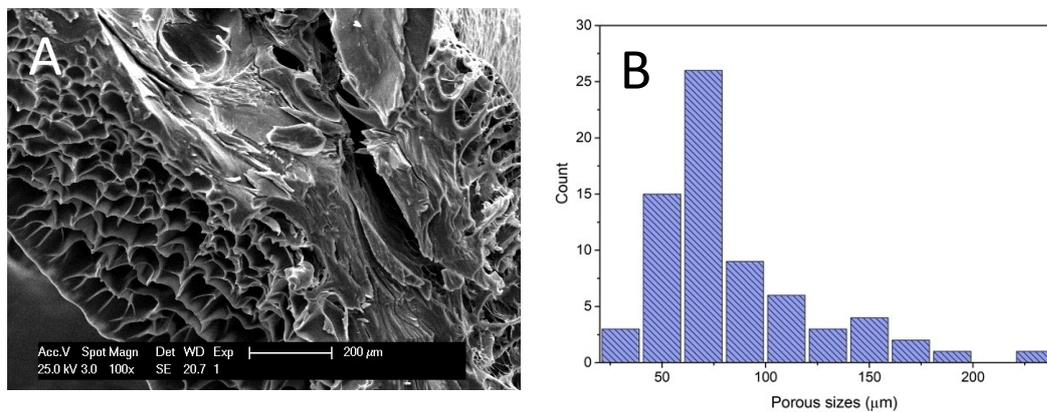
**Figure S6.** A. Representative SEM image corresponding to ChS-gelatin hydrogel. B. Analysis of the pore size distribution carried out with the software ImageJ.
