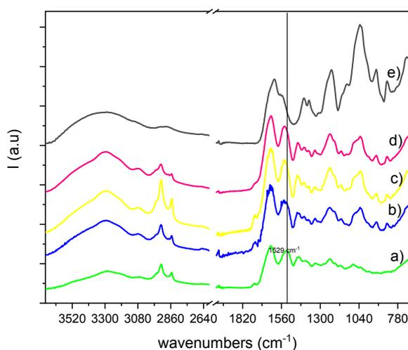
**Figure S4.** ATR-FTIR spectra corresponding to a) gelatin; b) sample A; c) sample B; d) sample D and e) ChS.
