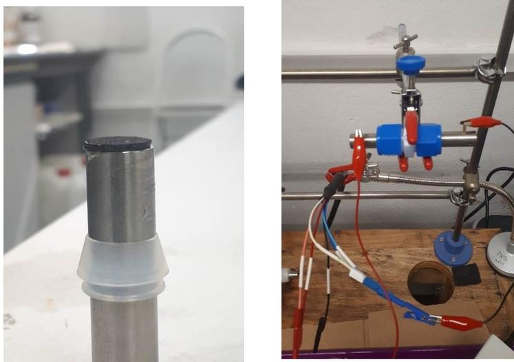
**Figure S7.** Left: Photograph corresponding to a CGDL/biohydrogel/CGDL electrochemical cell; Right: assembly of the electrochemical cell onto a Swagelok type cell with a symmetric configuration.
