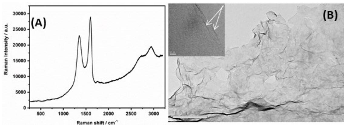
**Figure S1.** Characterization of GO employed in this work: a) Raman spectrum and b) transmission electron microscopy of drop-casted flakes. The inset represents a HRTEM image of the edges of the GO flakes (white arrows indicate the edges, in this case of a bilayer).
