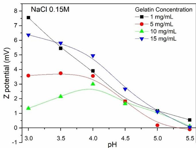
**Figure S2.** Representation of Z-potential as a function of pH for aqueous solutions of gelatin at different concentrations.
