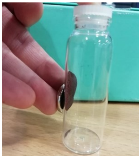
Fig. S2. Magnet placed next to FS-processed \text{Fe}_3\text{O}_4 : \text{CaCO}_3 , following sieving, demonstrating the \text{Ca}_2\text{Fe}_2\text{O}_5 microsphere products to be magnetic.
