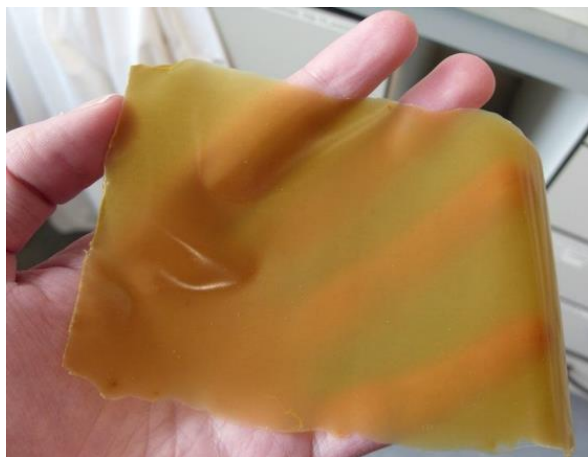
Figure S6: Photograph of as-prepared, stand-alone CPO-27 (Ni)-containing polyurethane film.
