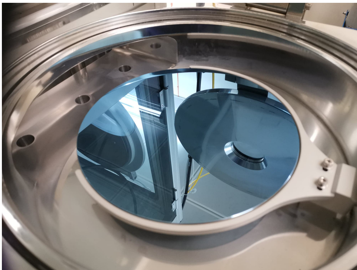
Figure S1: A 20 nm NiO film grown onto an 8" Si wafer with a 100 nm thermal oxide layer wafer at 250 °C using the 2 s/5 s/2 s/5 s optimised pulse sequence
