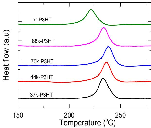
**Figure S1:** Second heating heat-flow curves of the different pristine P3HT samples obtained from DSC measurement.
