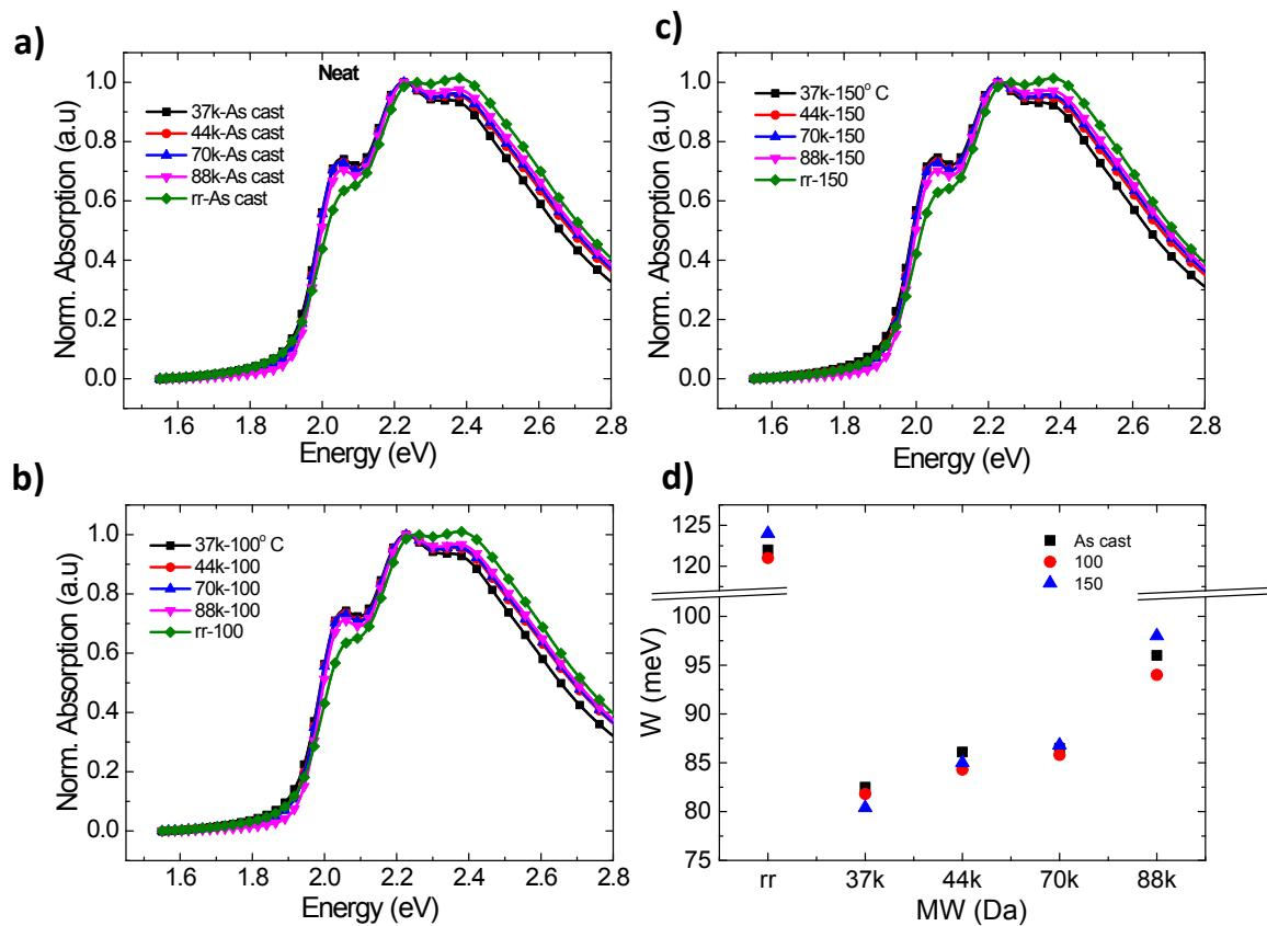
**Figure S2:** Normalized UV-Vis absorption spectrum at 0-1 peak of pristine P3HT polymers over glass substrate a) as-cast, b) 100 °C for 10 min and c) 150 °C for 10 min and d) represents the value of  $W$  with respect to different MW.
