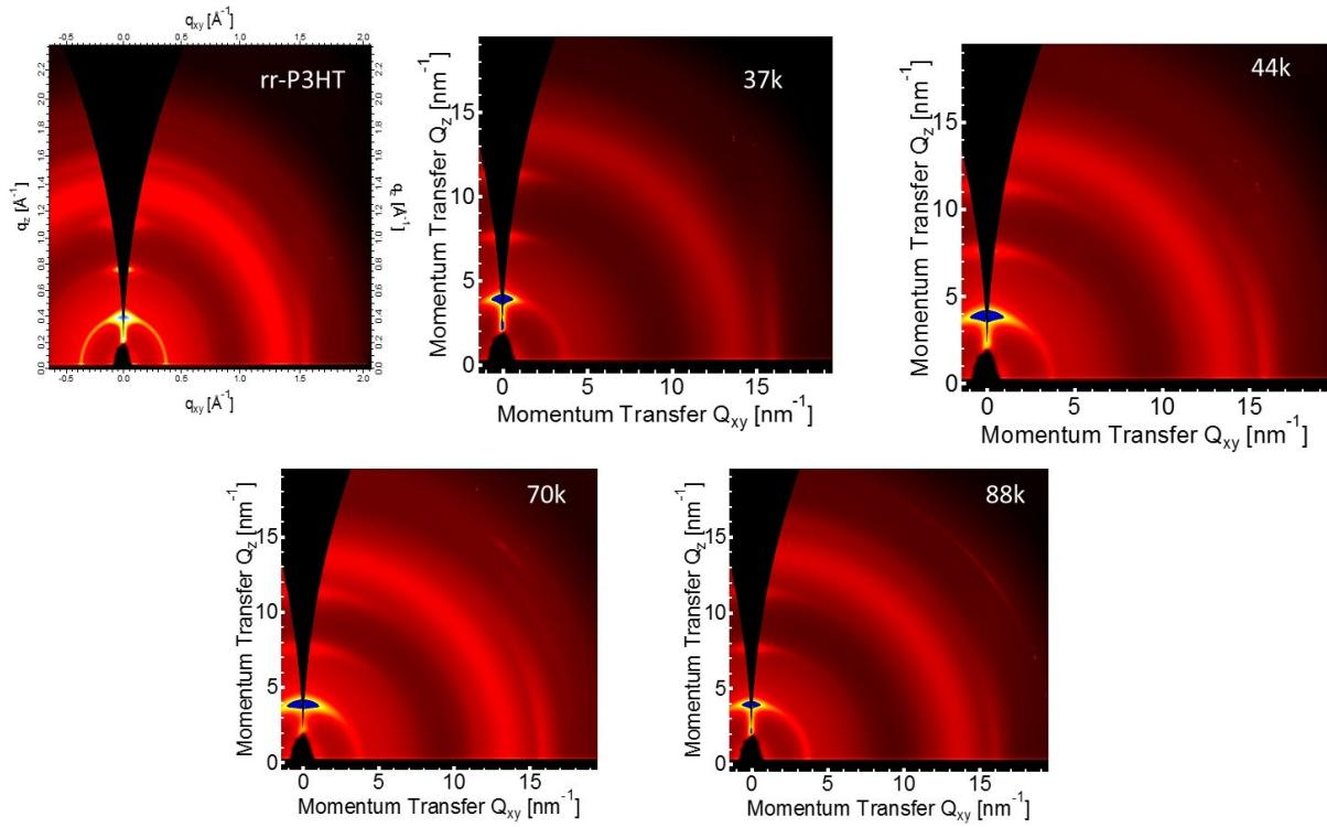
**Figure S7:** Two-dimensional GIWAXS image of as-cast P3HT:PCBM blend films.
