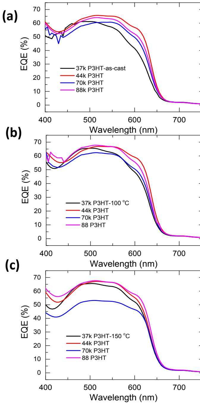
**Figure S11:** External quantum efficiency (EQE) plots of different MW P3HT at **a)** as-cast **b)** 100 °C and **c)** 150 °C.
