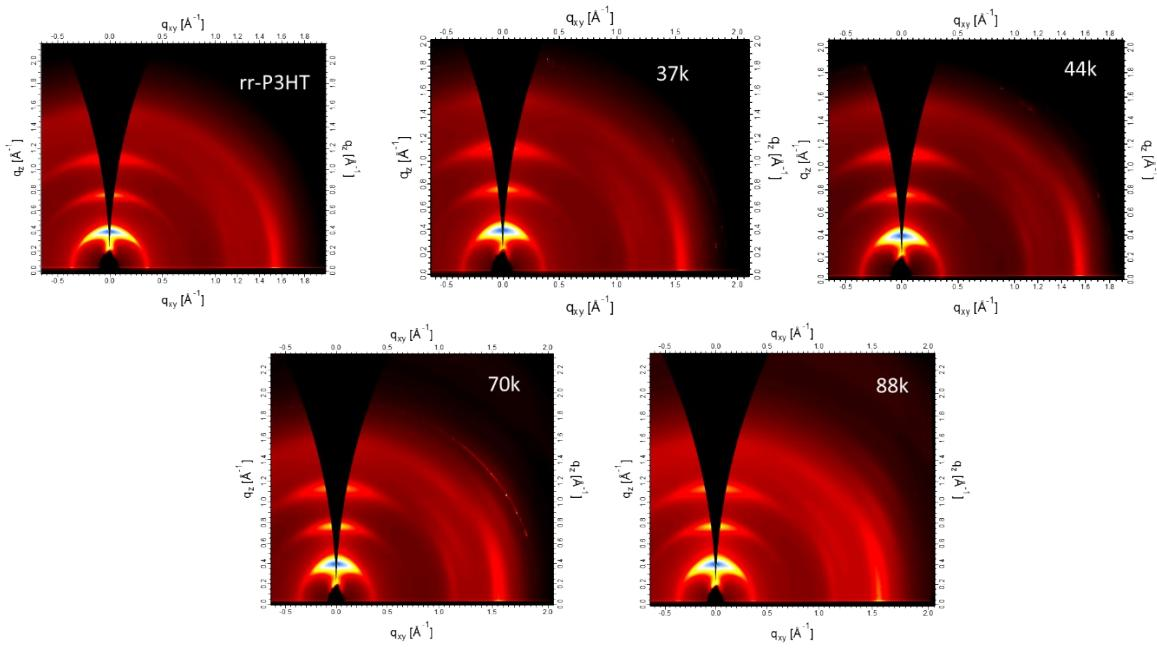
**Figure S3:** Two-dimensional GIWAXS image of as-cast pristine-P3HT films.
