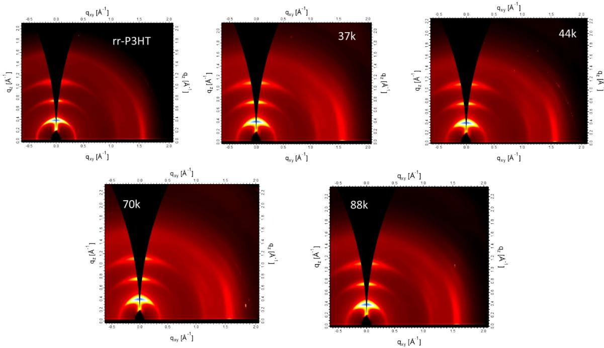
**Figure S4:** Two-dimensional GIWAXS image of pristine-P3HT films annealed at 150 °C for 10 min.
