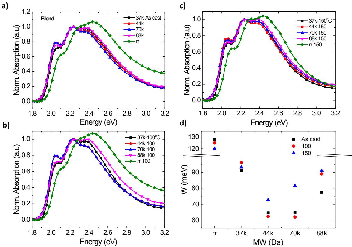
**Figure S5:** Normalized (0-1 peak) UV-Vis absorption spectrum of P3HT:PCBM blends over glass substrate a) as-cast, b) 100 °C, c) 150 °C, and d) represents the value of  $W$  with respect to different MW.
