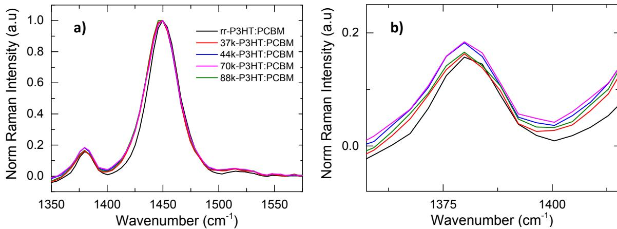
**Figure S6:** Resonant Raman spectra of different as-cast P3HT:PCBM polymer blends with 532 nm wavelength excitation. a) Raman spectra normalized with C=C stretching peak maximum intensity. b) Zoomed plot of normalized Raman spectra highlighting the height of C-C intra-ring stretching Raman mode
