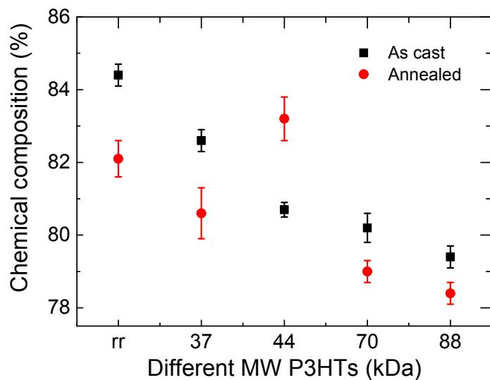
**Figure S9:** Surface chemical composition of P3HT on the top surface of the P3HT:PCBM blends extracted from the NEXFAS spectra.
