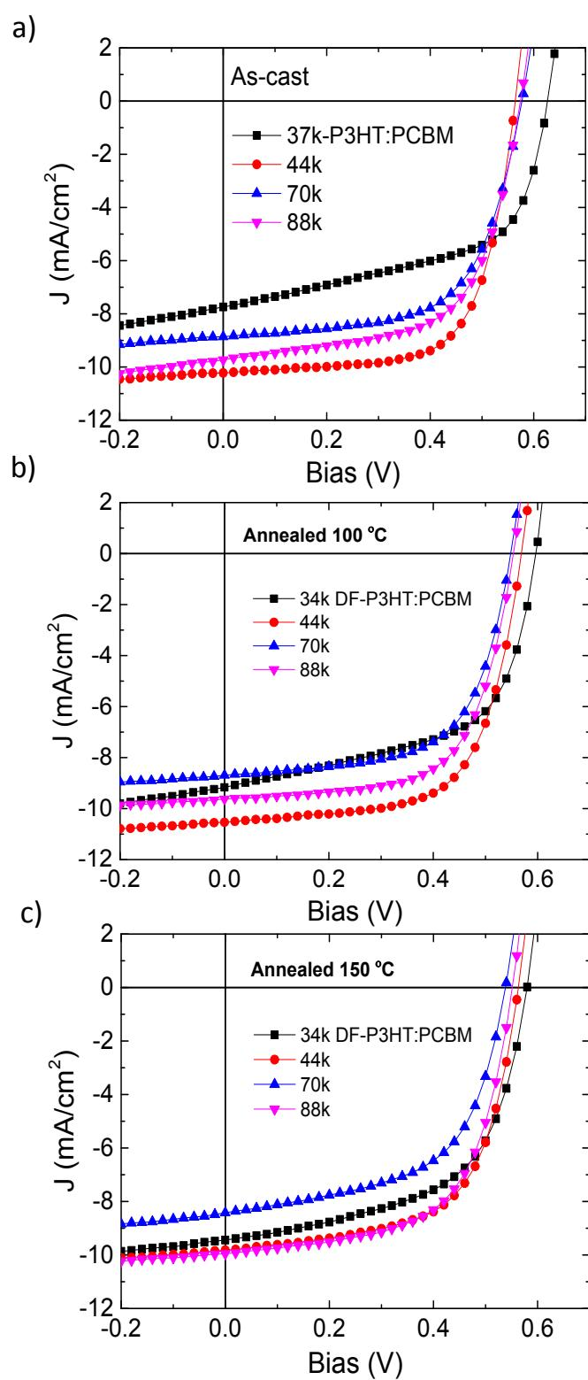
**Figure S10:** Light illuminated J-V characteristics of different P3HT:PCBM solar cells with different annealing conditions a) as-cast; b) thermal annealed at 100 °C for ten minutes, and c) thermal annealed at 150 °C for ten minutes.
