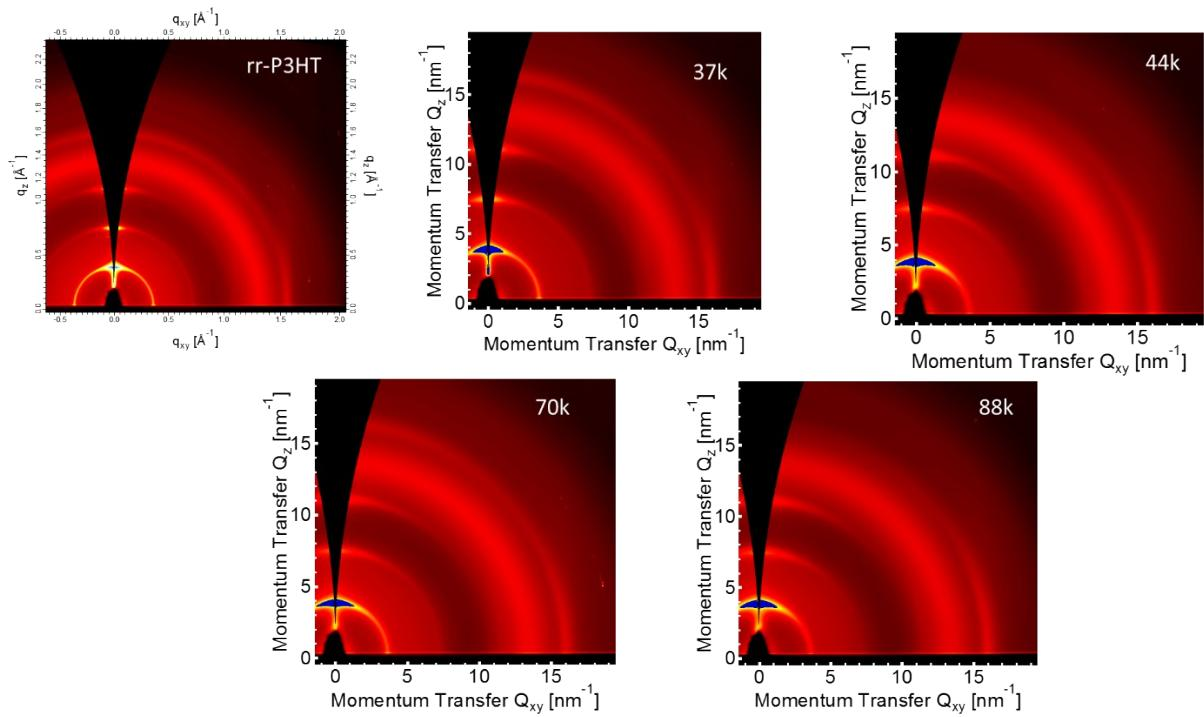
**Figure S8:** Two-dimensional GIWAXS image of P3HT:PCBM blend films annealed at 150 °C for 10 min.
