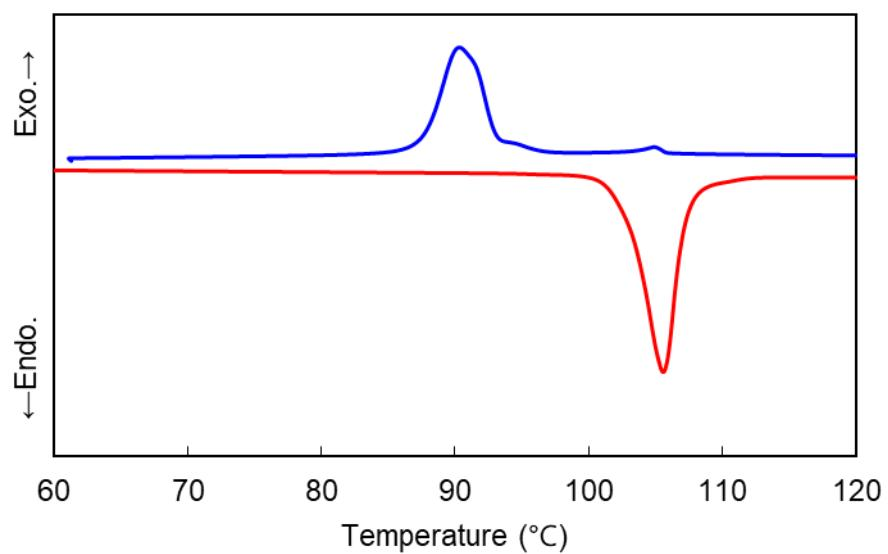
**Fig. S12.** DSC curves of CBCOO10SCB upon 1st heating and cooling at a rate of  $10\text{ }^{\circ}\text{C min}^{-1}$ .
