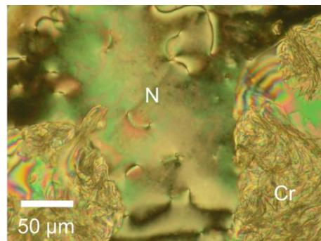
**Fig. S6.** POM image of CBOCO2SCB in a non-treated glass cell; the N phase accompanied by crystallization at 133 °C.
