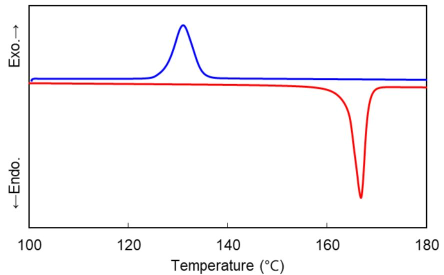
**Fig. S13.** DSC curves of CBOCO<sub>2</sub>SCB upon 1st heating and cooling at a rate of  $10\text{ }^{\circ}\text{C min}^{-1}$ .
