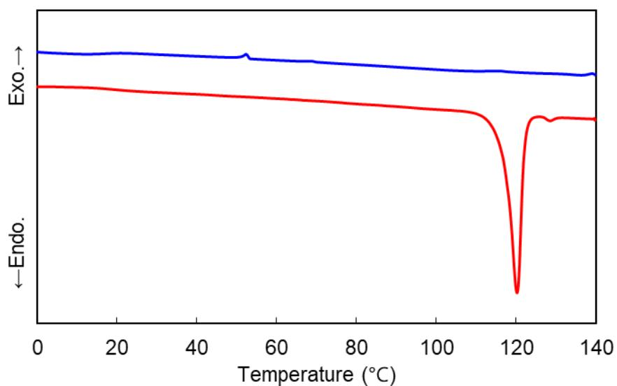
**Fig. S10.** DSC curves of CBCOO<sub>4</sub>SCB upon 1st heating and cooling at a rate of 10 °C min<sup>-1</sup>, which was reproduced from ref. S1 with permission from Elsevier.
