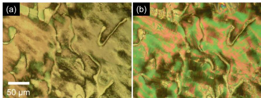
**Fig. S7.** POM images of CBOCO8SCB in a non-treated glass cell; (a) the N phase at 95 °C and (b) the N<sub>TB</sub> phase at 87 °C.
