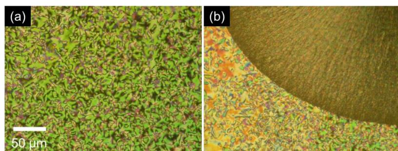
**Fig. S1.** POM images of  $\text{CBOCO}_2\text{SCB}$  in a non-treated glass cell; (a) the N phase at 75 °C and (b) the N phase accompanied by crystallization at 75 °C.
