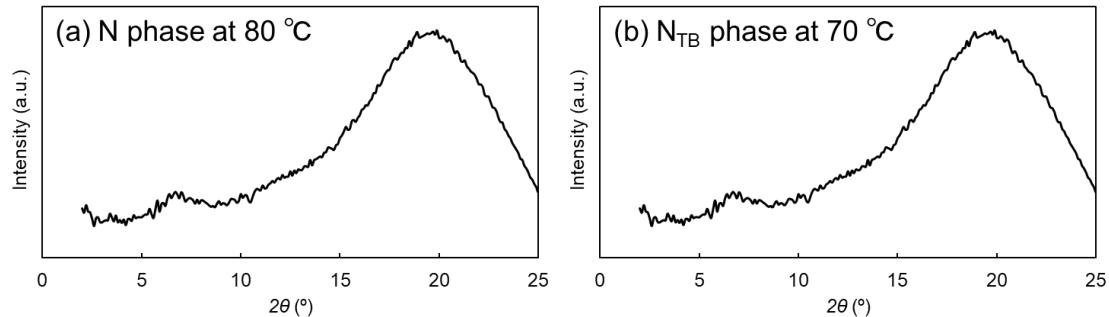
**Fig. S19.** 1D-XRD profiles of CBCOO<sub>6</sub>SCB; (a) the N phase at 80 °C, and (b) the  $N_{TB}$  phase at 70 °C.
