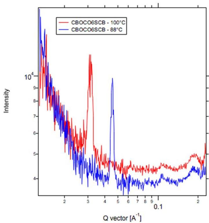
**Fig. S27.** 1D-TReXS profiles of CBOCO6SCB.
