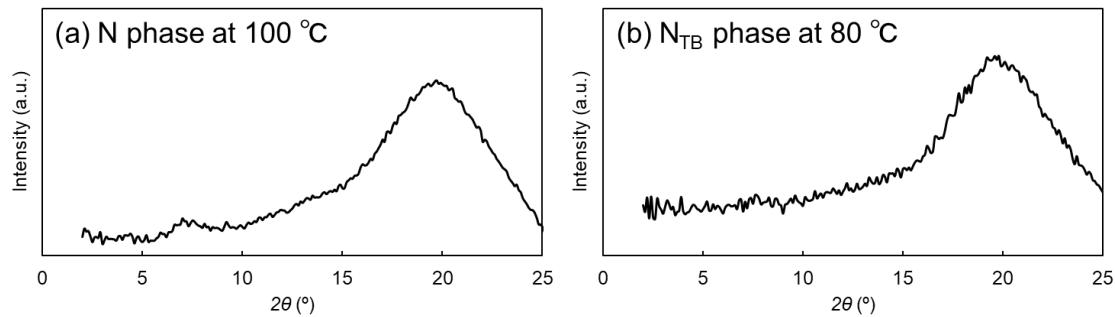
**Fig. S20.** 1D-XRD profiles of CBOCO<sub>4</sub>SCB; (a) the N phase at 100 °C, and (b) the  $N_{TB}$  phase at 80 °C.
