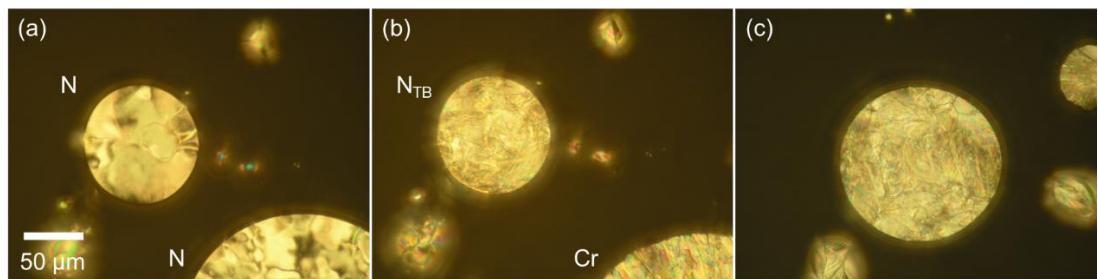
**Fig. S8.** POM images of CBOCO10SCB in a non-treated glass cell; (a) the N phase at 100 °C, (b) the N<sub>TB</sub> phase at 70 °C, and (c) the N<sub>TB</sub> phase at 69 °C.
