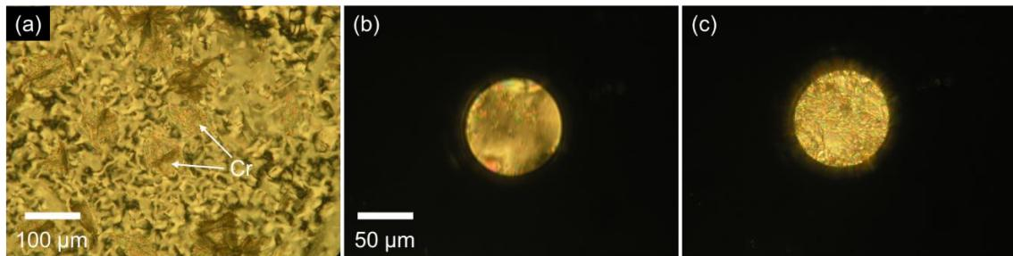
**Fig. S5.** POM images of CBCOO10SCB in a non-treated glass cell; (a) the N phase at 97 °C, (b) the N phase at 100 °C, and (c) the N<sub>TB</sub> phase at 75 °C.
