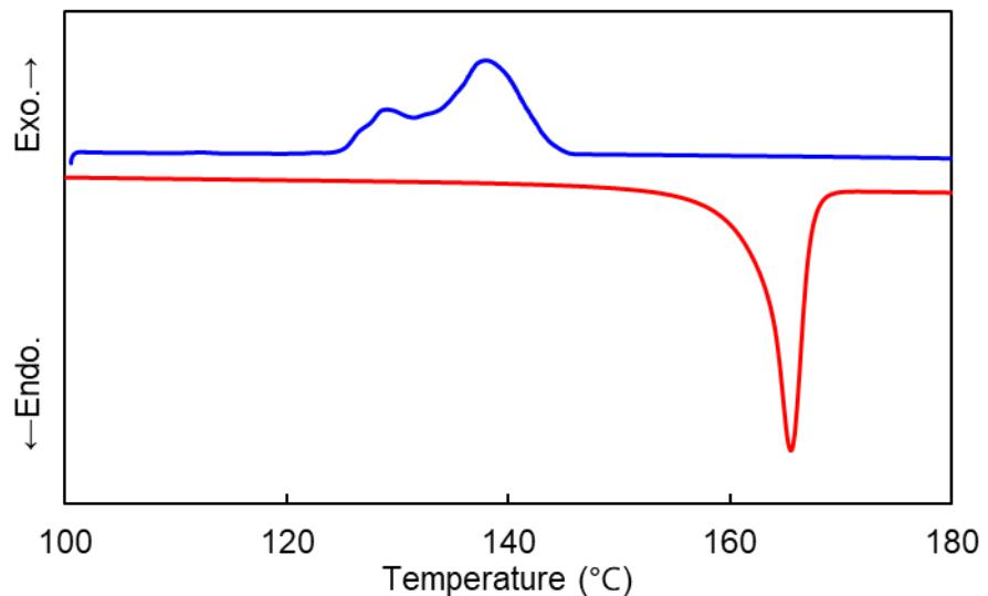
**Fig. S9.** DSC curves of CBCOO2SCB upon 1st heating and cooling at a rate of 10 °C min<sup>-1</sup>.
