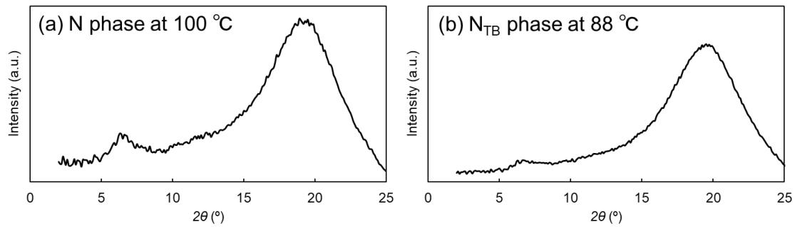
**Fig. S21.** 1D-XRD profiles of CBCOO6SCB; (a) the N phase at 100 °C, and (b) the N<sub>TB</sub> phase at 88 °C.
