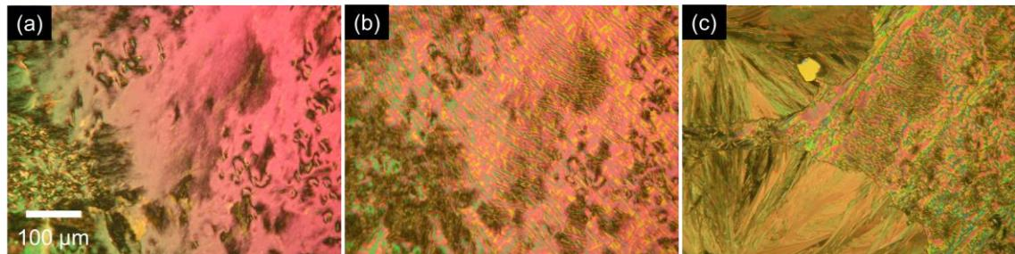
**Fig. S3.** POM images of CBCOO8SCB in a non-treated glass cell; (a) the N phase at 90 °C, (b) the  $N_{TB}$  phase at 83 °C, and (c) the  $N_{TB}$  phase accompanied by crystallization at 70 °C.
