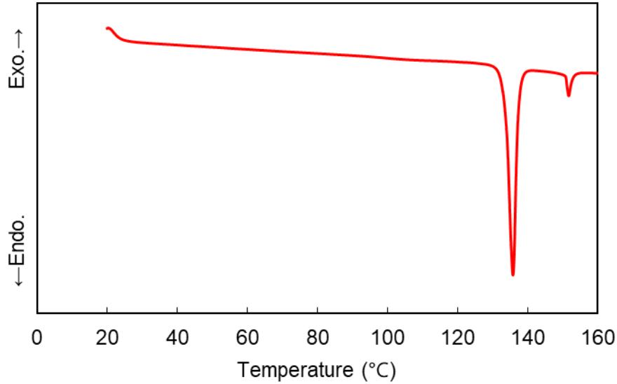
**Fig. S15.** DSC curves of CBOCO6SCB upon 1st heating at a rate of  $10\text{ }^{\circ}\text{C min}^{-1}$ .
