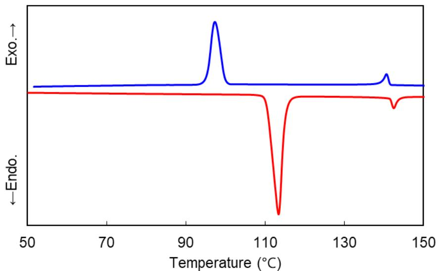
**Fig. S17.** DSC curves of CBOCO10SCB upon 1st heating and cooling at a rate of  $10\text{ }^{\circ}\text{C min}^{-1}$ .
