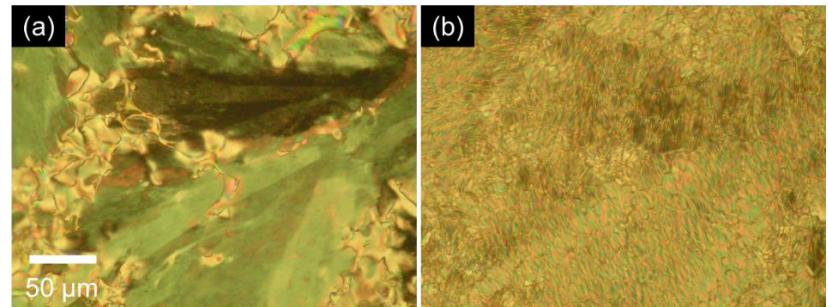
**Fig. S2.** POM images of CBCOO6SCB in a non-treated glass cell; (a) the N phase at 80 °C and (b) the  $N_{TB}$  phase at 58 °C.
