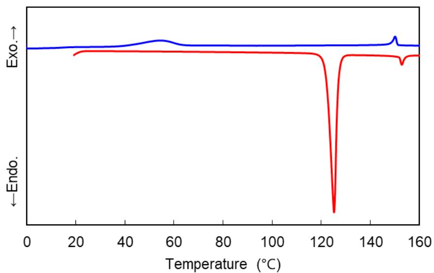
**Fig. S14.** DSC curves of CBOCO4SCB upon 1st heating and cooling at a rate of  $10\text{ }^{\circ}\text{C min}^{-1}$ , which was reproduced from ref. S1 with permission from Elsevier.
