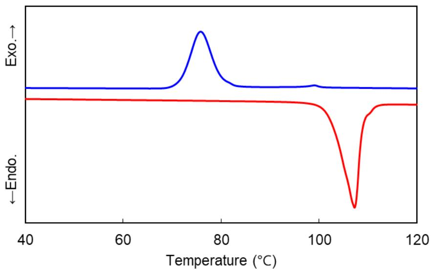
**Fig. S11.** DSC curves of CBCOO<sub>8</sub>SCB upon 1st heating and cooling at a rate of 10 °C min<sup>-1</sup>.
