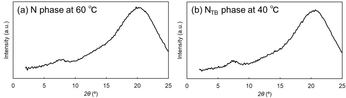
**Fig. S18.** 1D-XRD profiles of CBCOO<sub>4</sub>SCB; (a) the N phase at 60 °C, and (b) the  $N_{TB}$  phase at 40 °C.
