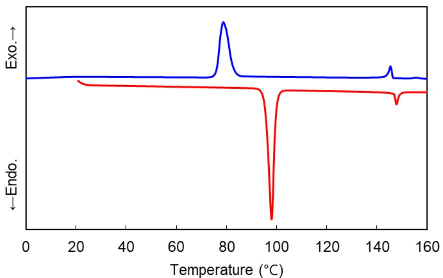
**Fig. S16.** DSC curves of CBOCO8SCB upon 1st heating and cooling at a rate of  $10\text{ }^{\circ}\text{C min}^{-1}$ .
