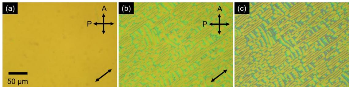
**Fig. S4.** POM images of CBCOO8SCB in a uniaxially rubbed polyimide-surface glass cell; (a) the N phase at 85 °C, (b) the  $N_{TB}$  phase at 82 °C, and (c) the  $N_{TB}$  phase at 77 °C. The double-headed arrows represent the rubbing direction.
