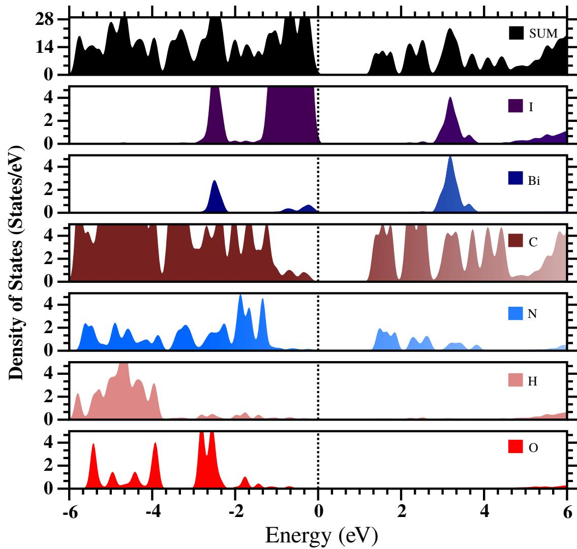
Figure S24: Density of states obtained with PBE+D3 for perovskite 3. The fundamental band gap is 1.406 eV.
