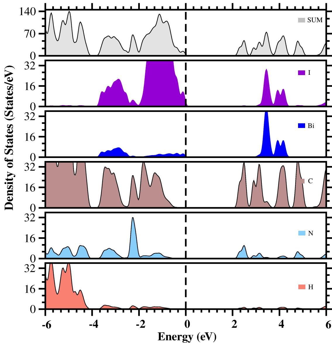
Figure S26: Density of states obtained with HSE06 for perovskite 2. The fundamental band gap is of 2.3525 eV
