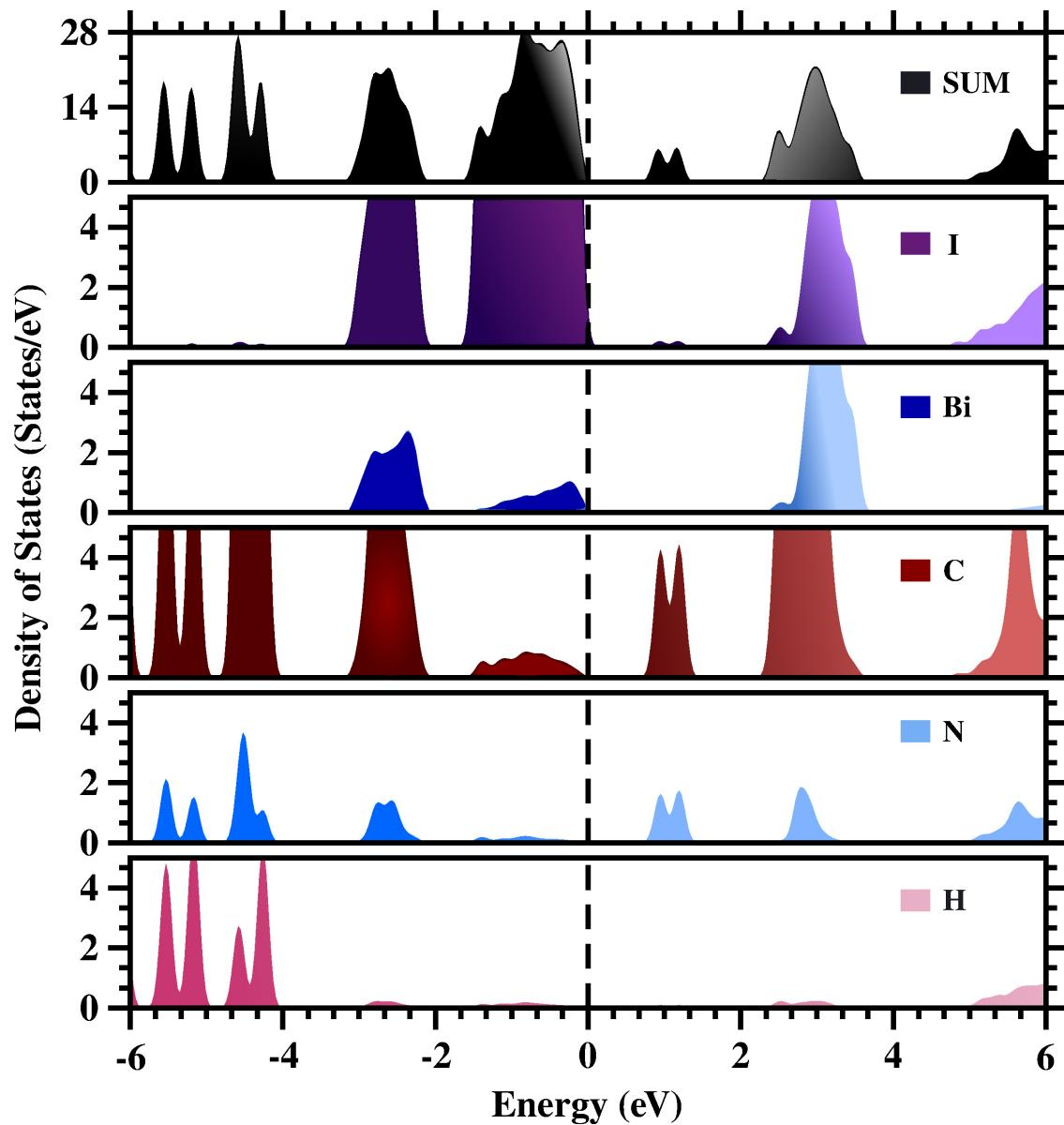
Figure S22: Perovskite 1: ( $C_{20}H_{20}N_4Bi_2I_{10}$ ) Density of states obtained with PBE+D3. Fundamental band gap is 0.9802 eV.
