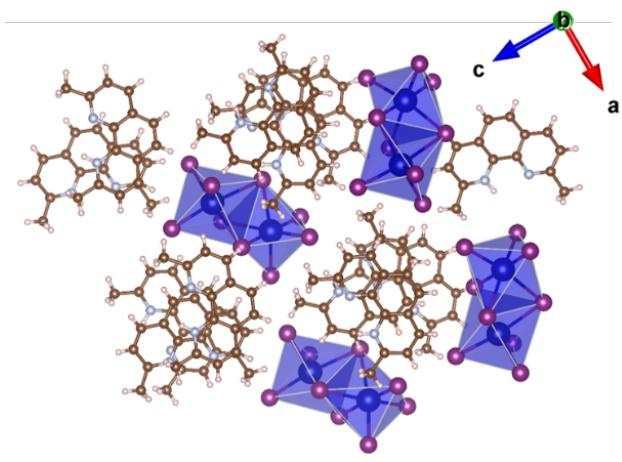
Figure S10: Crystal packing of 2 along crystallographic *b* axis, showcasing the  $\pi$ -stacking of Hdmphen<sup>+</sup> in a twisted arrangement.
