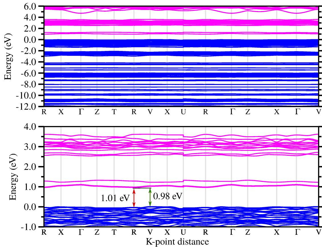
Figure S28: Band structure of perovskite 1 obtained with PBE+D3. The indirect fundamental band gap is 0.9756 eV with the top of valence band at V point and the bottom of conduction band at R point. The direct fundamental band gap is 1.0143 eV and occurs at R point.
