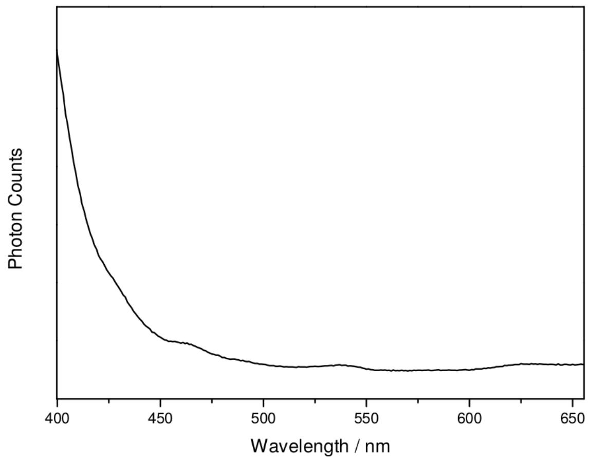
Figure S5: Photoluminescence spectra of 2 perovskite in thin film.
