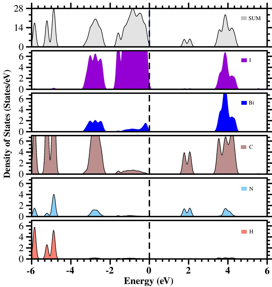
Figure S25: Density of states obtained with HSE06 for perovskite 1. The fundamental band gap is of 1.8004 eV
