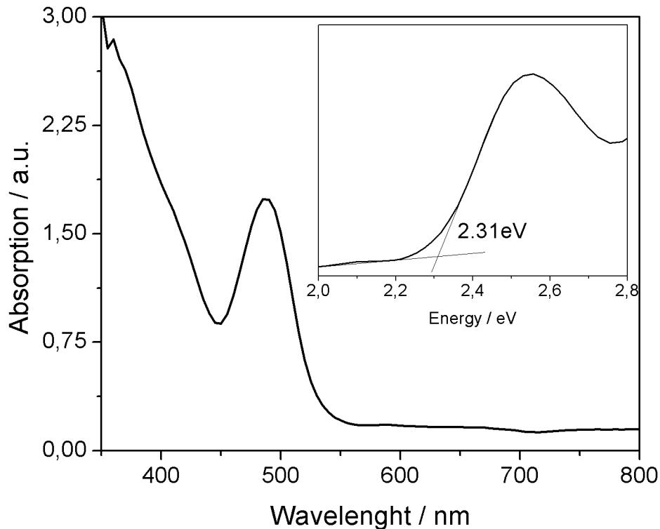
Figure S1: UV-vis absorption spectra of the 1 perovskite in thin film. Inset is direct optical band gap obtained by the Tauc plot for an direct allowed transition.
