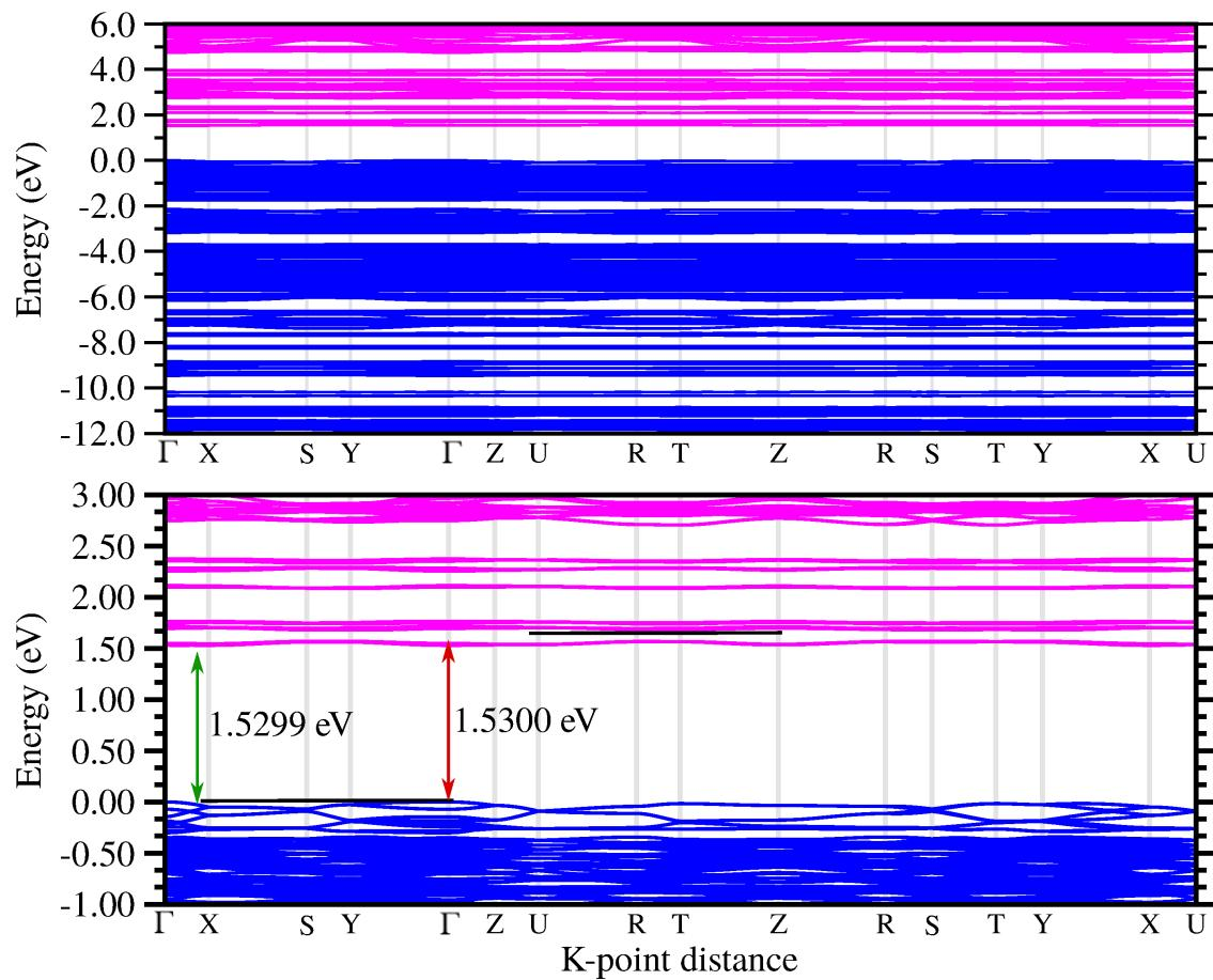
**Figure S29:** Band structure of perovskite 2 obtained with PBE+D3. The indirect fundamental band gap is of 1.53 eV with the top of valence band at  $\Gamma$  point and the bottom of conduction band in three degenerated points located between the path of  $\Gamma$  and X. The fundamental direct band gap is 1.53 eV and occurs at  $\Gamma$  point.
