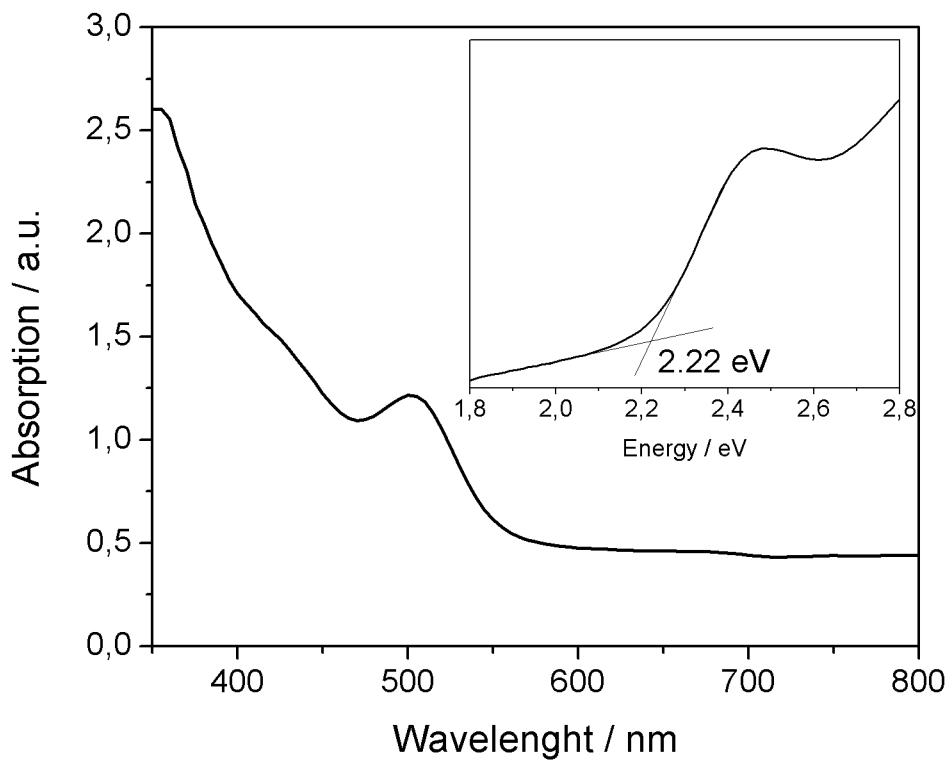
**Figure S3:** UV-vis absorption spectra of 3 perovskite in thin film. Inset is direct optical band gap obtained by the Tauc plot for an direct allowed transition.
