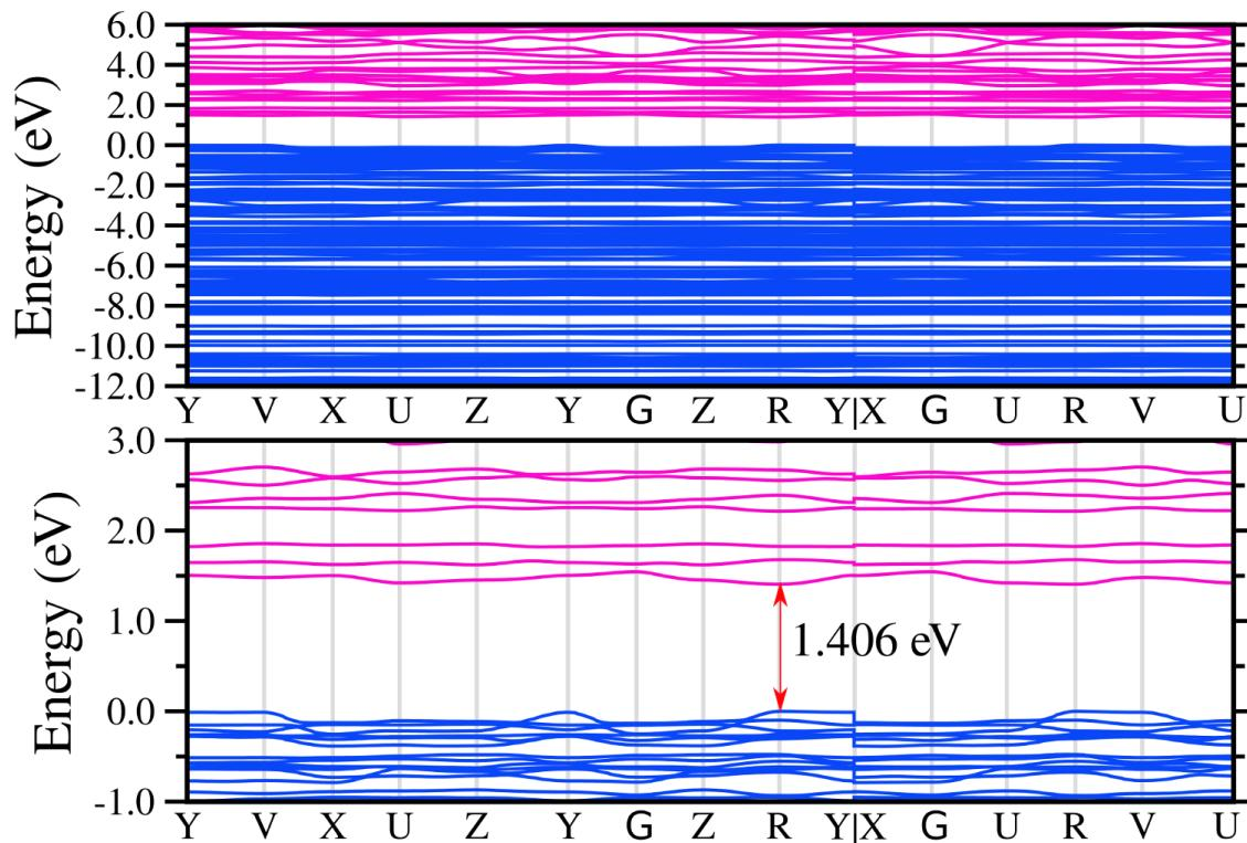
**Figure S30:** Band structure of perovskite 3 obtained with PBE+D3. Direct fundamental band gap of 1.406 eV at R point.
