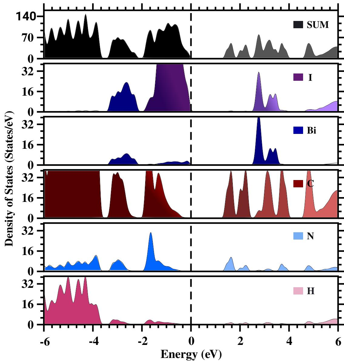
Figure S23: Density of states obtained with PBE+D3 for Perovskite 2. The fundamental band gap is 1.5300 eV.
