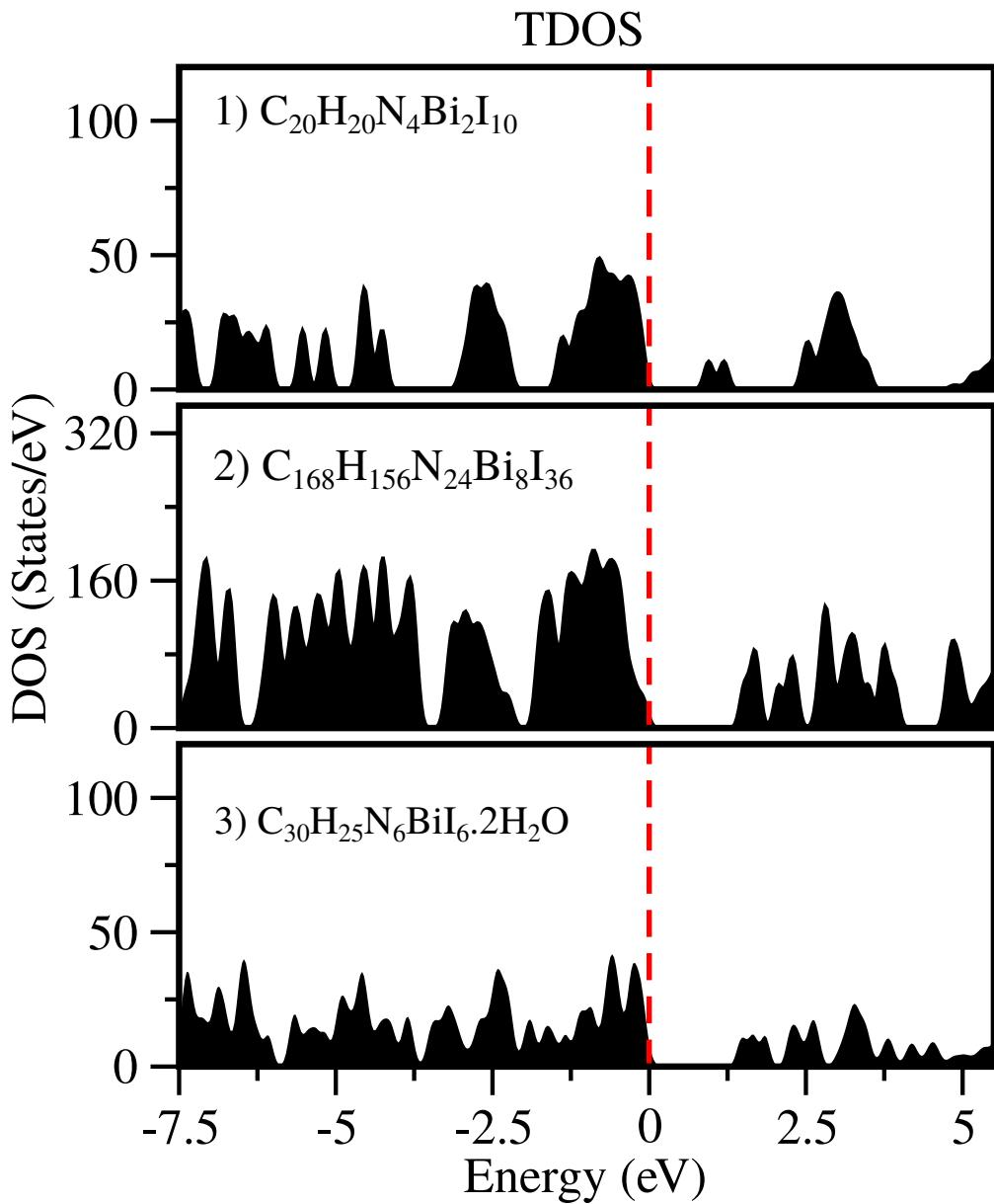
Figure S21: Total density of states (TDOS) for PBE+D3 optimized 1, 2, and 3 hybrid-perovskites. The fundamental band gap obtained in this calculations are (i) 1 = 0.9802 eV (ii) 2 = 1.5300 eV, and (iii) 3 = 1.406 eV.
