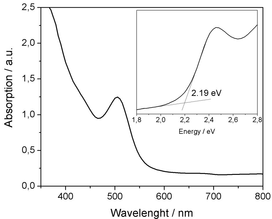
Figure S2: UV-vis absorption spectra of 2 perovskite in thin film. Inset is direct optical band gap obtained by the Tauc plot for an direct allowed transition.
