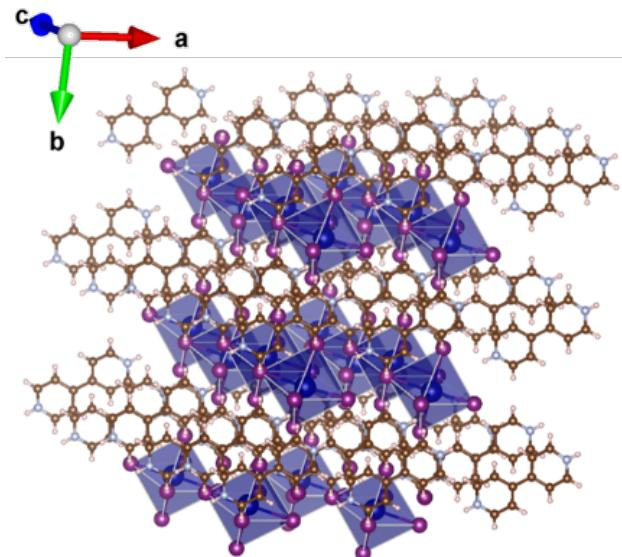
Figure S9: Crystal packing of 1 featuring the pseudo-2D perovskite like structure.
