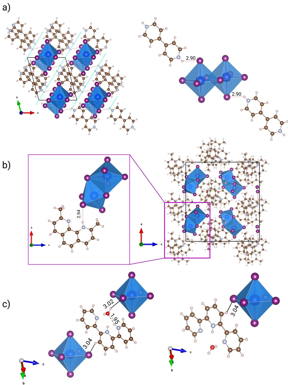
**Figure S8:** The lowest distance between iodine-hydrogen (hydrogen bonds) in the experimental a) 1, b) 2, and c) 3 perovskites.
