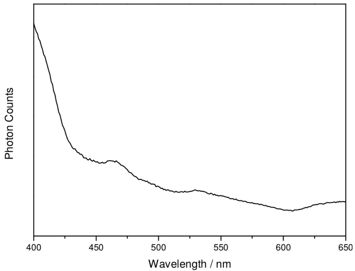
Figure S6: Photoluminescence spectra of 3 perovskite in thin film.
