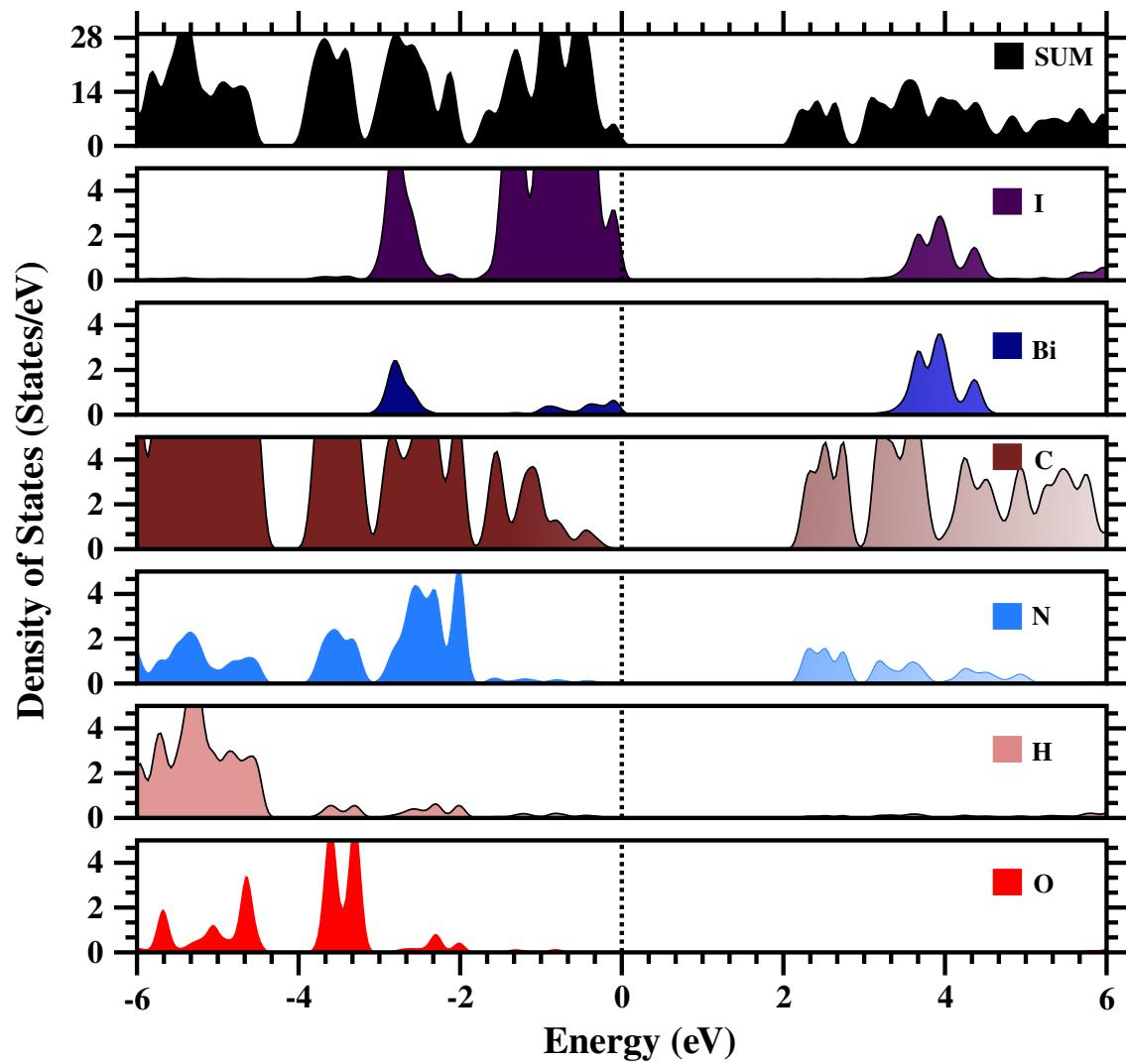
Figure S27: Density of states obtained with HSE06 for perovskite 3. The band gap is 2.24 eV
