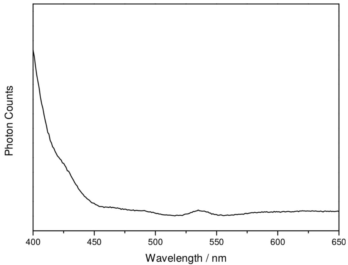
Figure S4: Photoluminescence spectra of 1 perovskite in thin film.
