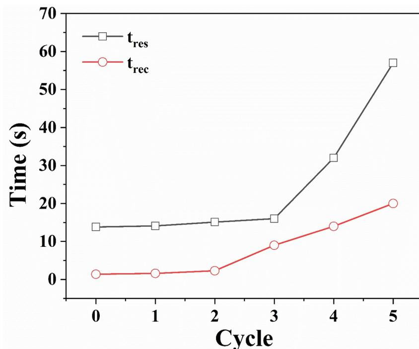
Figure S8. The response and recovery time of the humidity sensitive detector under multiple cycles of heat treatment.
