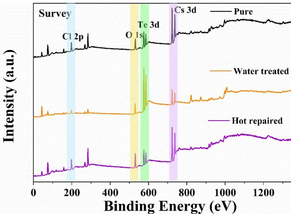
Figure S10. XPS survey scan spectra of  $\text{Cs}_2\text{TeCl}_6$  before and after heat treatment.
