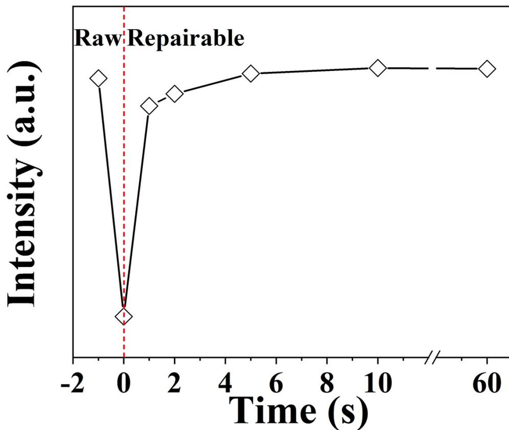
Figure S11. The time-dependent luminescence intensity of the sample under 365nm excitation for HCl gas treatment.
