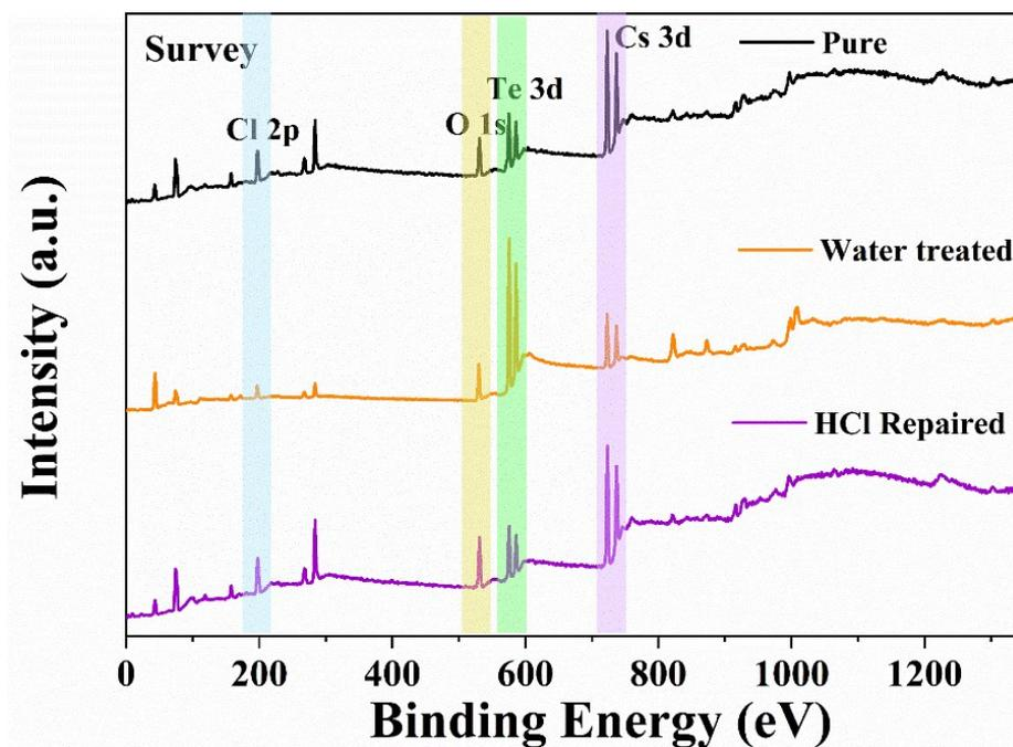
Figure S13. XPS survey scan spectra of  $\text{Cs}_2\text{TeCl}_6$  before and after HCl gas repairment.
