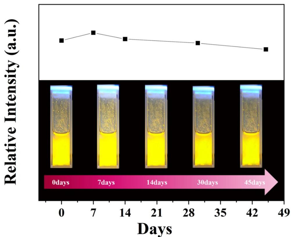
Figure S3. The luminescence intensity of the sample stored in the air under excitation at 365 nm, the inset is the physical luminescence of  $\text{Cs}_2\text{TeCl}_6$ .
