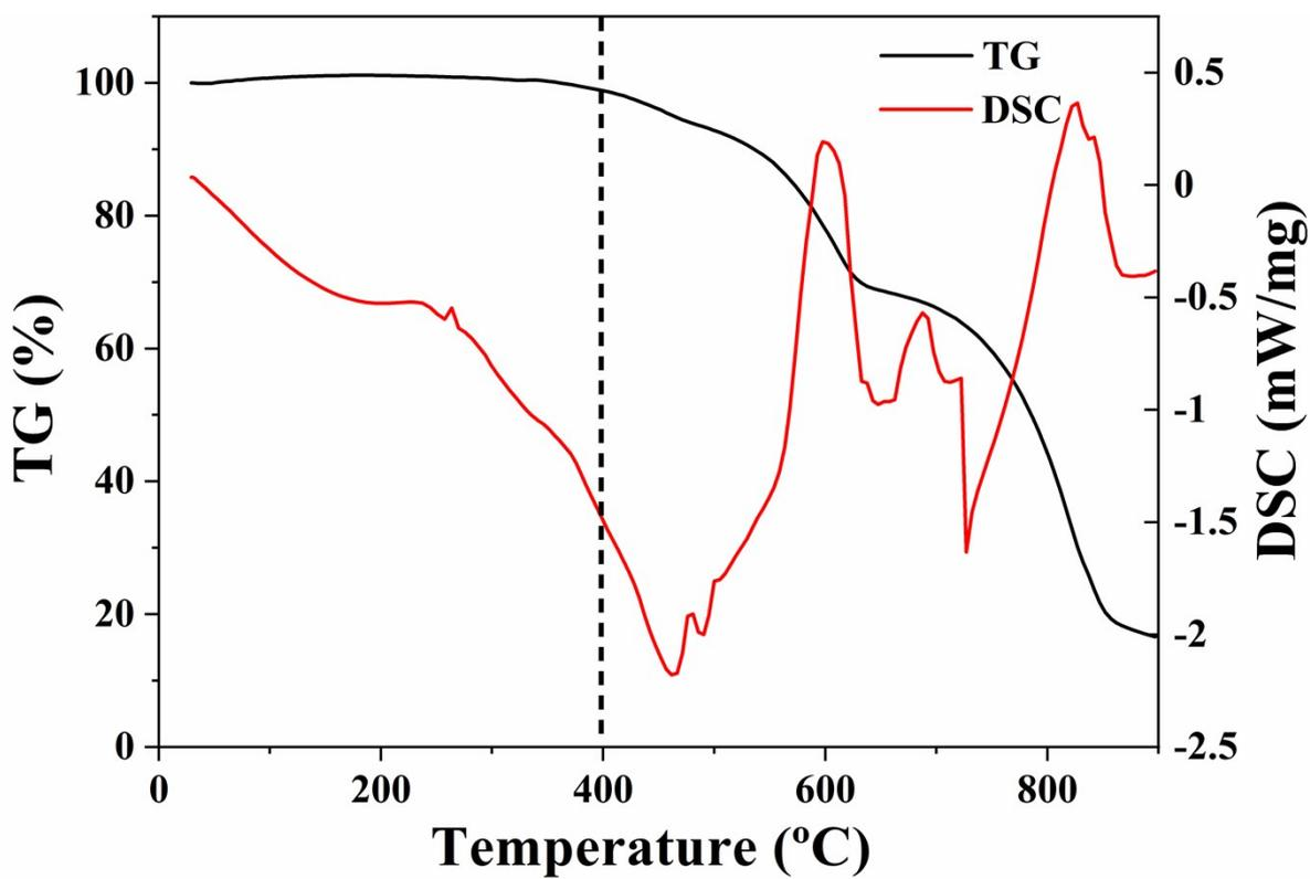
Figure S5. TG and DSC of  $\text{Cs}_2\text{TeCl}_6$ .
