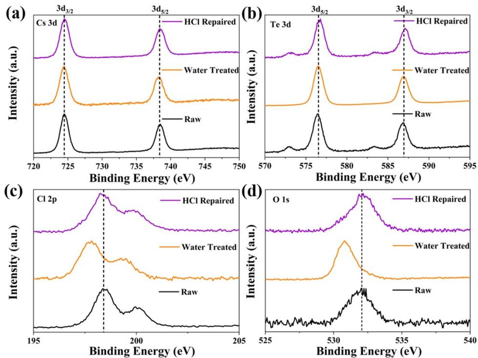
Figure S12. XPS spectra of (a) Cs 3d, (b) Te 3d, (c) Cl 2p, (d) O 1s for  $\text{Cs}_2\text{TeCl}_6$  before and after HCl gas repairment.
