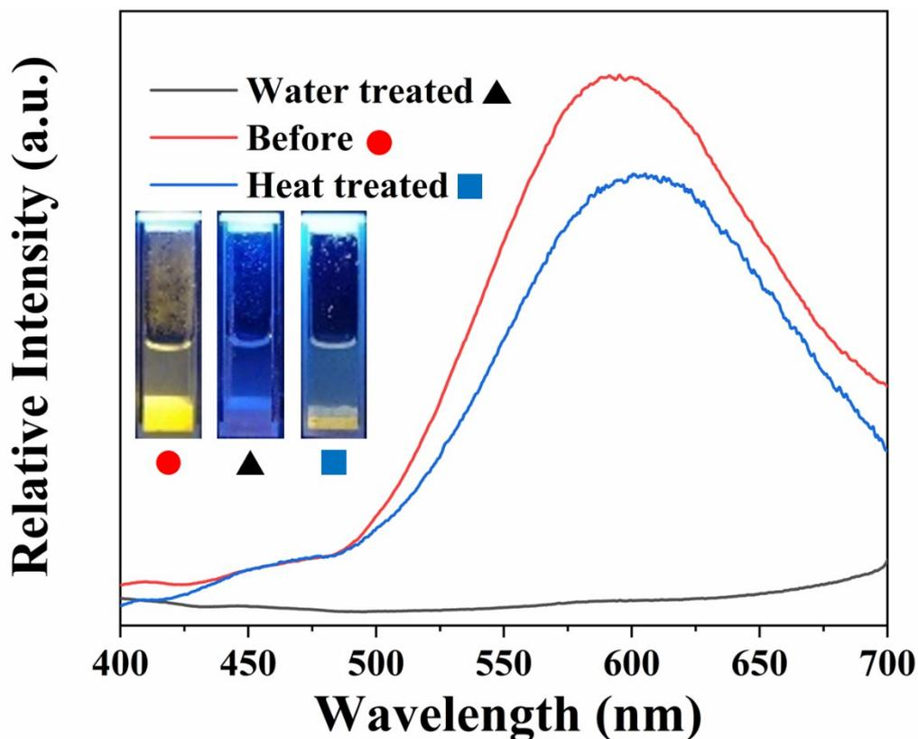
Figure S7. PL spectra of  $\text{Cs}_2\text{TeCl}_6$  before and after the thermal repair under 365nm excitation, insets are physical luminescence diagrams, where triangle, circle, and square represent water-treated, original, and heat-treated samples, respectively.
