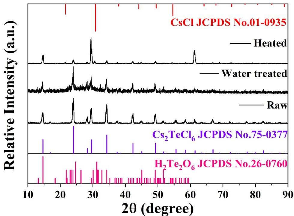
Figure S6. The XRD patterns of  $\text{Cs}_2\text{TeCl}_6$  before and after the thermal repair.
