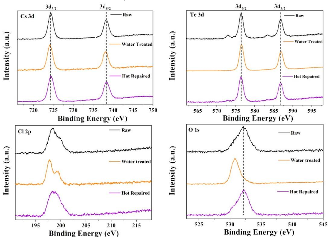
Figure S9. XPS spectra of (a) Cs 3d, (b) Te 3d, (c) Cl 2p, (d) O 1s for  $\text{Cs}_2\text{TeCl}_6$  before and after heat treatment.
