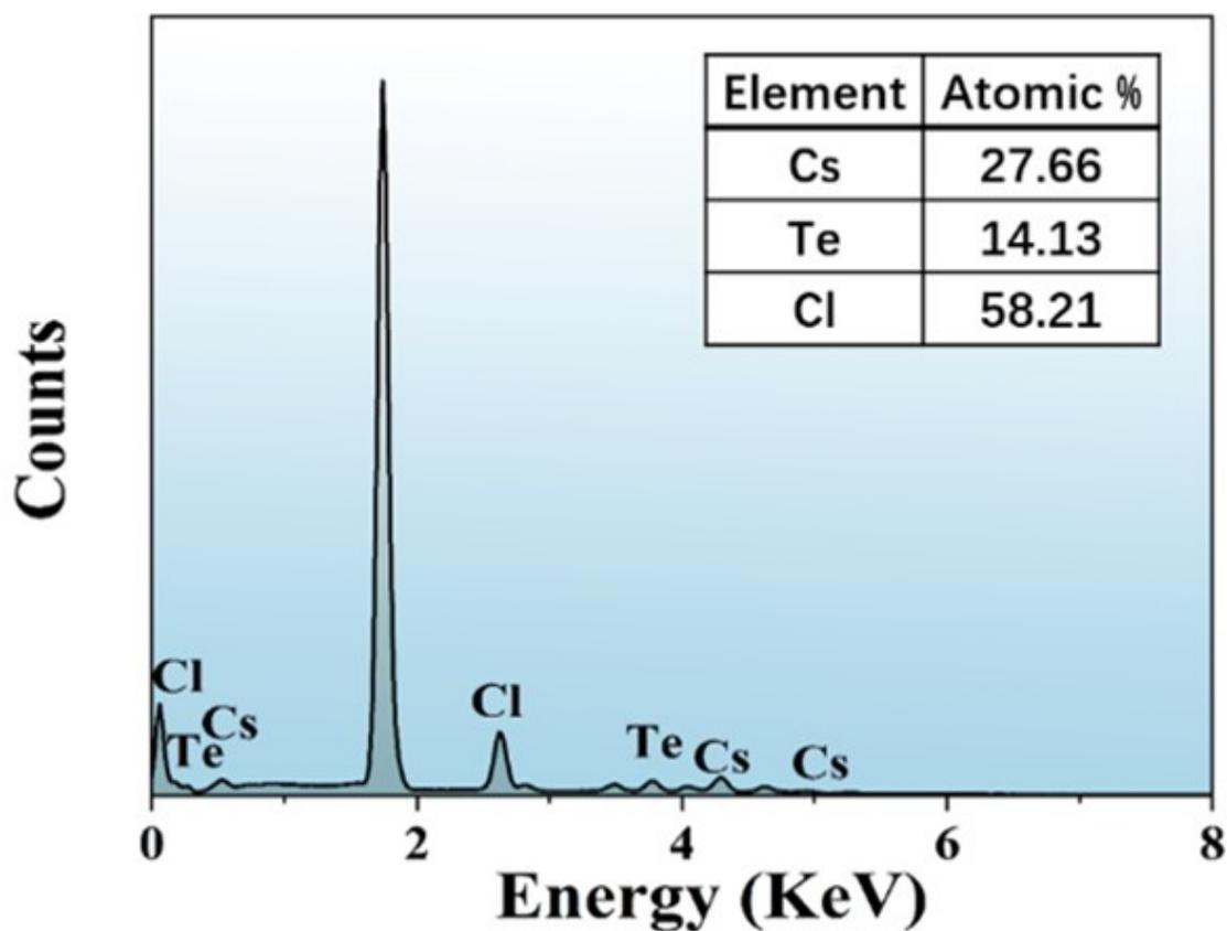
Figure S1. EDX spectroscopy of  $\text{Cs}_2\text{TeCl}_6$ , the inset is the average atomic ratio Cs/Te/Cl of 2:1:6 determined by EDS.
