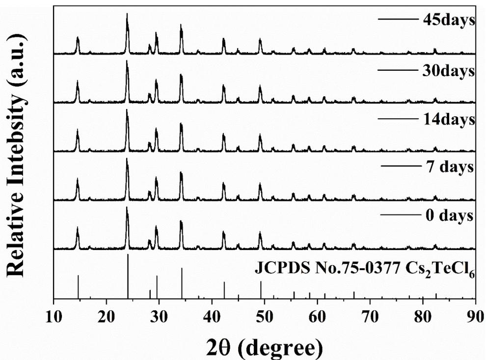
Figure S4. The XRD patterns of  $\text{Cs}_2\text{TeCl}_6$  stored in air for 45 days.
