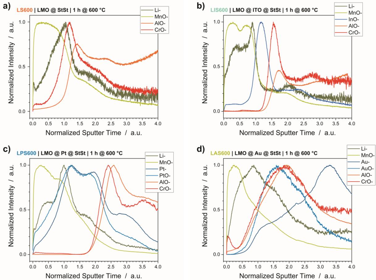
Fig. S4 ToF-SIMS depth profiles of 600 °C annealed a) LMO @ StSt, b) LMO @ ITO, c) LMO @ Pt and d) LMO @ Au. Sputter time is normalized to 1 for the interface between LMO and interlayer. LMO elements (Li<sup>-</sup> and MnO<sup>-</sup>) in green, StSt elements (AlO<sup>-</sup> and CrO<sup>-</sup>) in red and interlayer elements (InO<sup>-</sup>, Pt<sup>-</sup>, PtO<sup>-</sup>, Au<sup>-</sup> and AuO<sup>-</sup>) in blue.
