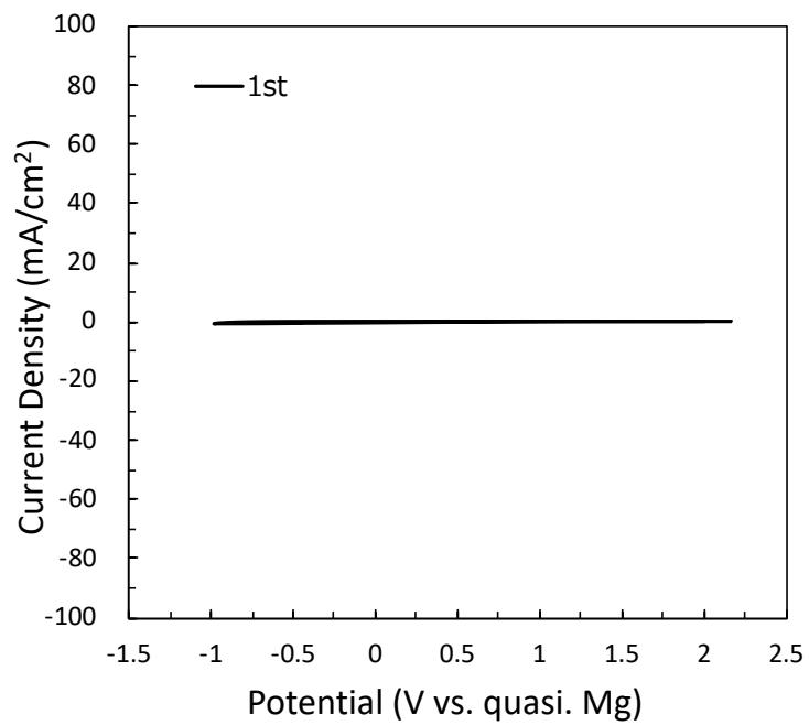
**Figure S4.** Cyclic voltammograms (1<sup>st</sup> cycle) of 0.5 M Mg<sup>2+</sup>[7–12-Br<sub>6</sub>-CCA]<sub>2</sub> in G3.
