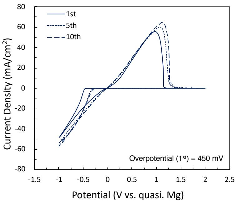
**Figure S2.** Cyclic voltammograms (1<sup>st</sup>, 5<sup>th</sup>, and 10<sup>th</sup> cycles) of 1.0 M Mg<sup>2+</sup>[12-Cl-CCA]<sub>2</sub> in DME.
