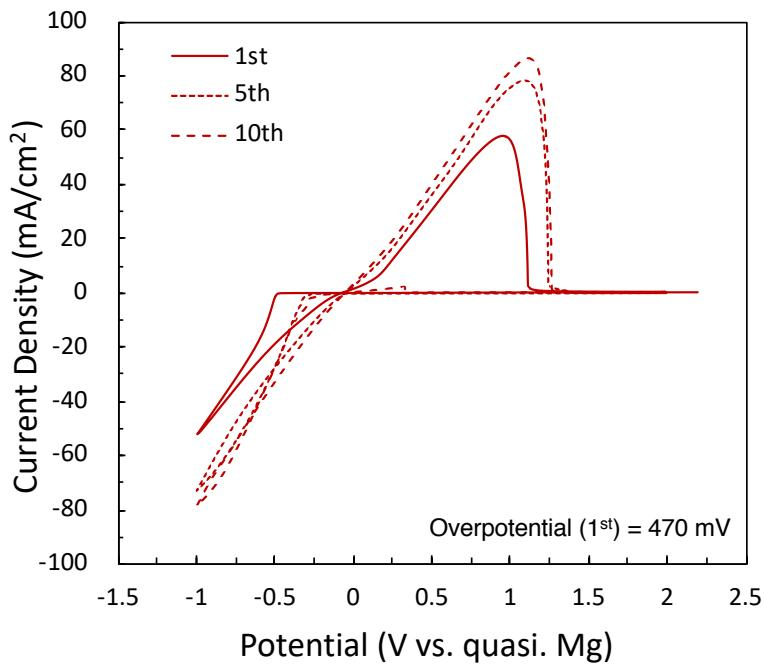
**Figure S3.** Cyclic voltammograms (1<sup>st</sup>, 5<sup>th</sup>, and 10<sup>th</sup> cycles) of 0.8 M Mg<sup>2+</sup>[12-Br-CCA]<sub>2</sub> in DME.
