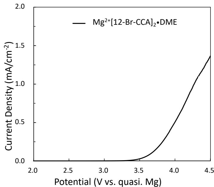
**Figure S6.** Linear sweep voltammogram of 0.3 M  $\text{Mg}^{2+}[12\text{-Br-CCA}]_2\bullet\text{DME}$  electrolyte on aluminium electrode at scan rate of 0.1 mV/s.
