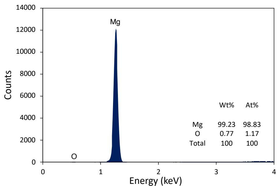
**Figure S5.** Energy dispersive X-ray spectroscopy (EDS) spectrum.
