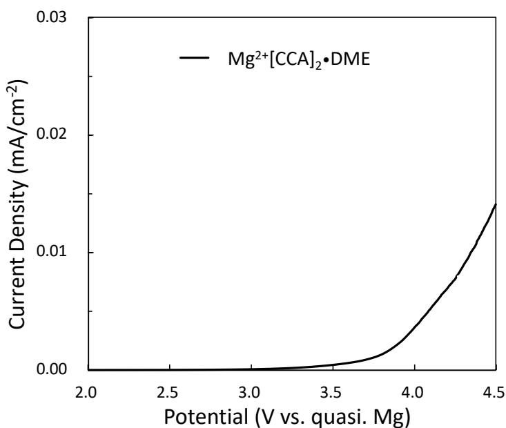
**Figure S7.** Linear sweep voltammogram of 0.3 M  $\text{Mg}^{2+}[\text{CCA}]_2\bullet\text{DME}$  electrolyte on aluminium electrode at scan rate of 0.1 mV/s.
