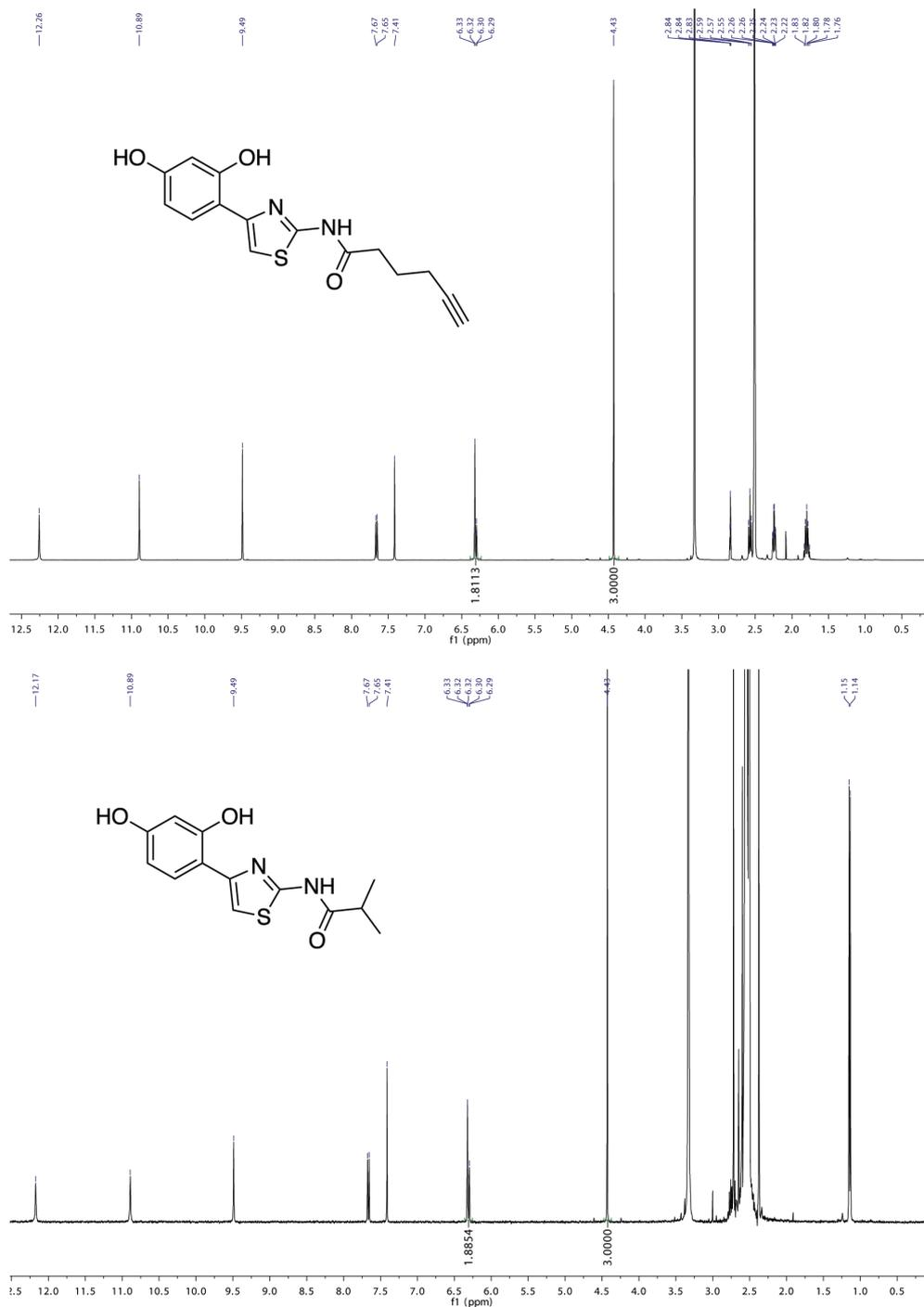
**Figure S4.** Concentration of Thiamidol<sup>TM</sup> and Thiamidol<sup>TM</sup>-alkyne was measured via NMR in presence of a known concentration of nitromethane (CH<sub>3</sub>NO<sub>2</sub>,  $\delta$  4.43, 3H).
