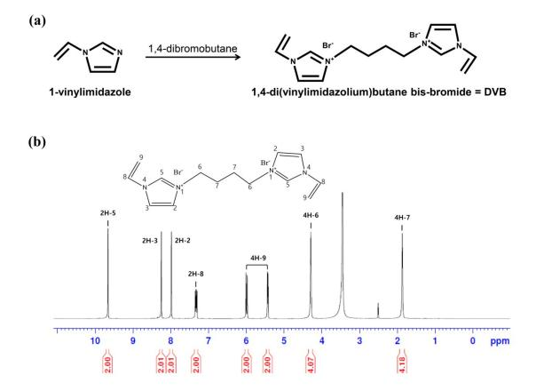
**Figure S1.** (a) Synthesis and (b) <sup>1</sup>H-NMR spectra of cationic crosslinker (1,4di(vinylimidazolium)butane dis-bromide; DVB).
