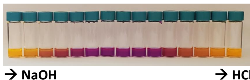
Figure S2. UV-vis spectra for 0.05 mg/mL PDIN-H solutions in n-propanol with molar equivalents of NaOH and HCl added sequentially. NaOH added PDIN-H followed by adding HCl to the formed PDIN- anion. This experiment shows that the deprotonation of PDIN-H is fully reversible. Pictures of the solutions shown.
