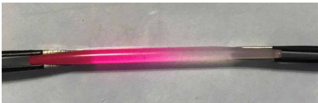
Figure. S17. Photograph of PNIPAm/PNAGA-4 healable hydrogel showing the ability to withstand stretching.
