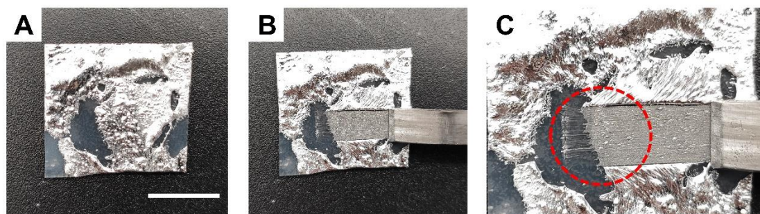
Figure S16. Scraping experiment to conductive nanoclay on silicone elastomer substrate. The scale bar is 1cm.
