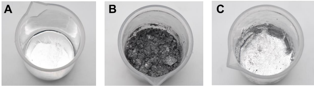
Figure S1. Three states in the stirring process of nanoclay and liquid metal: initial state(A), intermediate state(B) and final state(C).
