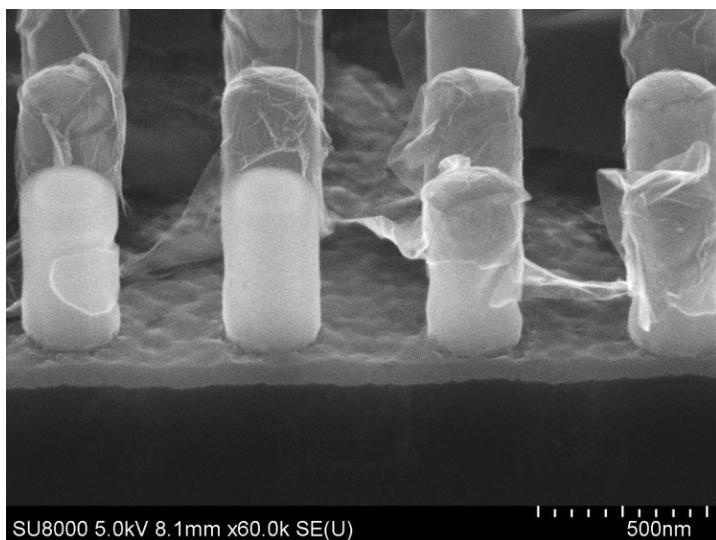
**Figure S6. 2 minute anneal.** SEM image of the sample annealed for 2 minutes, after etching nickel. The image is taken at the severed sample edge where the torn graphene layer is pulled off of some of the NWs. Similar to the anneal at 900 °C for 1.5 minutes, there is visible damage to the SiO<sub>2</sub> layer as now seen with the graphene layer removed. Despite the lower anneal temperature, the longer anneal at 875 °C still eventually resulted in destructive nickel dewetting behavior.
