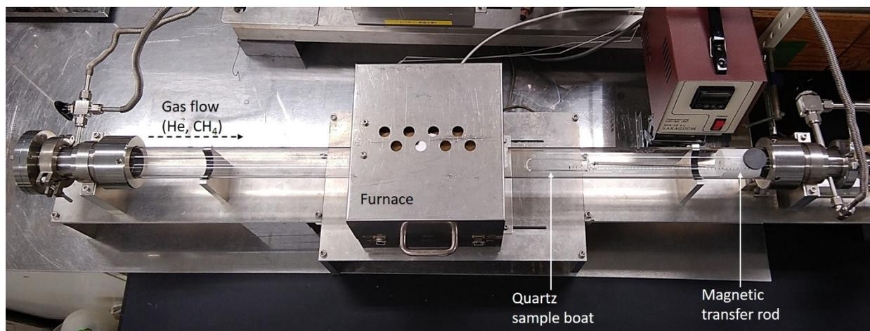
**Figure S1. Custom-made quartz tube furnace CVD system.** Picture of the multi-purpose furnace system that was used during the main portion of the described experiment where the samples were annealed at high temperature with a carbon source to form the graphene. The furnace reaches the target temperature of 875
