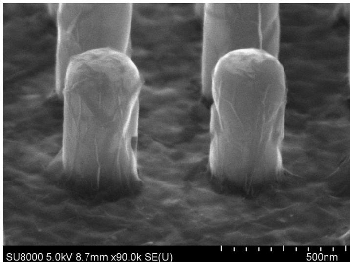
**Figure S4. 900 °C anneal.** SEM image of the sample annealed at 900 °C, after etching nickel. The sample experienced clear nickel dewetting behavior due to the high temperatures. Although a visible graphene sheet appears to be intact, the SiO<sub>2</sub> layer of most of the NWs are damaged through the removal of SiO<sub>2</sub> material and the formation of pores along the NW walls.
