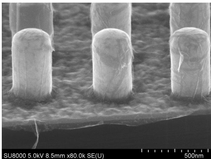
**Figure S9. 25 sccm CH<sub>4</sub> anneal.** SEM image of the sample annealed with 25 sccm CH<sub>4</sub>, after etching nickel. The results with the low CH<sub>4</sub> concentration are visually similar to the lower temperature and shorter anneal time, again pointing to a reduction in graphene growth.
