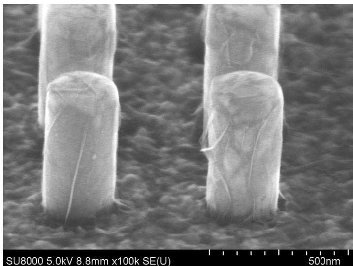
**Figure S7. 1 minute anneal.** SEM image of the sample annealed for 1 minute, after etching nickel. Similar to the results at 850 °C, there are thinly visible graphene films and a lack of visible damage. The shorter anneal time therefore also limits the extent of the graphene growth.
