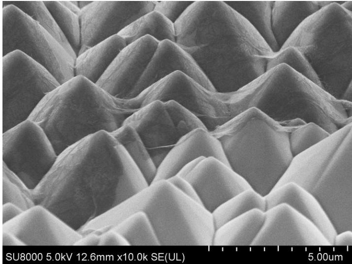
**Figure S12. Pyramid structure results.** SEM image of multilayer graphene partially remaining on nanopyramid array, after etching nickel. The pyramidal structure was able to create a graphene layer with a 3D shaped structure, but the silicon pyramids cannot anchor the graphene during etching. As a result, almost all the graphene was washed away and the image here represents only an extremely small section where some graphene remained as seen in the upper half of the image.
