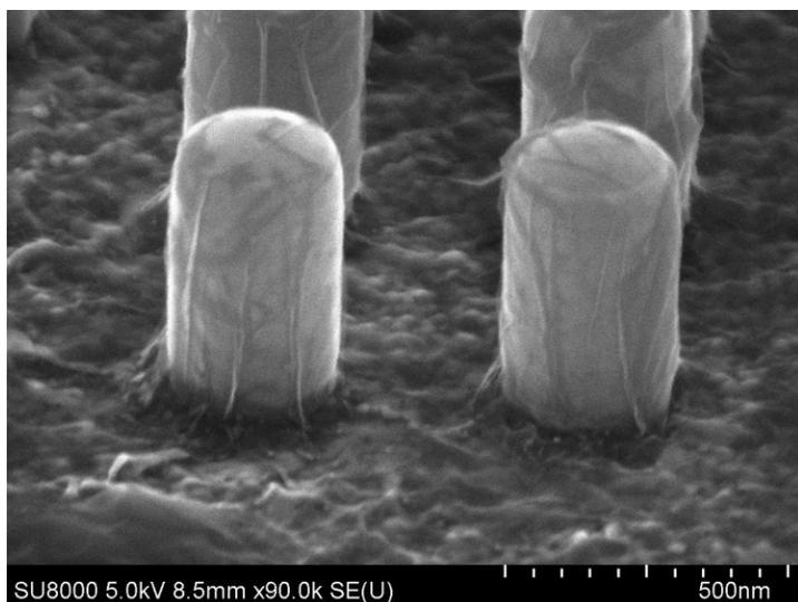
**Figure S5. 850 °C anneal.** SEM image of the sample annealed at 850 °C, after etching nickel. The sample is similar to the results at 875 °C except for an increase in contrast of spots on the NWs due to the different number of layers of graphene (either from folds or small graphene patches), and a less stiff appearance of the film. There is almost no visible damage to the SiO<sub>2</sub> layer of the NWs because of the lower temperature.
