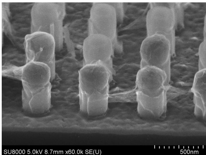
**Figure S10. 50 torr anneal.** SEM image of the sample annealed at 50 torr, after etching nickel. There is a large amount of visible damage to the NWs due to nickel dewetting at this lower pressure compared to the higher pressure experiments despite being performed at the same temperature and annealing time. The graphene growth is also very poor and segmented perhaps due to a reduction in the density of carbon precursors at low pressure.
