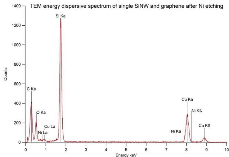
**Figure S2. Elemental analysis of graphene on a single NW.** EDS spectrum measured using TEM (on a TEM grid containing C and Cu) of single NW after nickel etching. The spectrum shows silicon, carbon, and oxygen as expected. Copper is also detected presumably from the TEM grid and is not seen in SEM-EDS results. Most important is the lack of clear nickel peaks. This shows that the etching process was effective enough to remove nickel to below detectable levels.
