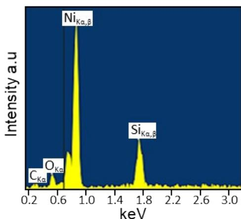
**Figure S3. Elemental analysis before Nickel etching.** EDS spectrum measured using SEM of multiple nanowires before nickel etching. Nickel is clearly the dominant signal before etching, illustrating the extent that it is reduced when compared to Figure 5 (c) and Figure S2
