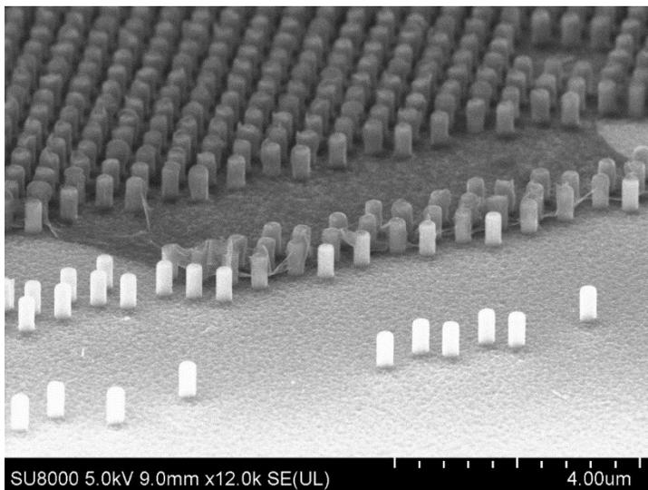
**Figure S13. NW and planar section boundary.** SEM image demonstrating the limits of multilayer graphene anchoring by NWs. Graphene on the clustered together NWs stay on-site after wet etching, while graphene on the planar areas is ripped and washed away. Isolated NWs on the bottom portion of the image cannot retain the graphene layer either. But, small enough planar sections between clusters of NWs can be kept in place such as is the middle of the image.
