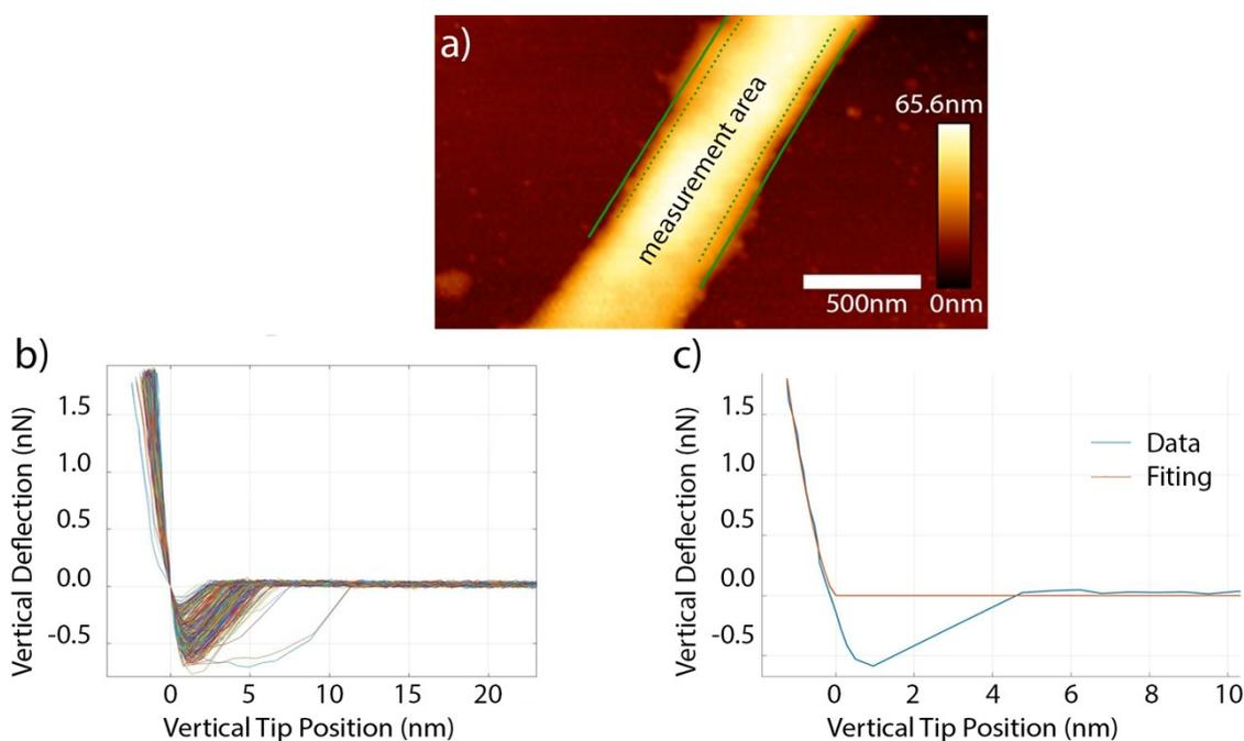
Supplementary Figure S1. a) representative polymer line measured by AFM. b) overlay of 400 force-distance curves measured on the polymer line. d) zoom of one representative force-distance curve (blue) and applied Hertz fit (orange) to retrieve the value of the Young's modulus.
