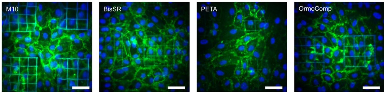
*Supplementary Figure S3. Immunofluorescent staining of HUVEC grown on four different polymer grids. From left to right: M10, BisSR, PETA, and OrmoComp. HUVEC were stained with CD31 Ab (green), and a DAPI nuclear stain (blue). The scale bar is 50 $\mu$ m.*
