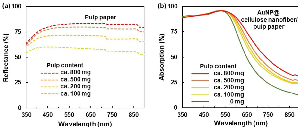
**Fig. S5** (a) UV-vis-NIR reflectance spectra of pulp paper with different pulp contents (pulp content: ca. 100, 200, 500 and 800 mg, thickness: ca. 80, 130, 300 and 410  $\mu\text{m}$ , respectively), and (b) absorption spectra of AuNP@cellulose nanofiber/pulp paper with different pulp contents (pulp content: 0, ca. 100, 200, 500 and 800 mg, thickness: ca. 100, 160, 210, 360 and 520  $\mu\text{m}$ , respectively).
