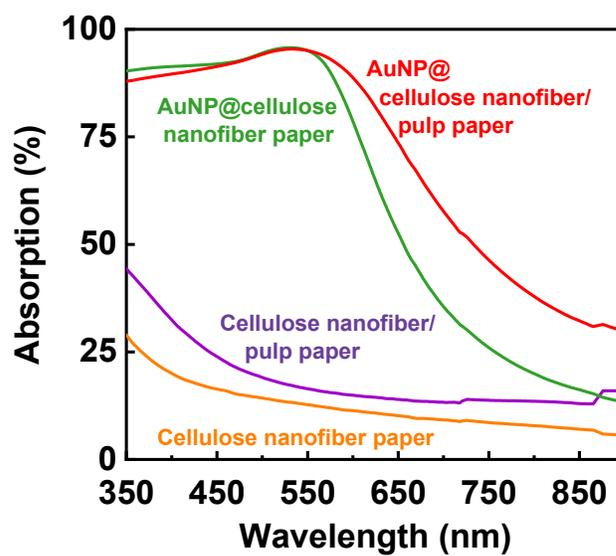
**Fig. S4** UV-vis-NIR absorption spectra of AuNP@cellulose nanofiber paper (thickness: ca. 100  $\mu\text{m}$ , AuNP content: 3.3  $\text{mmol m}^{-2}$ ), AuNP@cellulose nanofiber/pulp paper (thickness: ca. 520  $\mu\text{m}$ , AuNP content: 3.3  $\text{mmol m}^{-2}$ , pulp content: ca. 800 mg), cellulose nanofiber paper, and cellulose nanofiber/pulp paper (pulp content: ca. 800 mg).
