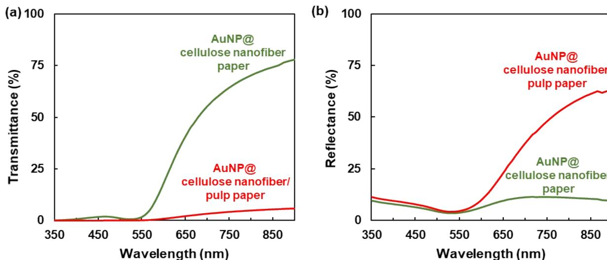
**Fig. S3** UV-vis-NIR (a) transmittance spectra and (b) reflectance spectra of AuNP@cellulose nanofiber paper (thickness: ca. 100  $\mu\text{m}$ , AuNP content: 3.3  $\text{mmol m}^{-2}$ ) and AuNP@cellulose nanofiber/pulp paper (thickness: ca. 520  $\mu\text{m}$ , AuNP content: 3.3  $\text{mmol m}^{-2}$ , pulp content: ca. 800 mg).
