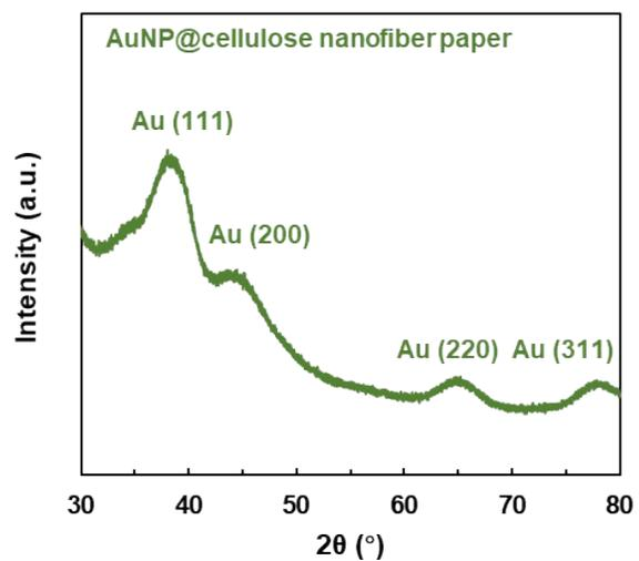
**Fig. S1** X-ray diffraction pattern of the AuNP@cellulose nanofiber paper. The characteristic peaks of the Au crystal<sup>1</sup> at 38.2°, 44.5°, 64.7° and 77.7° are confirmed, which indicate the formation of AuNP within the cellulose nanofiber paper.
