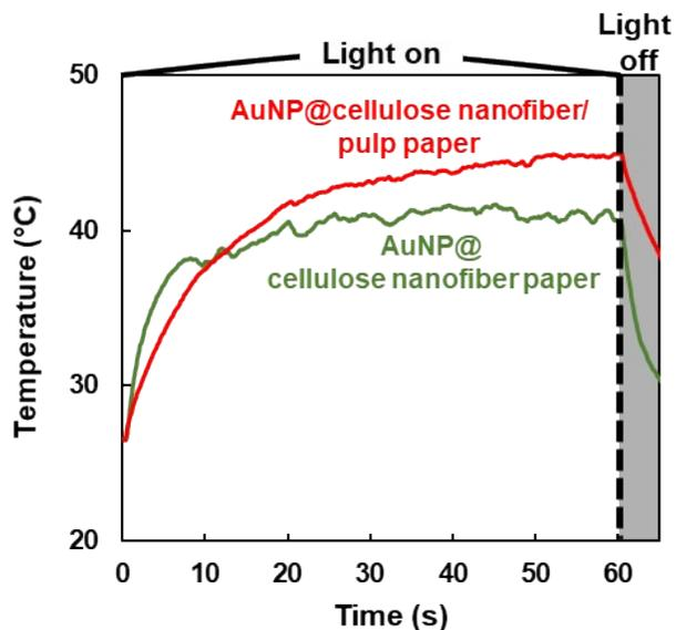
**Fig. S6** Surface temperature of AuNP@cellulose nanofiber paper (thickness: ca. 100  $\mu\text{m}$ , AuNP content: 3.3  $\text{mmol m}^{-2}$ ) and AuNP@cellulose nanofiber/pulp paper (thickness: ca. 520  $\mu\text{m}$ , AuNP content: 3.3  $\text{mmol m}^{-2}$ , pulp content: ca. 800 mg) over time during surface temperature measurement under 1.0  $\text{kW m}^{-2}$  irradiation.
