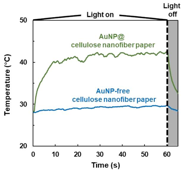
**Fig. S2** Surface temperature of cellulose nanofiber paper and AuNP@cellulose nanofiber paper (AuNP content:  $3.3 \text{ mmol m}^{-2}$ ) over time during surface temperature measurement under  $1.0 \text{ kW m}^{-2}$  irradiation.
