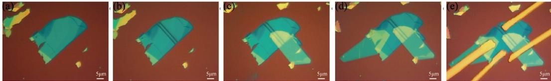
**Figure S2.** The optical microscope images of the fabrication procedure for the BP/MoS<sub>2</sub>/BP SBJT. (a) The pristine BP flake. (b) The BP flake after FSLP. (c) Transfer MoS<sub>2</sub> flake. (d) Transfer hBN flake. (e) Deposit Au metal electrodes.
