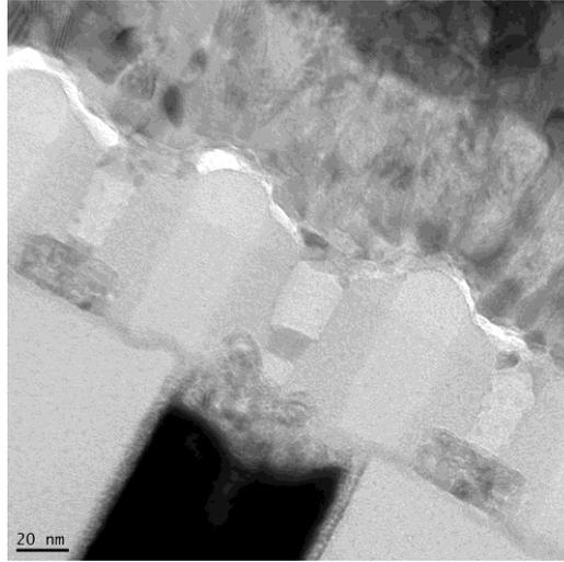
**Figure S1.** TEM image showing a TEM sample failed during SEM nano-probing test due to the volatilization of GST.
