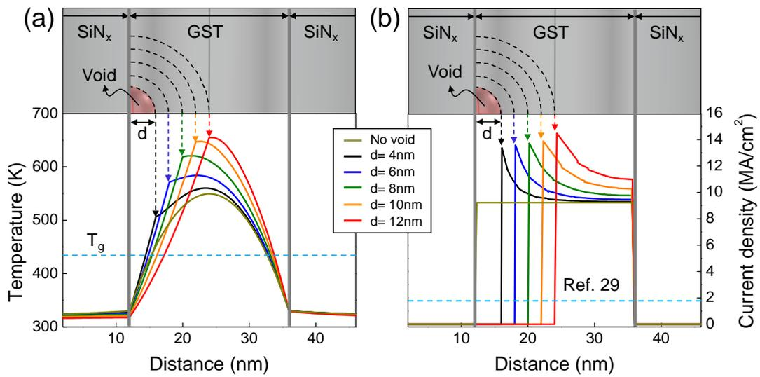
**Figure S2.** Finite element modeling of temperature distribution and current density. (a) Temperature profiles and (b) current density profiles across the confined GST nanopillar with different size of void. The glass transition temperature ( $T_g$ ) and the critical current density for initiating the electromigration of GST elements is indicated by a blue dotted line (Ref. 29).
