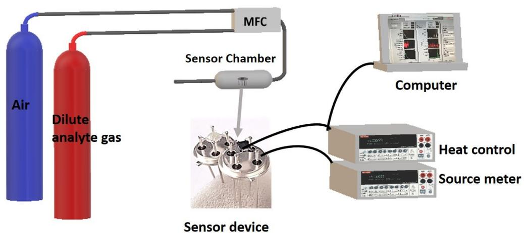
Fig. S6 Schematic illustration of the set up for the gas sensing measurements.
