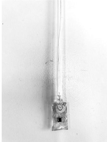
Fig. S7 Photograph of the electrode for Mott-Schottky measurement.
