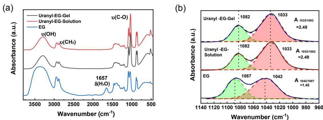
Fig. S2 FT-IR spectroscopy of uranyl-ethylene-gel and uranyl-ethylene-solution.
