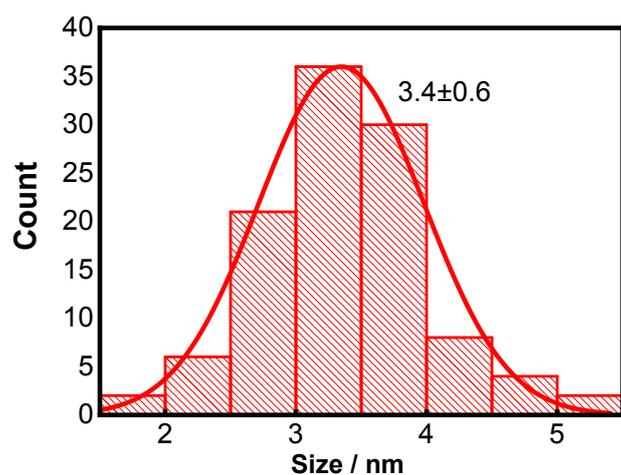
Fig. S4 Figure. Size distribution of the UO<sub>2</sub> nanoparticles from TEM images.
