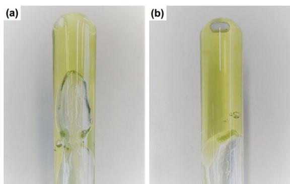
Fig. S1 Thixotropy properties of uranyl EG gel (a) the gel after shaken and (b) the gel recovery from solution state in minutes.
