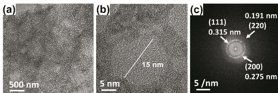
Fig. S5 TEM image of uranyl gel skeleton after photoreaction.
