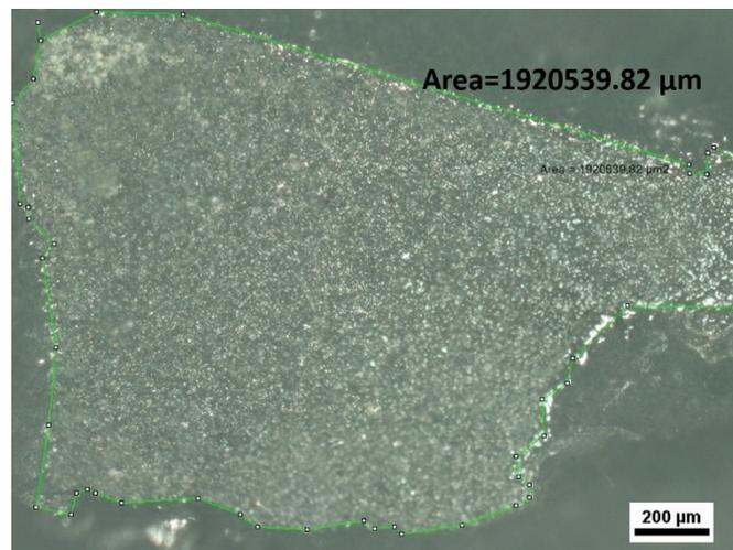
Fig. S8 Optical graph for area calibration of the electrode for Mott-Schottky measurement.
