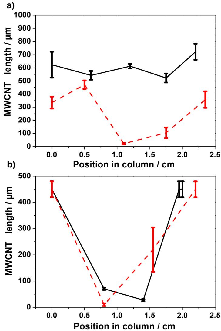
**Fig. S13.** Length profiles of VA-MWCNTs inside 2 cm long columns with (a) 2 mm ID and (b) 1 mm ID as a function of the position in the column for 2 cm long columns. The carrier gas flow was 5000 sccm and column-substrates were placed 39 (black, plain) and 45 cm (red, dashed) within the reactor. The precursor injection time was 90 minutes.
