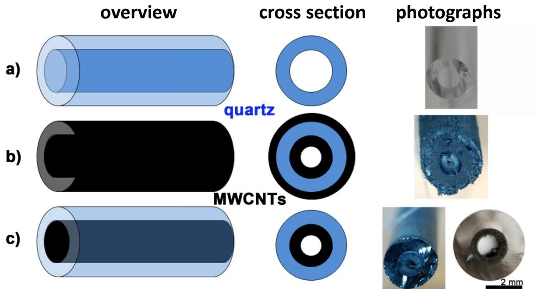
**Fig. S4.** Schematic representations and related photographs of quartz columns (blue), (a) before synthesis, (b) after VA-MWCNT (black) deposition, and (c) after removing the VA-MWCNTs grown on the outside surface of the columns. All columns in pictures are 2 mm inner diameter and 4 mm outer diameter.
