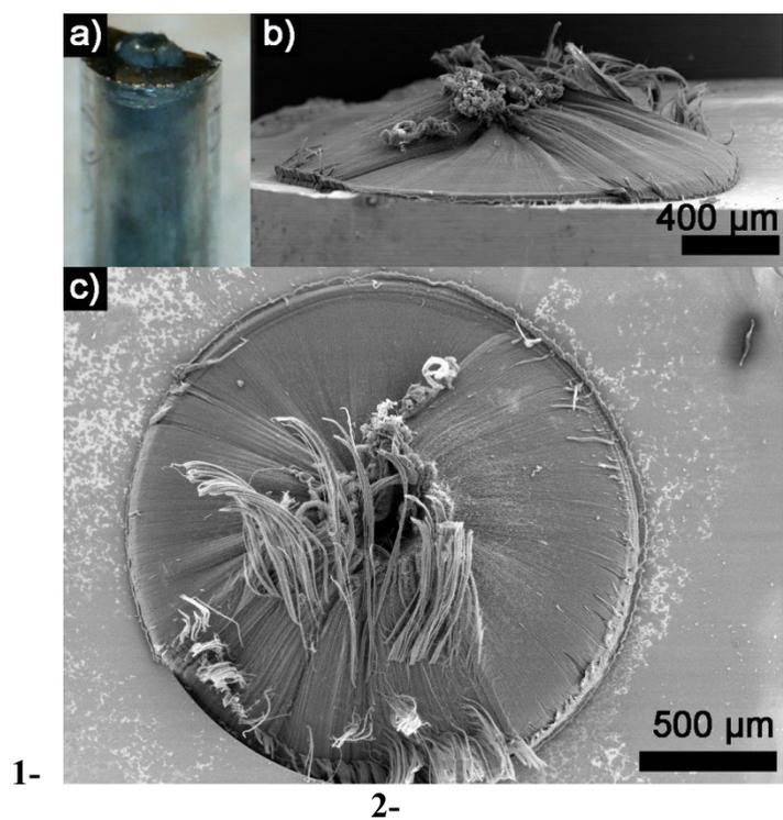
**Fig. S9.** (a) Pictures of VA-MWCNTs protruding at the exit (OUT position) of a CNC with a 2 mm ID and 4 mm outer diameter. (b) and (c) SEM micrographs close-ups of the cross section shown in (a) revealing protruding VA-MWCNTs blocking the core of the column.
