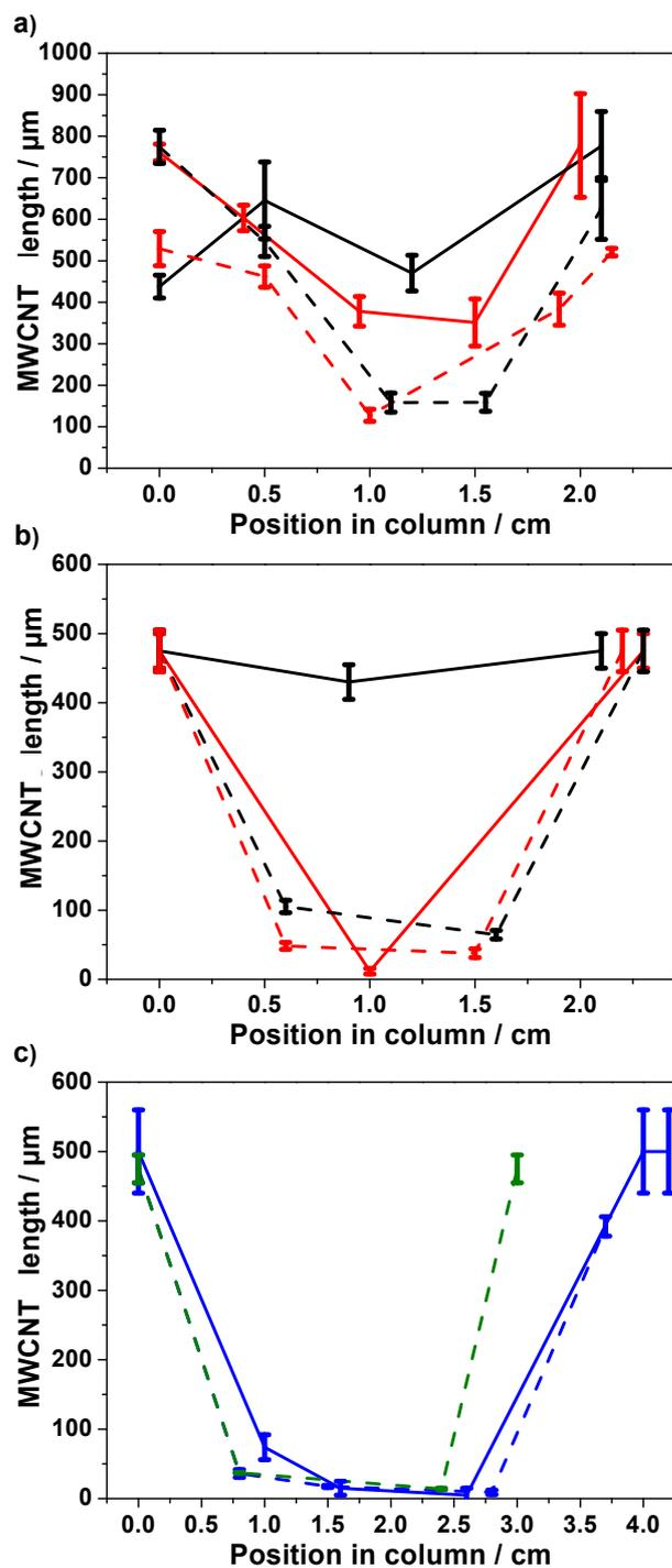
**Fig. S12.** Length profiles of VA-MWCNTs inside (a) 2 and (b) 1 mm ID columns as a function of the position in the column. The carrier gas flow rate was 1000 sccm (dashed) or 2500 sccm (plain). The column-substrates were placed 23 (black), 27 (green and blue) and 29 cm (red) within the furnace. Experiments were performed with precursor injection times of (a and b) 150 minutes or (c) 90 minutes.
