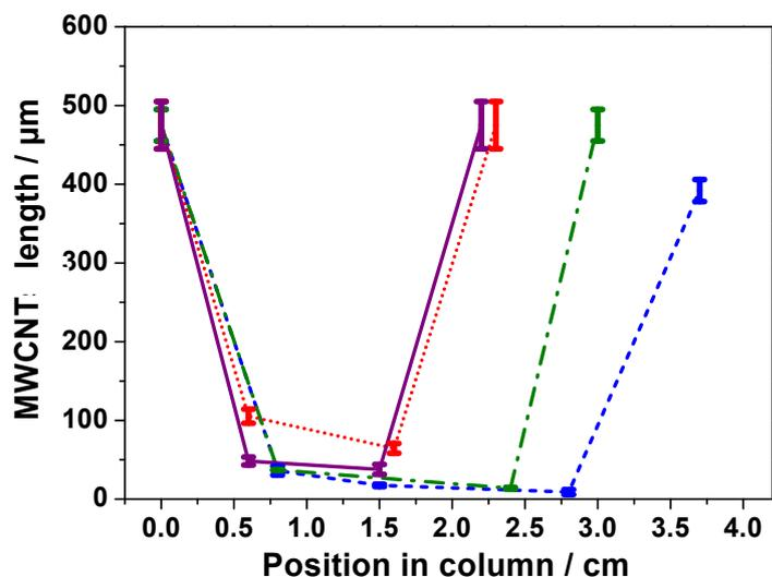
**Fig. S10.** Length profiles of VA-MWCNTs inside 2, 3 and 4 cm long 1mm ID columns as a function of the position in the column. The carrier gas flow rate was 1000 sccm and the precursor injected for 150 minutes for 2 cm long columns and 90 minutes for 3 and 4 cm long columns. All column-substrates were placed between 23 and 29 cm within the furnace.
