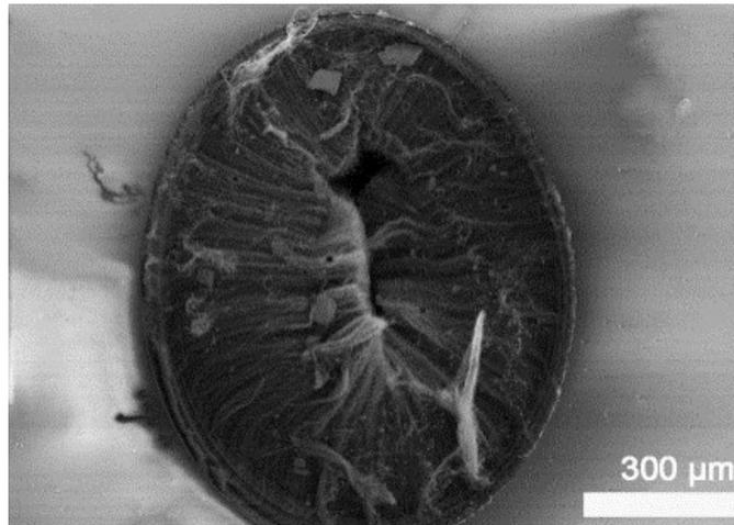
**Fig. S8.** Scanning electron microscope (SEM) micrograph of a completely blocked 1 mm ID column. It is observed that the as-received 1 mm ID columns do not exhibit a perfectly circular cross section.
