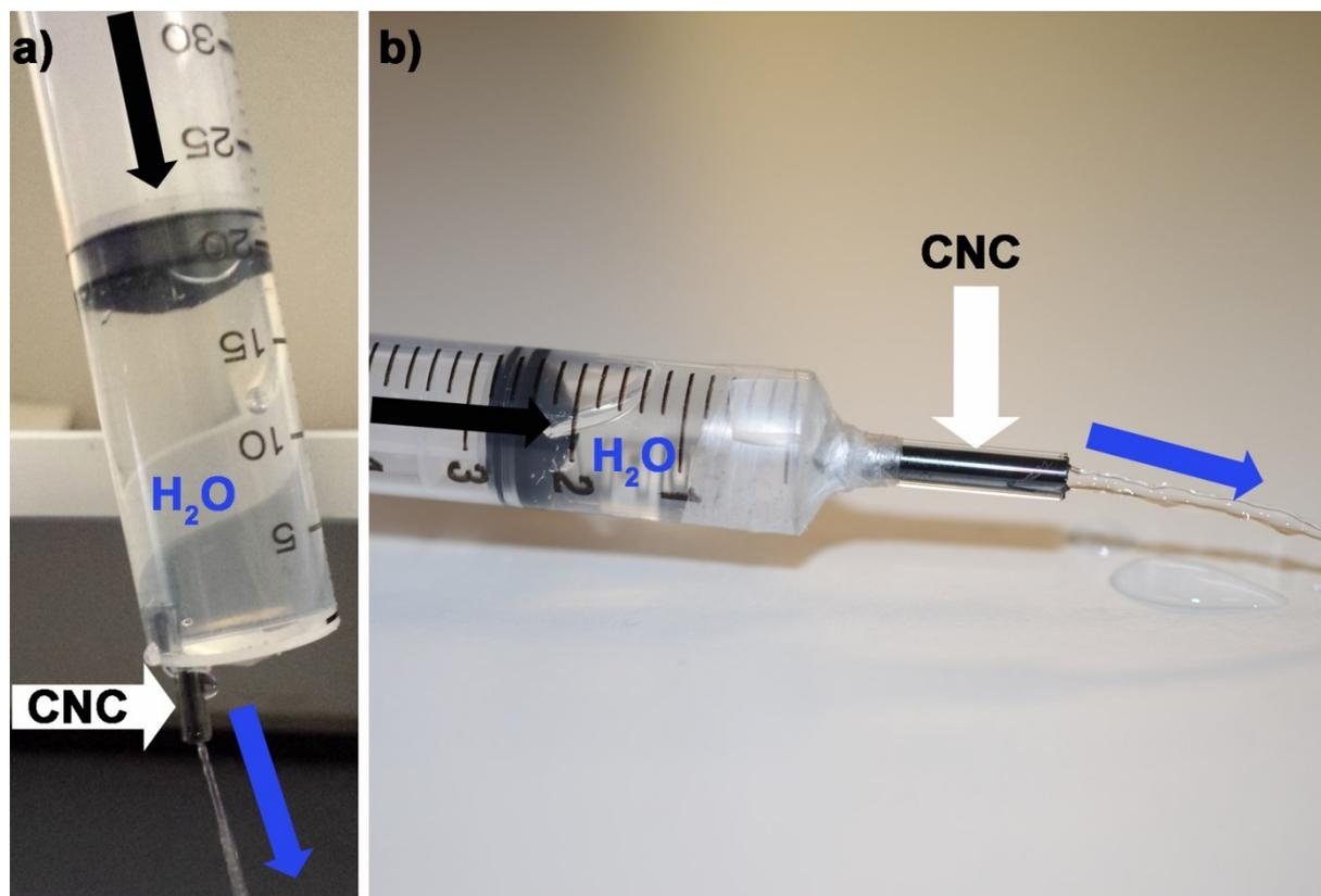
**Fig. S3.** (a,b) Pictures of a stream of water (highlighted with blue arrows) passing through a CNC. The applied pressure is indicated by a black arrow on the syringe connected to a CNC used as needle (2 mm ID, 2 cm long). Water is passing through the CNC without noticeable loss of the VA-MWCNTs from the CNC.
