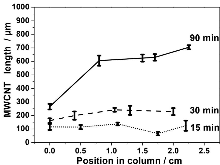
**Fig. S6.** Length profiles of VA-MWCNTs grown inside 2 cm long columns as a function of the position in the column and as a function of injection time of the hydrocarbon precursor during synthesis. Results were obtained for columns placed 23 cm within the furnace.
