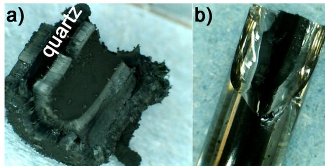
**Fig. S5.** (a) Optical image of a cross section along a 2 mm ID column axis (longitudinal section) before removing the outer deposits. The picture shows VA-MWCNTs grown on the internal and external quartz surfaces of the column. (b) Optical image of a CNC after removal of the VA-MWCNTs grown on the outer surface of the CNC, the photograph shows the growth of VA-MWCNT forests inside the column.
