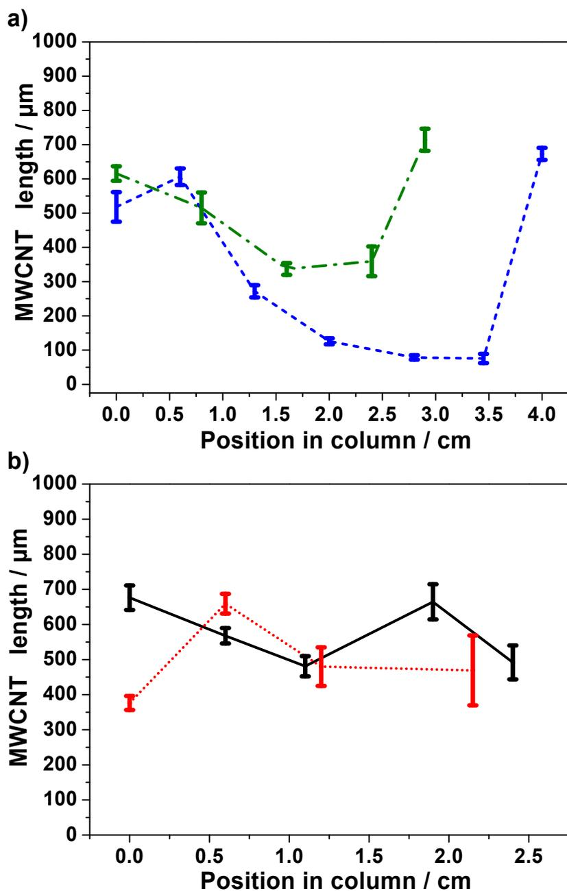
**Fig. S14.** Length profiles of VA-MWCNTs inside 2 mm ID columns as a function of the position in the column. A change of the carrier gas flow rate was performed during synthesis and the precursor injection time was (a) 15 minutes at 2500 sccm and then 75 minutes at 1000 sccm. Samples were placed at 27 (blue and green) cm into the furnace. The reproducibility of the results displayed in Fig. 5a is reported here in (b) where samples were placed 23 cm (red) or 29 cm (red) into the furnace.
