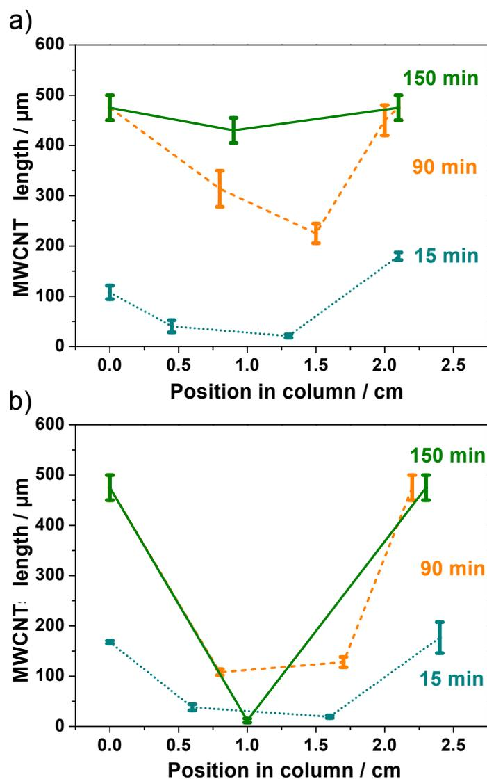
**Fig. S7.** Length profiles of VA-MWCNTs grown inside a 2 cm long 1 mm ID column as a function of the position in the column and as a function of the duration of the precursor injection. The carrier gas flow rate was 2500 sccm and the column placed (a) 23 cm and (b) 29 cm into the furnace.
