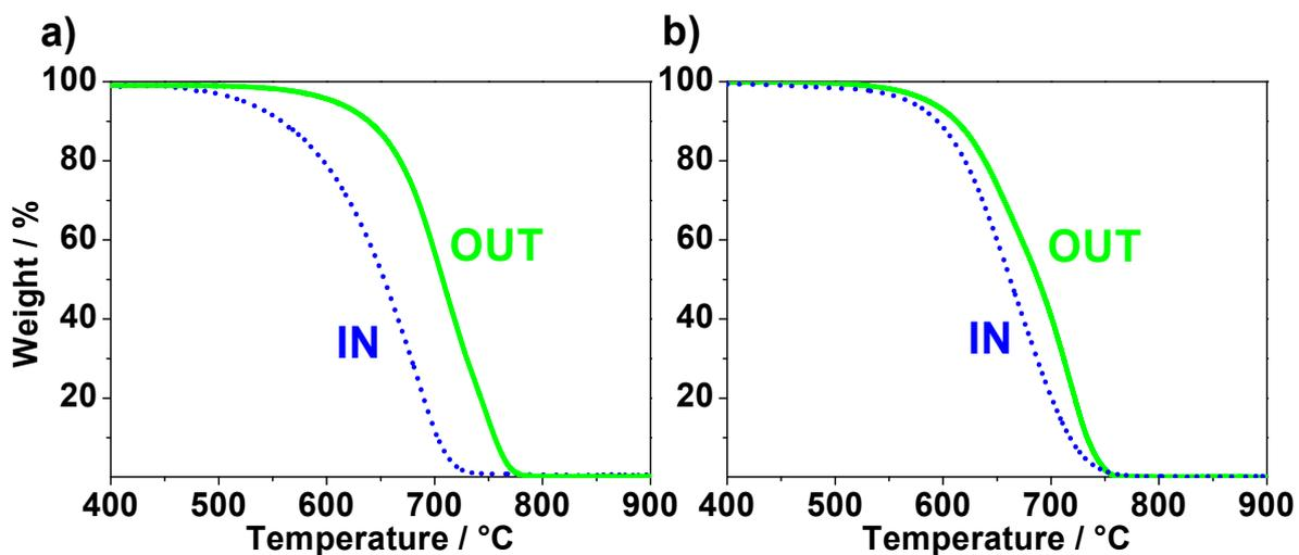
**Fig. S17.** Thermogravimetric analysis of MWCNTs collected at the IN and OUT positions of two 2 mm ID CNCs. A carrier gas flow rate of 2500 sccm was used for the synthesis of both CNS. The precursor injection time was (a) 90 minutes and (b) 150 minutes.
