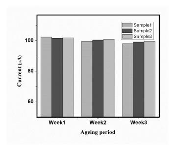
SI.1: Repeatability and Reproducibility of the sample carried out with three different electrodes prepared with the same sample denoted as sample 1, 2 and 3. The electrode was aged for three weeks and every week the analysis is carried out in all three samples
