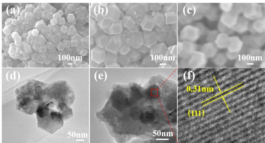
**Fig. S1.** (a, b) FESEM images of Si@ZIF-8; (c) FESEM images of Si@NC; (d, e, f) The HRTEM images corresponding to Si@ NC.
