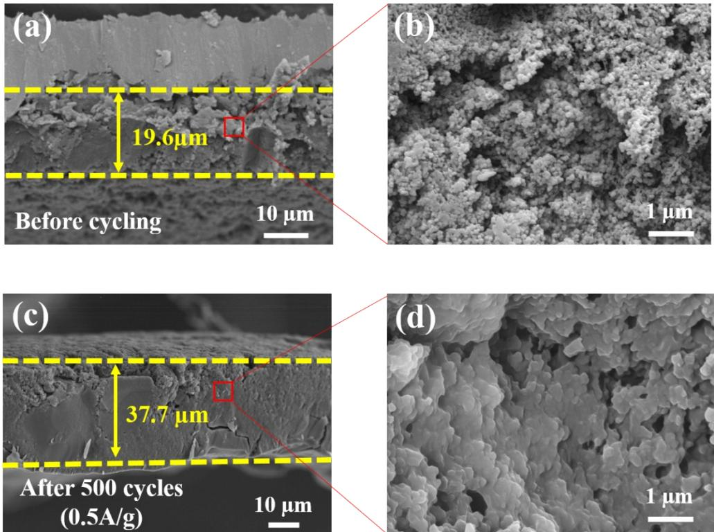
**Fig. S9.** (a) Cross-sectional SEM images of Si@NC; (b) Partial enlargement of active materials Si@NC electrode before cycling; (c) Cross-sectional SEM images of Si@NC electrode after 500 cycles at a current density of 0.5 A g<sup>-1</sup>; (d) Partial enlargement of active materials Si@NC after 500 cycles.
