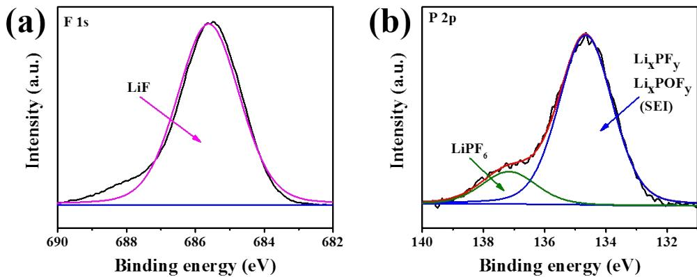
**Fig. S11.** XPS spectrum (a) F 1s, (b) P 2p of Si@H-NC@GC composite electrode after 400 cycles in LiPF<sub>6</sub>.
