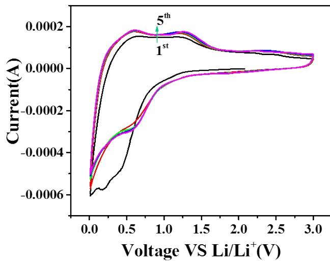
**Fig. S6.** CV curves for Si@NC at a scan rate of  $0.5\text{mV s}^{-1}$  in the potential window of  $0.01\sim 3.0\text{V}$  vs  $\text{Li}/\text{Li}^+$ .
