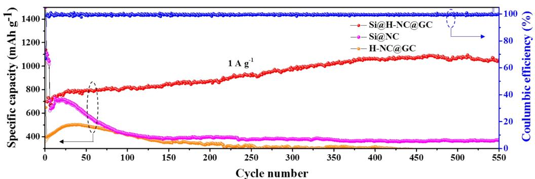
**Fig. S8.** Comparison of cycling performance of three electrodes at a current density of  $1.0\text{ A g}^{-1}$ .
