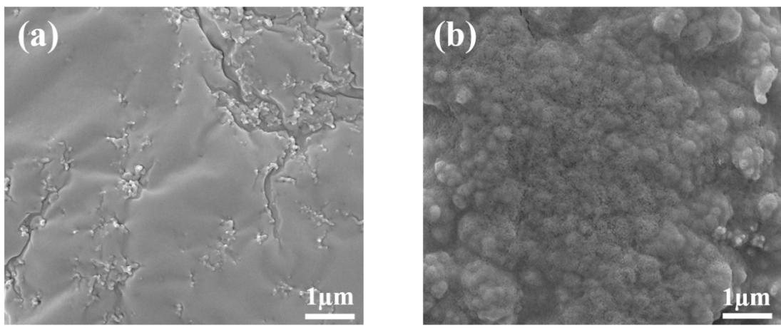
**Fig. S10.** (a) The electrode surface SEM images of Si@NC after 500 cycles at 0.5 A g<sup>-1</sup> current density; (b) The electrode surface SEM images of Si@H-NC@GC after 500 cycles at 0.5 A g<sup>-1</sup> current density.
