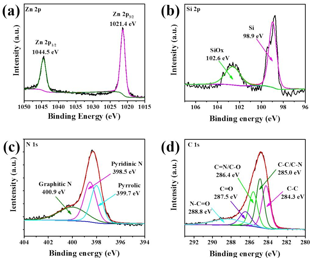
**Fig. S5.** XPS spectra of Zn 2p, Si 2p , N 1s, C 1s of the Si@NC sample. (a) Zn 2p has two peaks corresponding to metal Zn and ZnO at 1044.5 and 1021.4eV, respectively; (b) Silicon 2p has two peaks corresponding to silicon oxide and silicon at 102.6 and 98.9eV, respectively; (c) The N 1s peaks show the presence of pyridine N, pyrrole N and Graphitic N; (d) C1s peaks show N-doped carbon and carbon layers coating.
