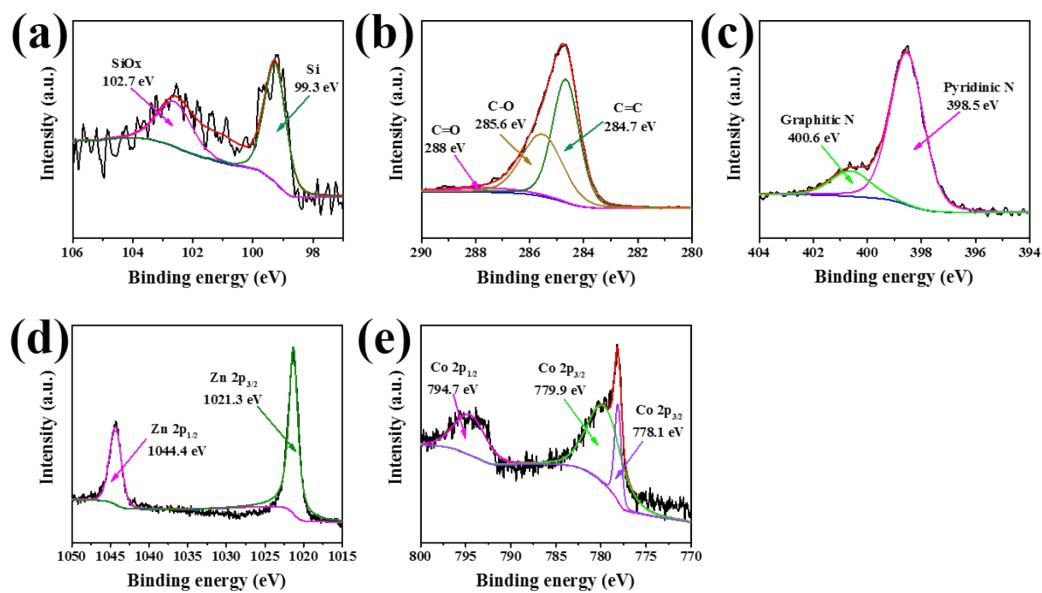
**Fig. S4.** XPS spectra of (a) Si 2p, (b) C 1s, (c) N 1s, (d) Zn 2p, (e) Co 2p of the Si@H-NC@GC sample.
