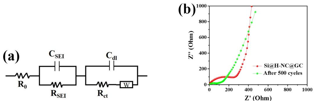
**Fig. S7.** (a) The corresponding equivalent circuit diagram of Si@H-NC@GC material EIS test; (b) Nyquist plots of Si@H-NC@GC composites before and after cycling.
