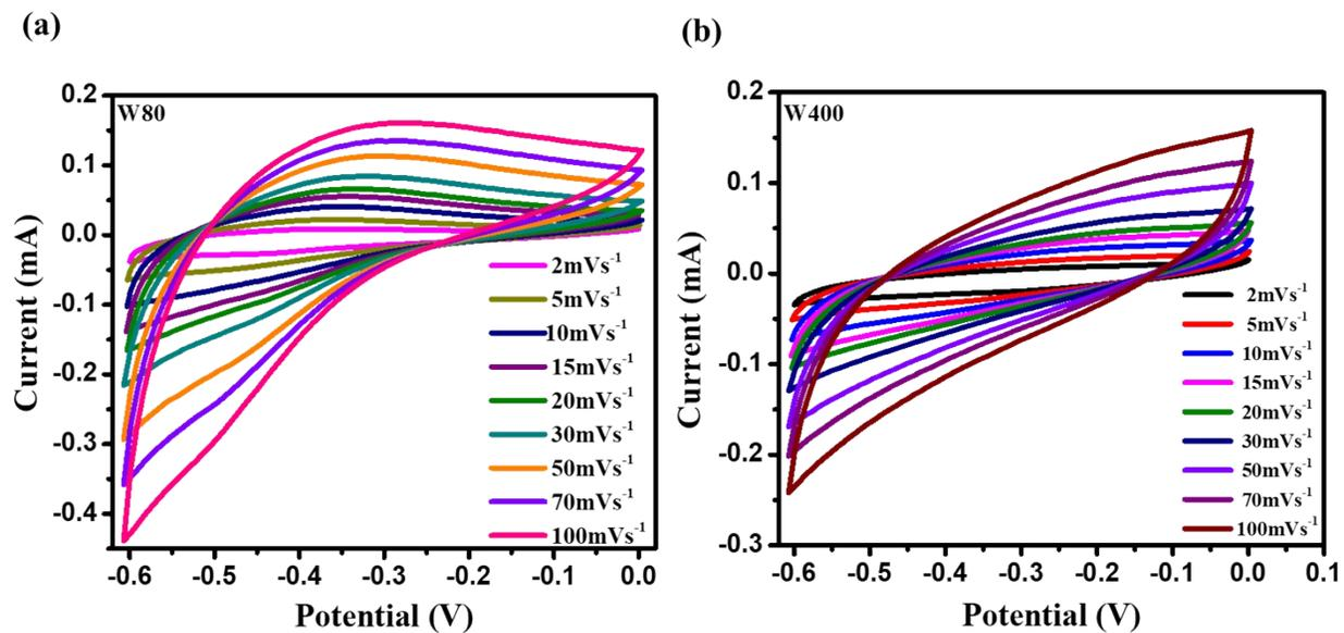
**Fig. S3.** Cyclic voltammetry curves of (a) W80, (b) W400 at various scan rates.
