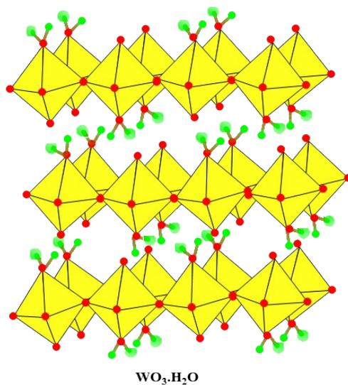
**Fig. S1.** Crystal structure of 2D layered  $\text{WO}_3 \cdot \text{H}_2\text{O}$  (W80).
