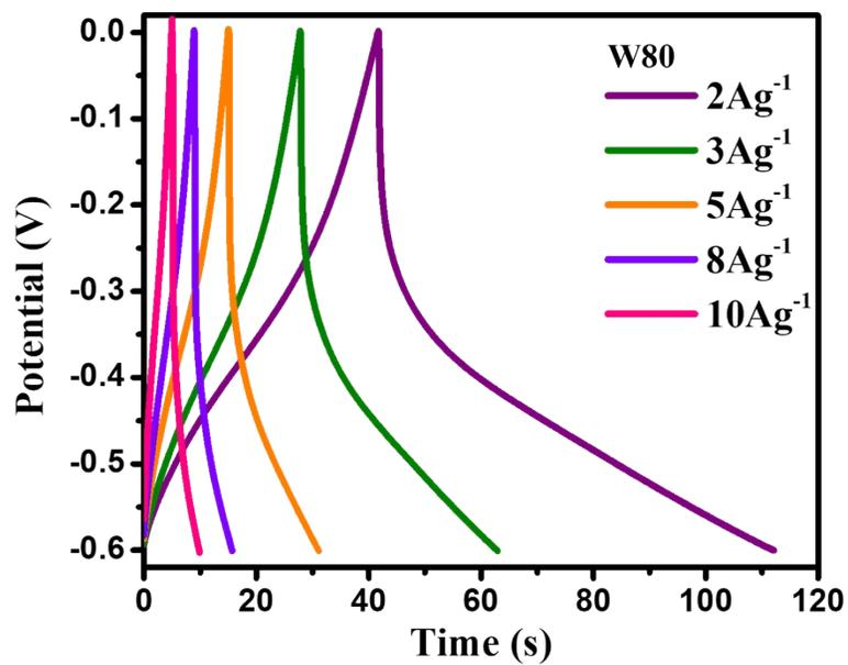
**Fig. S4.** Galvanostatics charge-discharge curves of W80 at various current densities.
