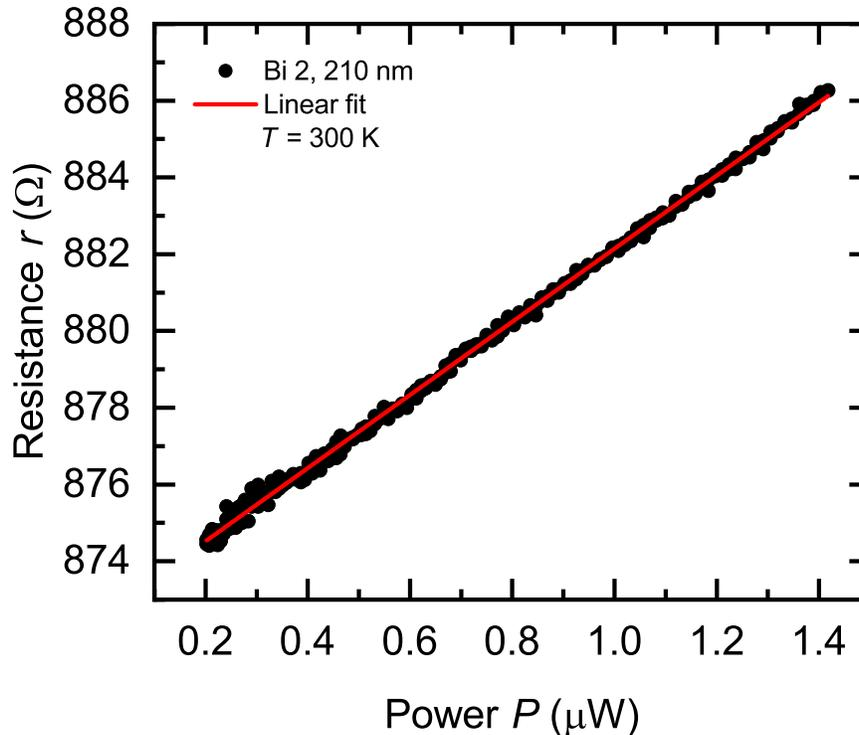
FIG. 2. **Resistance change of a Bi nanowire due to self-heating.** a, Four-terminal resistance  $r$  of Bi 2 (210 nm) as a function of the power  $P$  in the nanowire due to the applied current at  $T = 300$  K. The slope of the red line (linear fit) yields the relation between  $r$  and  $P$  that is used to determine the thermal conductivity.
