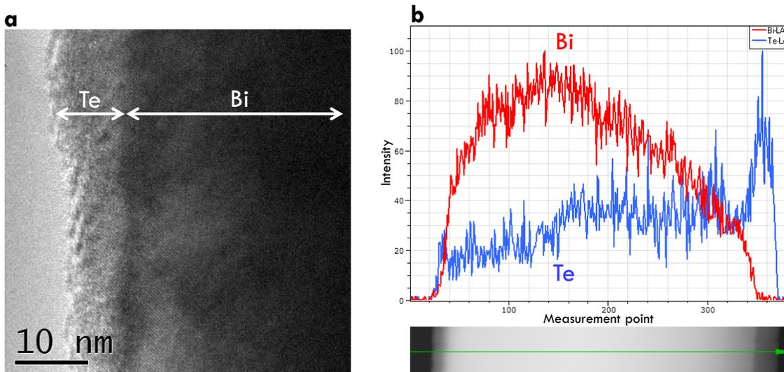
FIG. 4. **Structural properties of the Bi/Te core/shell nanowires.** a, Conventional transmission electron microscopy image that shows a section of the Bi/Te nanowire (Bi/Te 1 (370 nm)). b, Energy dispersive X-ray spectroscopy presenting the tellurium shell distribution of the Bi/Te core/shell nanowire (Bi/Te 1 (370 nm)).
