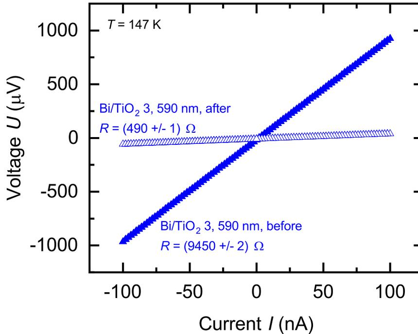
FIG. 3. **Resistance change of Bi/TiO<sub>2</sub> 3 (590, nm) due to lattice relaxation.** Measured voltage  $U$  of the nanowire before and after the lattice relaxation as a function of the applied current  $I$ . The four-terminal resistance  $R$  of the nanowire is after the lattice relaxation 19 times smaller than before.
