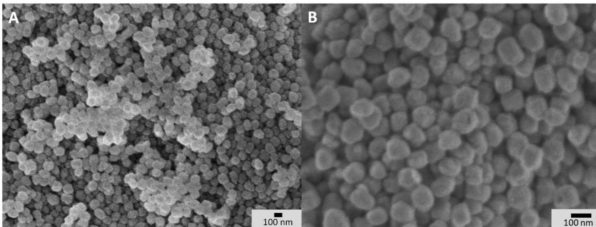
**Figure S2.** A) SEM images of TS-1 nanocrystals. B) SEM images of Hybrid\_EPCs. Experimental conditions: powders were metallized with chromium. Image A) was measured at 5.0 kV and image B) was measured at 1.0 kV
