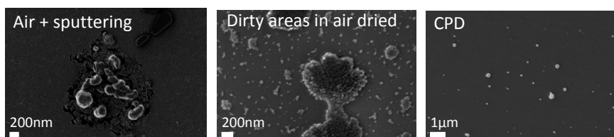
Figure S4. Representative images of additional substrates used to compare air drying with CPD. As shown, in the case of air drying, the wafers showed some dirty areas possibly arising from the drying process (middle image).
