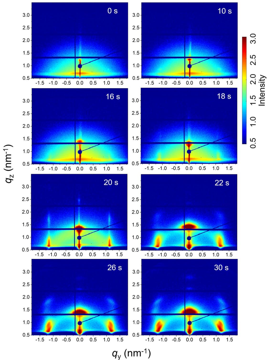
**Fig. S3.** Selected 2D GISAXS data at different times after deposition as indicated.
