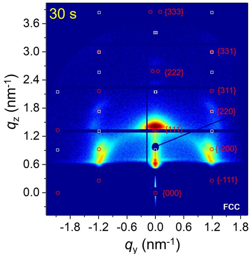
**Fig. S5.** 2D GISAXS image of printed film at  $t = 30$  s with predicted Bragg peak positions as indicated with white (reflected) and red (diffracted) points based on the FCC superlattice calculation with lattice parameters  $a = b = c = 8.6$  nm and  $\alpha = \beta = \gamma = 90^\circ$ .
