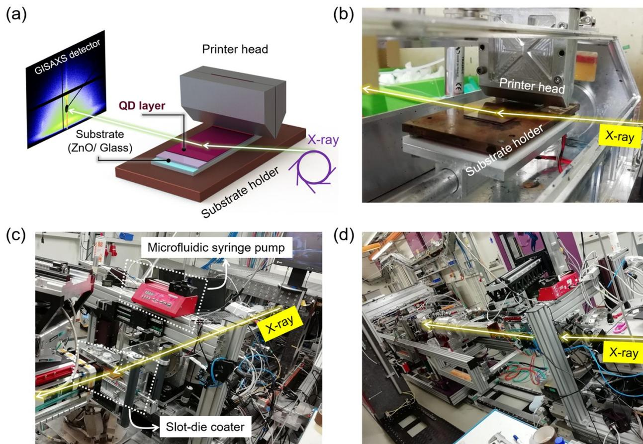
**Fig. S1.** Schematic (a) of the in-situ set-up used for printing and (b) the corresponding photograph with print head and substrate holder as indicated (X-ray beam is sketched for clarity). (c, d) Photographs of the integration of the slot-die coater in the experimental station P03.
