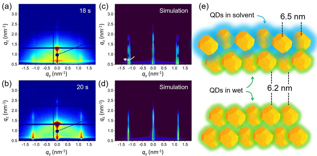
**Fig. S4.** (a,b) 2D GISAXS data and (c,d) respective simulated 2D images with BornAgain at (a,c)  $t = 18$  s and (b,d)  $t = 20$  s describing a templated stacking behavior of QDs. In the BornAgain simulation, a lattice length of 6.5 nm and 6.2 nm in a hexagonal layout is used to describe the scattering peaks at small and larger  $q_y$  values, respectively. (e) The corresponding schematics for describing the changes of inter-dot distances at  $t = 18$  s (top) and  $t = 20$  s (bottom).
