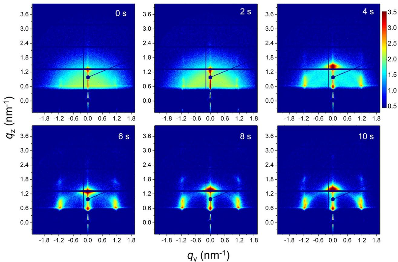
**Fig. S9.** 2D GISAXS data of QDs film deposited on a different substrate (ZnO/ITO/glass) by printing with the same protocol as used for the printing on ZnO/glass substrate at times as indicated. Times are not exactly compatible with the printing experiment described in the main manuscript due to additional alignment before the measurement. The observed superlattice structure evolution indicates similar QD stacking kinetics.
