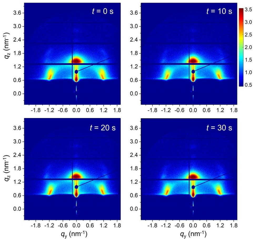
**Fig. S8.** 2D GISAXS data from the beam damage check performed after the X-ray measurement. The GISAXS data are taken at exactly the same positions corresponding to the GISAXS in situ measurements during the printing at times as indicated.
