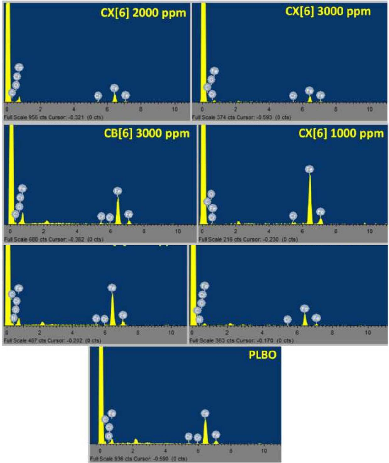
Figure S13. EDAX Elemental Analysis of Worn Surface
