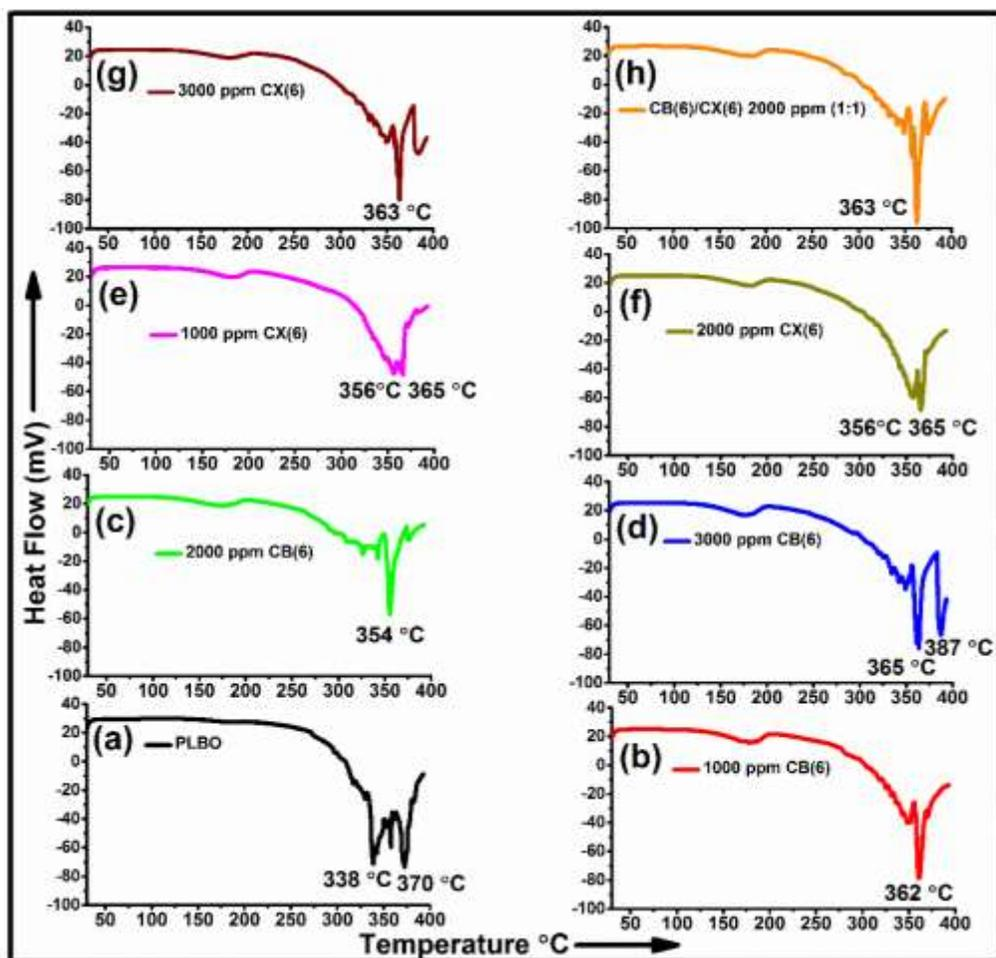
**Figure S9.** Showing Oxidation Stability by DSC with neat PLBO and PLBO spiked with various concentrations of CB[6] and CX[6]. (a) Blank PLBO, (b) CB[6] 1000 ppm, (c) CB[6] 2000 ppm, (d) CB[6] 3000 ppm, (e) CX[6] 1000 ppm, (f) CX[6] 2000 ppm, (g) CX[6] 3000 ppm (h) CB[6]/CX[6] 2000 ppm (1:1).
