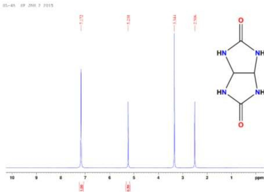
**Figure S2.** Showing <sup>1</sup>HNMR results of Glycouril in DMSO-d<sub>6</sub> (2.506 δ), 5.238 δ (S, 2H), 7.172 (S,4H).
