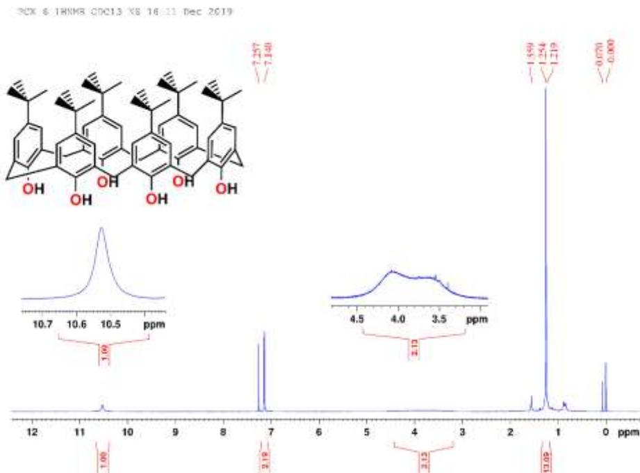
**Figure S5.** Showing CX[6]  $^1\text{H}$ NMR (500 MHz,  $\text{CDCl}_3$ ) :  $^1\text{H}$  NMR ( $\text{CDCl}_3$ )  $\delta$ : 1.25 (s, 54 H), 3.69 (s, 12 H), 7.14 (s, 12 H), 10.533 (s, 6 H). Locked in  $\text{CDCl}_3$ .
