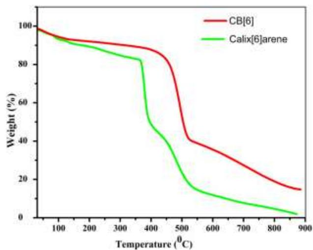
**Figure S15.** TGA curve of CB[6] and CX[6] showing their high-temperature stability
