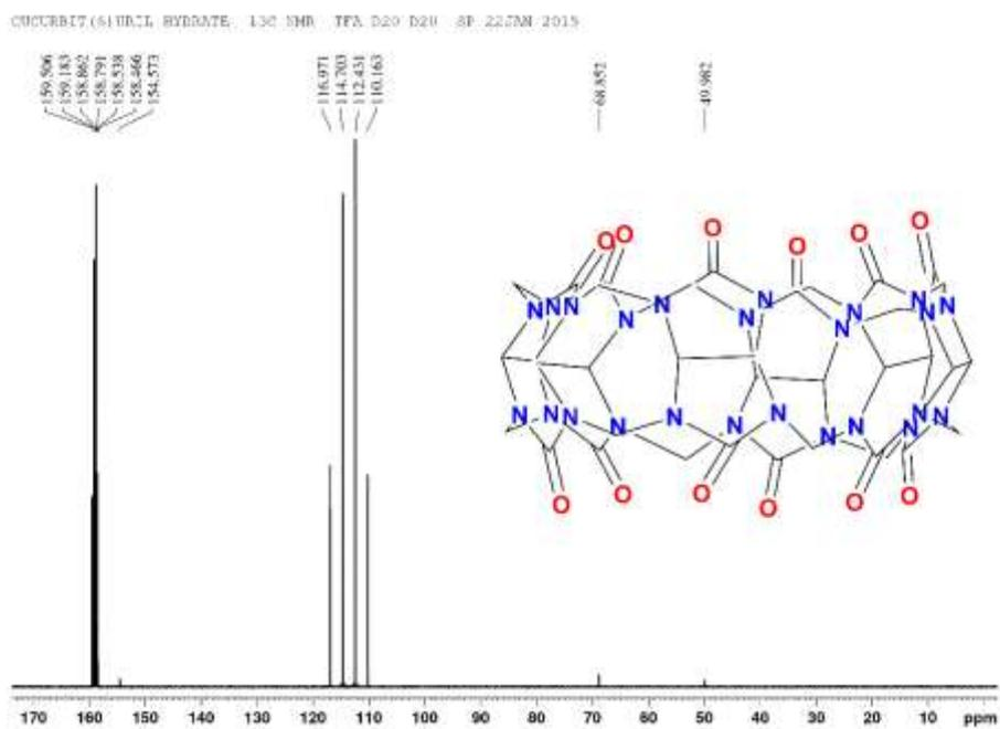
**Figure S4.** Showing CB[6]  $^{13}\text{C}$ NMR (500 MHz,  $\text{D}_2\text{O}/\text{CF}_3\text{-CO}_2\text{D}$  (1:1) : 154.57  $\delta$  (12C), 68.852  $\delta$  (12C), 49.982  $\delta$  (12C). Locked in  $\text{D}_2\text{O}$ .
