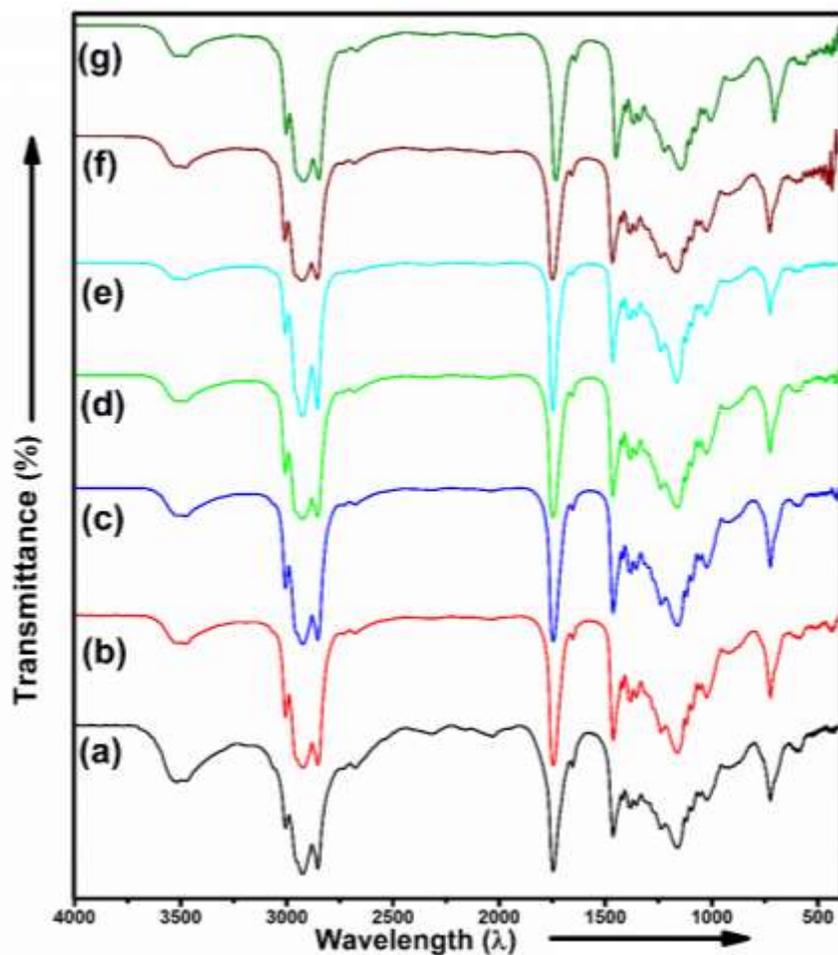
**Figure S7.** Showing Oxidation Stability by FTIR with neat PLBO and PLBO spiked with various concentrations of CB[6] and CX[6] before oxidation (a) Blank PLBO, (b) CB[6] 1000 ppm, (c) CB[6] 2000 ppm, (d) CB[6] 3000 ppm, (e) CX[6] 1000 ppm, (f) CX[6] 2000 ppm, (g) CX[6] 3000 ppm.
