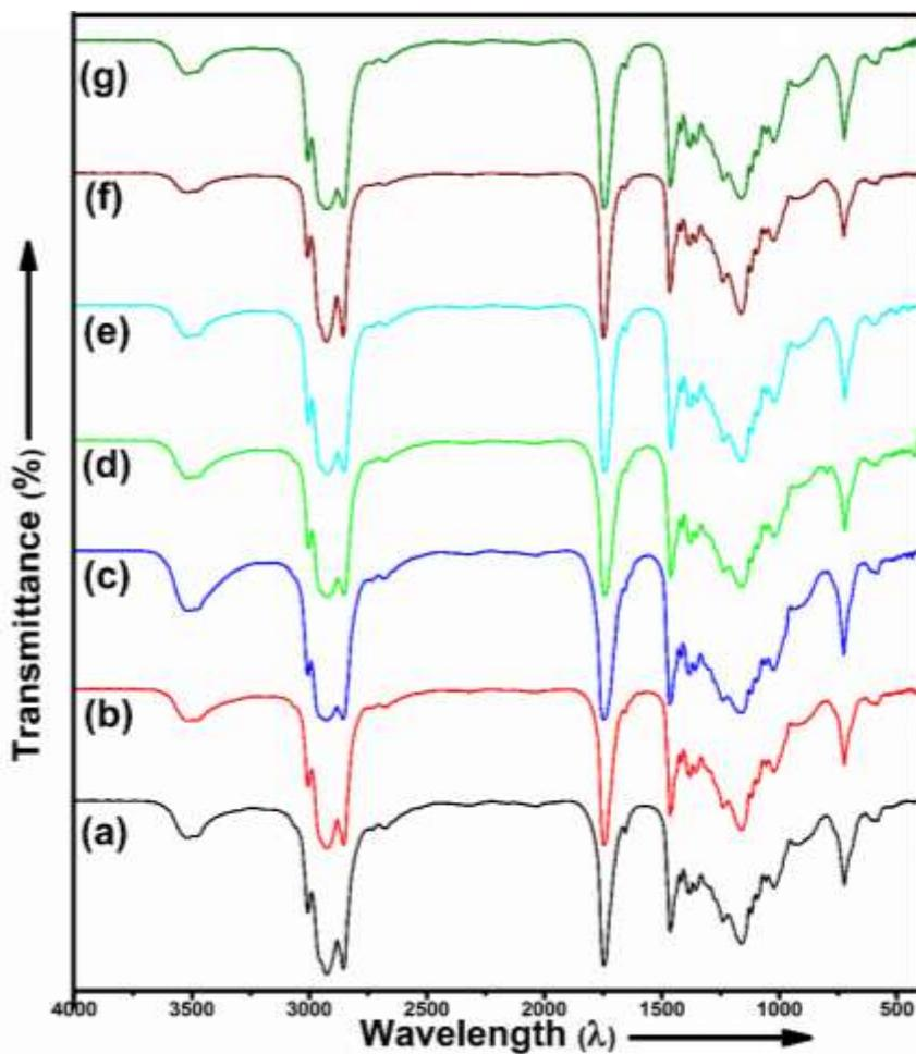
**Figure. S8.** Showing Oxidation Stability by FTIR with neat PLBO and PLBO spiked with various concentrations of CB[6] and CX[6] after Oxidation (a) Blank PLBO, (b) CB[6] 1000 ppm, (c) CB[6] 2000 ppm, (d) CB[6] 3000 ppm, (e) CX[6] 1000 ppm, (f) CX[6] 2000 ppm, (g) CX[6] 3000 ppm.
