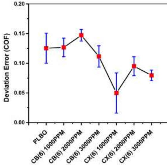
**Figure S11.** Showing mean and standard deviation for repetitive experiments of COF ( Coefficient of Friction Four ball test ASTM D4172 ).
