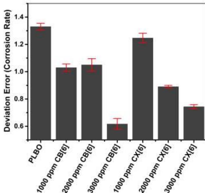
**Figure S14.** Showing mean and standard deviation for repetitive experiments of AC ( Anticorrosion Study Four ball test ASTM D4172 ).
