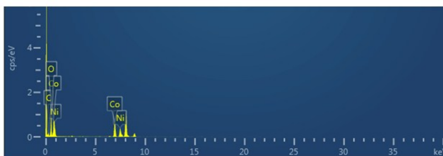
Fig. S8 The EDX spectrum of NC-LDHs/LIG.
