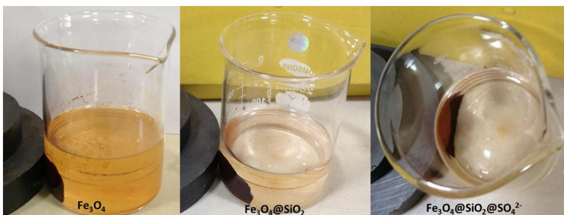
Fig. ESI-1. Magnetic separation with external magnet during preparation of magnetic catalyst.
