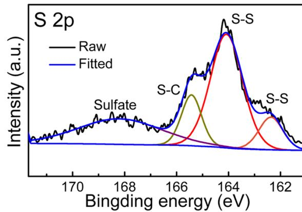
**Fig. S6** High-resolution XPS spectra of S 2p in S/Co, N@CPDA-HCS.
