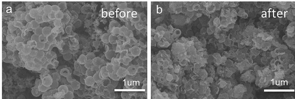
**Fig. S8** SEM images of S/Co, N@CPDA-HCS before (a) and after (b) cycling.
