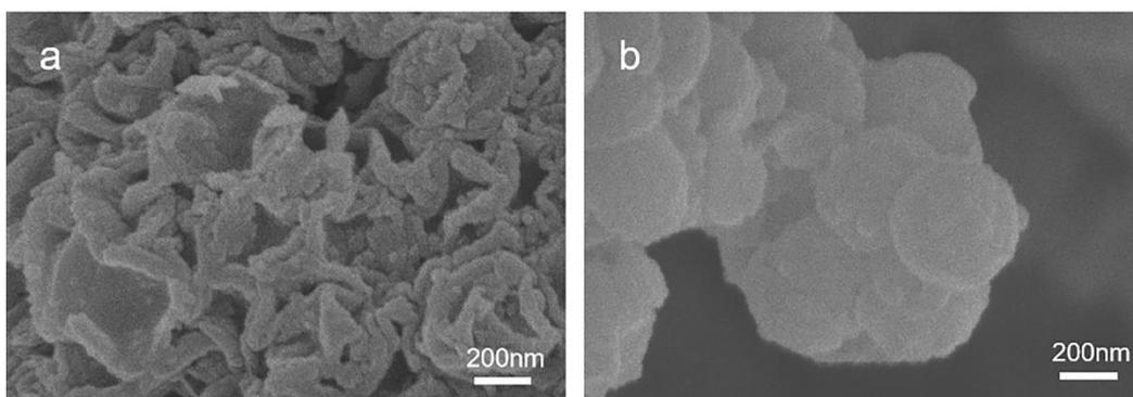
**Fig. S2** SEM images of (a) the S/N@CPDA and (b) S/Co, N@CPDA-HCS.
