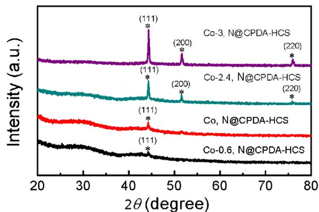
**Fig. S3** XRD patterns of Co-0.6, N@CPDA-HCS, Co, N@CPDA-HCS, Co-2.4, N@CPDA-HCS and Co-3, N@CPDA-HCS.
