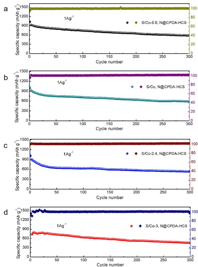
**Fig. S9** Cycling performances of (a) S/Co-0.6, N@CPDA-HCS, (b) S/Co, N@CPDA-HCS, (c) S/Co-2.4, N@CPDA-HCS and (d) S/Co-3, N@CPDA-HCS tested at a current density of 1A g<sup>-1</sup>.
