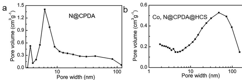
**Fig. S5** Aperture distribution curve of (a) N@CPDA and (b) Co, N@CPDA-HCS.
