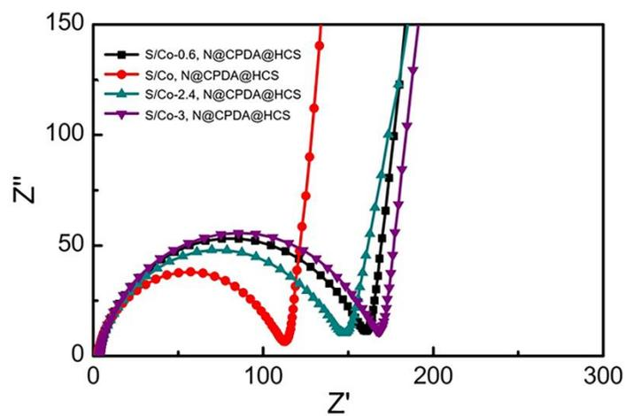
**Fig. S10** EIS plots of the S/Co-0.6, N@CPDA-HCS, S/Co, N@CPDA-HCS, S/Co-2.4, N@CPDA-HCS and S/Co-3, N@CPDA-HCS.
