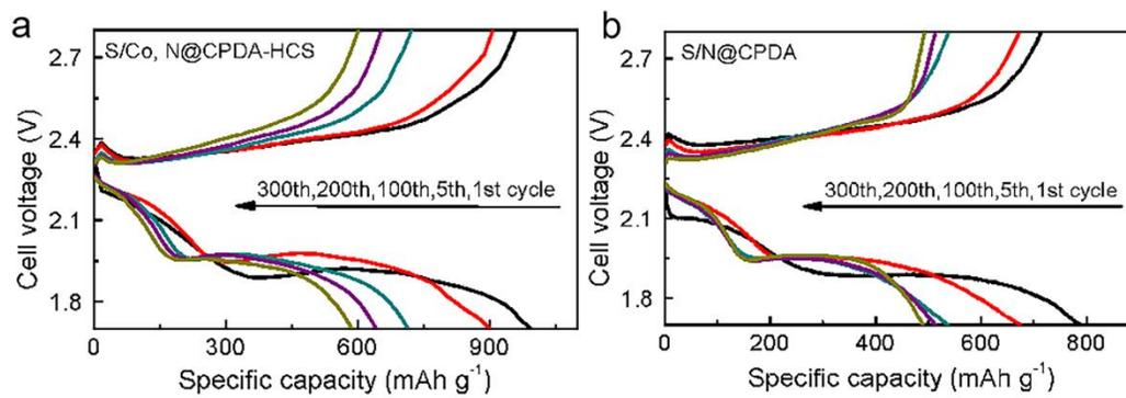
**Fig. S7** Charge and discharge voltage profiles of (a) S/Co, N@CPDA-HCS and (b) S/N@CPDA.
