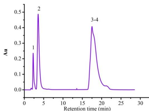
**Fig. S7** Separation of test mixtures of SDM (1); SM2 (2); SG (3) and SST (4) on 0.1g-NIPAM@Sil column. The chromatographic condition same as Fig. 7a.
