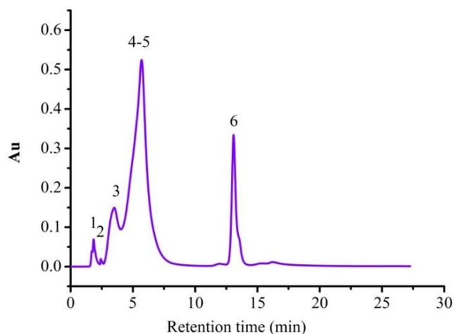
**Fig. S6** Separation of test mixtures of sanguinarine (1); theophylline (2); colchicines (3); berberine hydrochloride (4); palmatine hydrochloride (5); jatrorrhizine (6) on 0.1g-NIPAM@Sil column. The chromatographic condition same as Fig 6.
