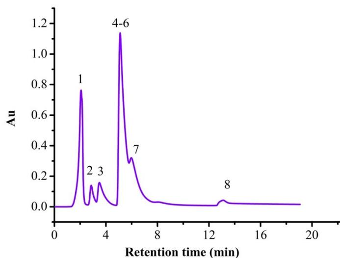
**Fig. S4** Separation of test mixtures of 6-chlorouracil (1), thymidine (2); uridine (3); inosine (4); guanine (5); adenine (6); cytidine (7); cytosine (8) on 0.1g-NIPAM@Sil column. The chromatographic condition same as Fig 5.
