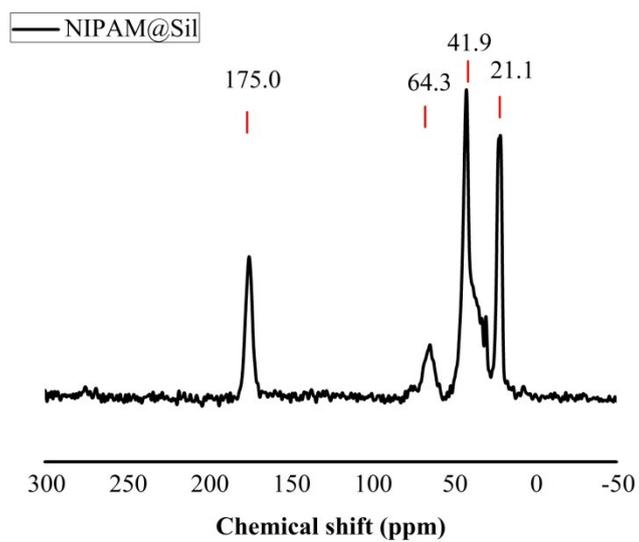
**Fig. S3** Solid-state  $^{13}\text{C}$  NMR spectrum of NIPAM@Sil.
