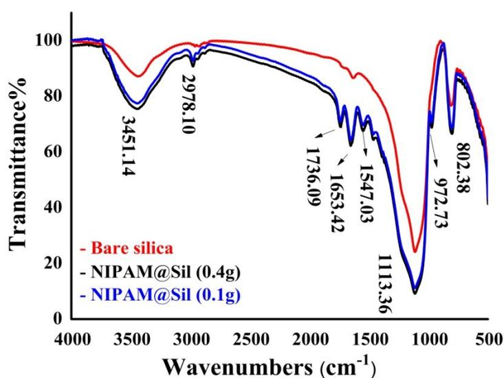
**Fig. S1** IR spectra of Bare silica, NIPAM@Sil (0.1g) and NIPAM@Sil (0.4g).
