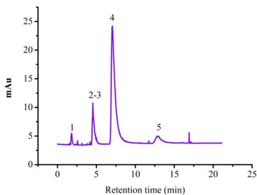
**Fig. S8** Separation of test mixtures of D-ribose (1); D-fructose (2); sucrose (3); lactulose (4) and triaccharide (5) on 0.1g-NIPAM@Sil column. The chromatographic condition same as Fig. 7b.
