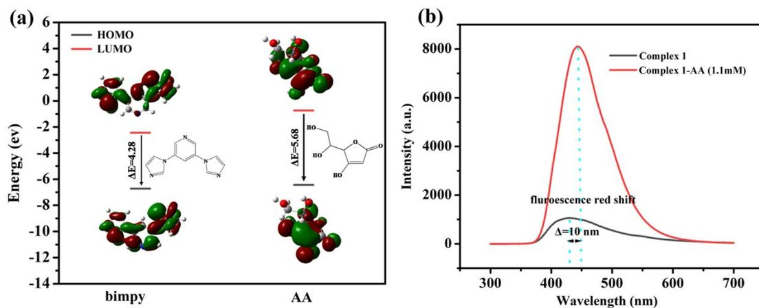
**Fig. S10** (a) HOMO–LUMO energy levels of bimpy ligand and AA. (b) Fluorescence intensity of complex **1** before and after adding AA.
