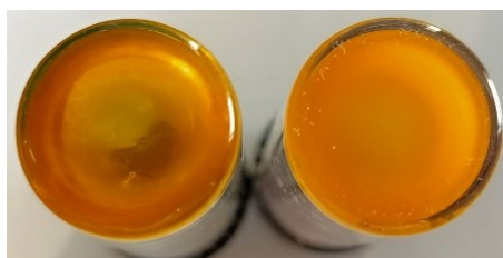
Figure S10. The transparency changes of toluene gel before and after adsorption of rhodamine B.
