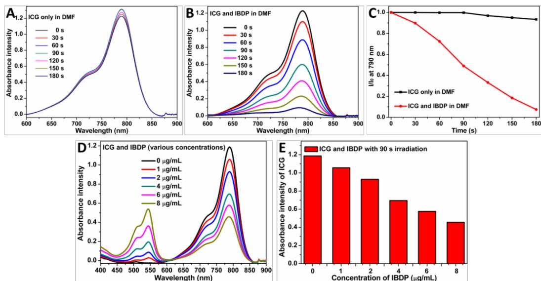
**Figure S4.** A-B) Singlet oxygen generation by IBDP in DMF monitored by disappearance of UV absorbance of ICG with an LED light power density of 20 mW/cm<sup>2</sup> over 180 seconds. C) The quantification of the  $^1\text{O}_2$  generation ability of ICG blank (black), IBDP (red). D) Singlet oxygen generation by IBDP with different concentrations in DMF monitored by disappearance of UV absorbance of ICG with an LED light power density of 20 mW/cm<sup>2</sup> for 90 seconds.
