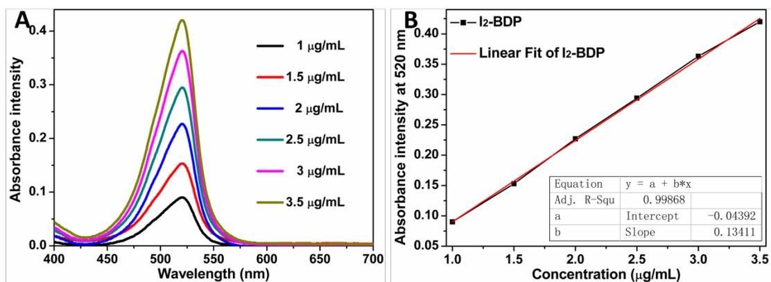
**Figure S1.** A) and B) Standard absorbance curve of IBDP. (The absorbance of IBDP molecules at 520 nm (from a mixture of acetone and water (v/v = 4:1)) as a function of IBDP concentration.)
