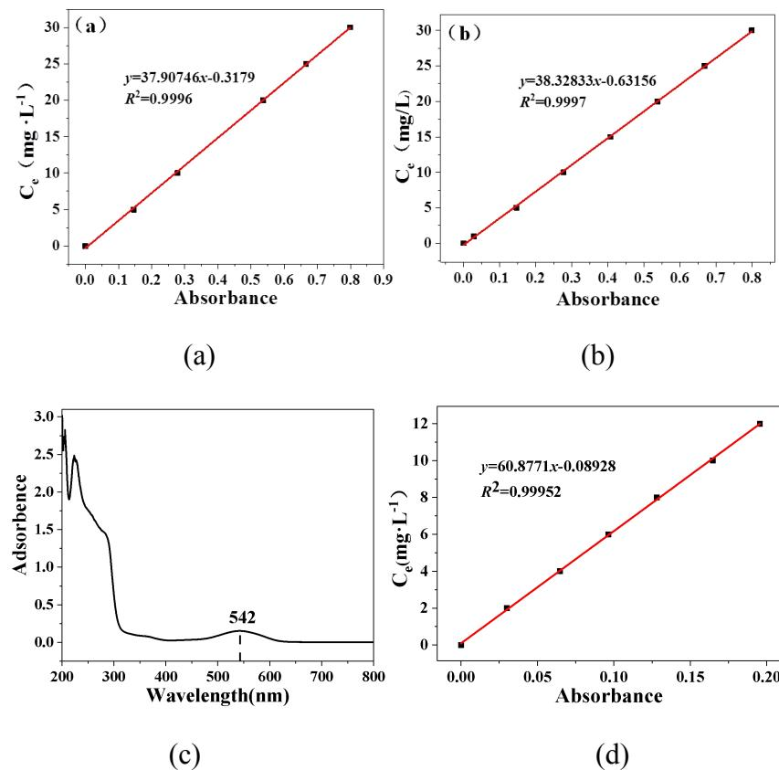
Fig. S5. (a) the standard curve of TC at pH 6.80; (b) the standard curve of TC at pH 3.80; (c) The UV spectra of Cr(VI) solution; (d) the standard curve of Cr(VI).
