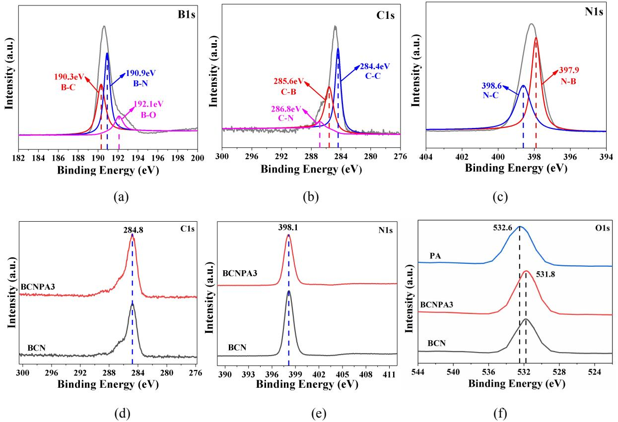
Fig. S9. (a) the B1s spectra of BCN; (b) the C1 spectra of BCN; (c) the N1s spectra of BCN; (d) the C1s spectra of BCN and BCNPA3; (e) the N1s spectra of BCN and BCNPA3; (f) the O1s spectra of PA , BCN and BCNPA3.
