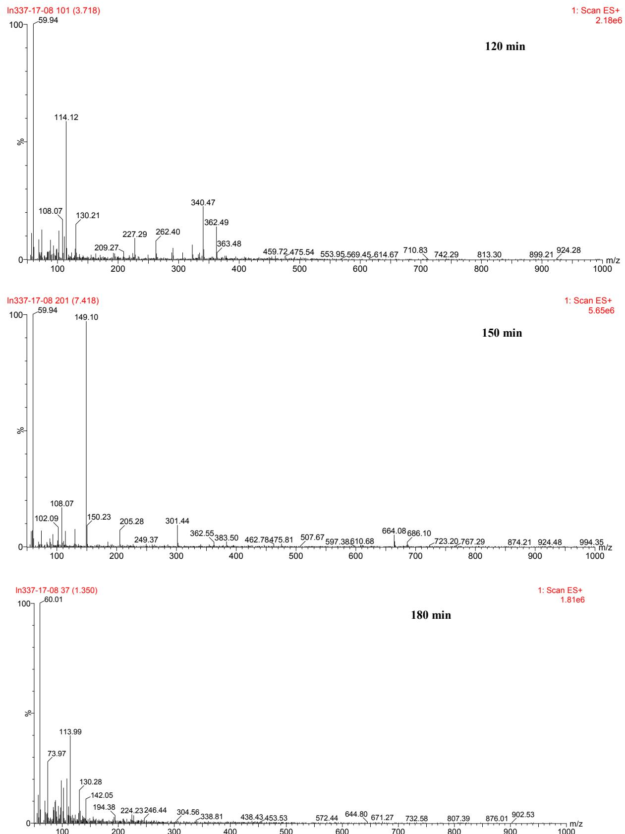
Fig. S22. LC-MS chromatogram of TC transformation intermediates in TC/Cr(VI) solution at different reaction time.
