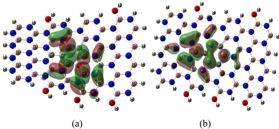
Fig. S11. (a) HOMO orbital of BCN model; (b) LUMO orbital of BCN model.
