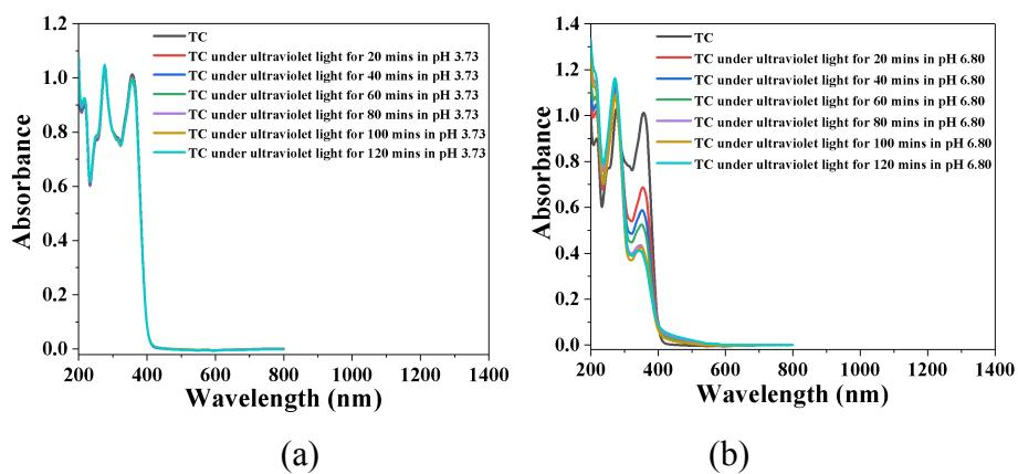
Fig. S17. (a) UV-visible spectra of TC photodegradation under ultraviolet light irradiation at pH 3.73 (concentration:  $30 \text{ mg} \cdot \text{L}^{-1}$ , volume: 100 mL); (b) UV-visible spectra of TC photodegradation under ultraviolet light irradiation at pH 6.80 (concentration:  $30 \text{ mg} \cdot \text{L}^{-1}$ , volume: 100 mL).
