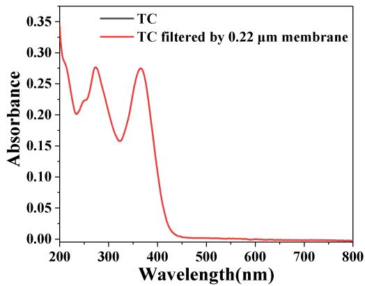
Fig. S6. The UV spectra of TC solution before and after filtration by 0.22  $\mu\text{m}$  membrane.
