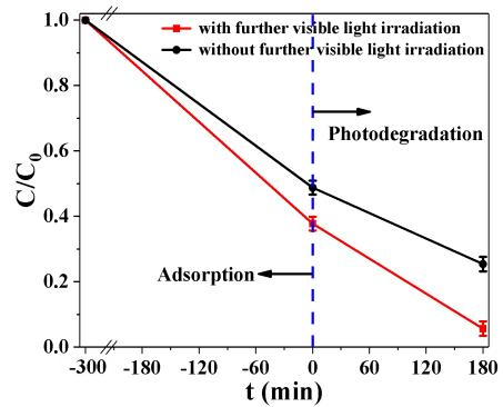
Fig. S23. The test for why BCNPA3 need a further irradiation treatment after the adsorption and photodegradation experiment (dosage: 25 mg, TC/Cr(VI) concentration: 30/10 mg·L<sup>-1</sup>, volume: 100 mL).
