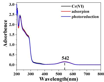
Fig. S19. The UV-visible spectra of single Cr(VI) solution after adsorption for 300 minutes and photoreduction under visible light irradiation for 180 minutes by BCNPA3.
