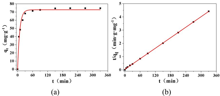
Fig. S13. (a) The pseudo-first-order kinetic adsorption of TC by BCNPA3; (b) the pseudo-second-order kinetic adsorption of TC by BCNPA3.
