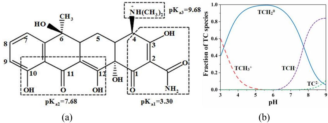
Fig. S1. (a) The structure of tetracycline (TC), the dotted areas represent the structural moieties associated with the three acidic dissociation constants ( $pK_a$ ); (b) speciation distributions of TC in different pH values.
