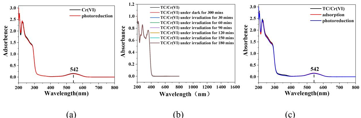
Fig. S20. (a) UV-visible spectra of Cr(VI) under visible light irradiation for 180 mins via diphenylcarbazide spectrophotometric method (Cr(VI) concentration:  $10 \text{ mg}\cdot\text{L}^{-1}$ , volume: 100mL, photodegradation time: 180 minutes); (b) The UV-visible spectra of TC adsorption and
