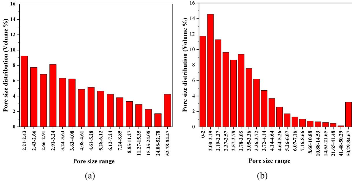
Fig. S10. (a) the pore size distribution of BCN; (b) the pore size distribution of BCNPA3.
