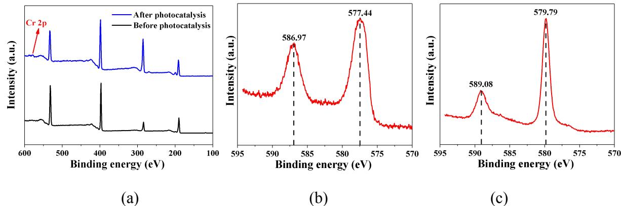
Fig. S21. (a) XPS spectra of BCNPA3 before and after simultaneous photocatalytic redox conversion of TC and Cr(VI) system; (b) High-resolution XPS spectrum of standard Cr(III) samples( $\text{CrCl}_3 \cdot 6\text{H}_2\text{O}$ ); (c) High-resolution XPS spectrum of standard Cr(VI) samples( $\text{K}_2\text{Cr}_2\text{O}_7$ ).
