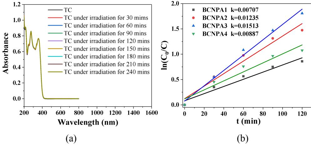
Fig. S8. (a) the UV-vis spectra of TC at different time scales under visible light irradiation for 180mins. The time scales are 30 mins, 60 mins, 90 mins, 120 mins, 150 mins, 180 mins, 210 mins and 240 mins, respectively; (b) the kinetic curves data of TC photo-removal by different BCNPA composites under visible light irradiation.
