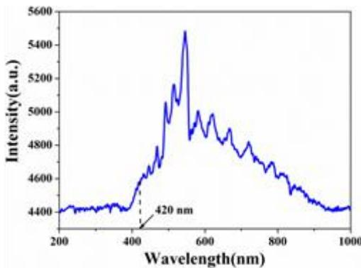
Fig. S16. The light spectrum of visible light source that used in the photo-removal experiments of TC by BCNPA3 under visible light irradiation. A 420 nm filter is used during whole irradiation process.
