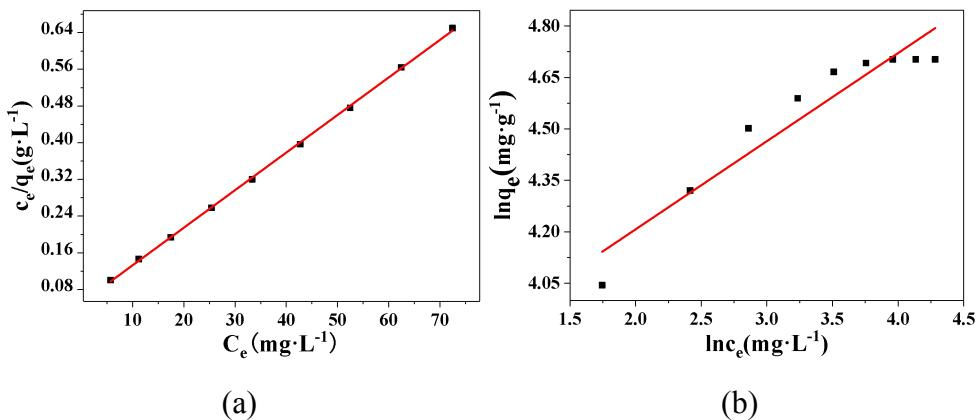
Fig. S14. (a) the Langmuir isotherm adsorption curve of TC by BCNPA3; (b) the Freundlich isotherm adsorption curve of TC by BCNPA3.
