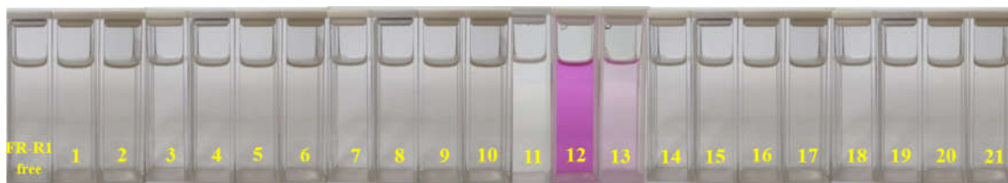
Fig. S11. Color changes of FR-R1 (10 \mu\text{M} ) in \text{H}_2\text{O}/\text{THF} (4:1, v/v) with different metal ions (50 \mu\text{M} ) under visible light, where 1-21 are \text{Li}^+ , \text{Na}^+ , \text{K}^+ , \text{Cs}^+ , \text{Mg}^{2+} , \text{Ca}^{2+} , \text{Sn}^{2+} , \text{Pb}^{2+} , \text{Ag}^+ , \text{Zn}^{2+} , \text{Cd}^{2+} , \text{Hg}^{2+} , \text{Cu}^{2+} , \text{Fe}^{2+} , \text{Fe}^{3+} , \text{Co}^{2+} , \text{Ni}^{2+} , \text{La}^{3+} , \text{Ce}^{3+} , \text{Nd}^+ , and \text{Eu}^{3+} , respectively.
