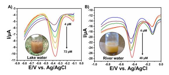
DPV response of RGO@CuO@Mn<sub>2</sub>O<sub>3</sub> modified electrode for each sequential additions of real samples containing 2-NP into continuously stirred phosphate buffer (pH 7). A) Lake water and B) River water.
