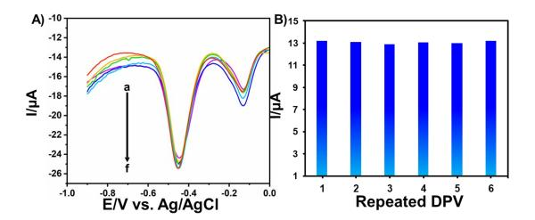
(A) DPV selective responses of a) nitrobenzene, b) catechol, c) hydroquinone, c) resorcinol, d) nitrite, e) mercury, and f) 4-NP at RGO@CuO@Mn<sub>2</sub>O<sub>3</sub>/GCE towards 100 μM of 2-NP. (B) Bar diagram of repeated DPV vs. current responses.
