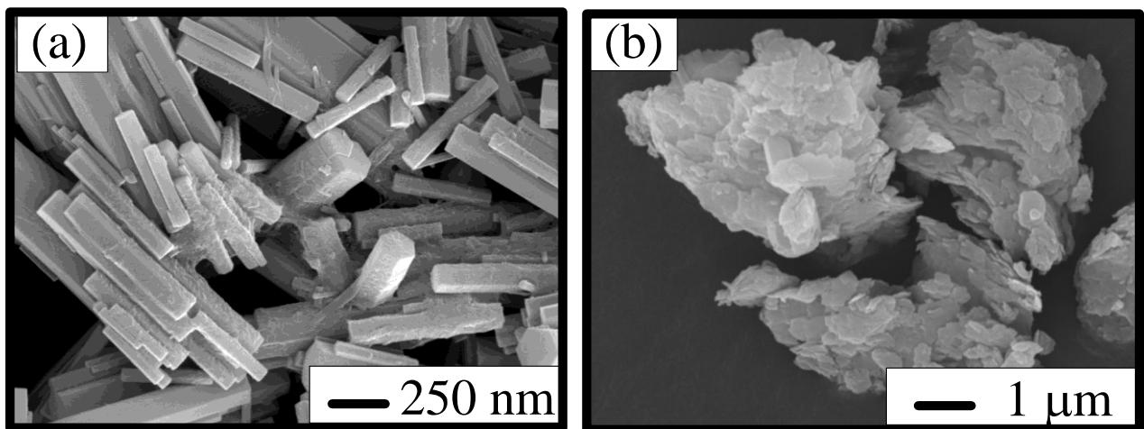
Figure S1. The SEM images of (a)  $h$ - $\text{MoO}_3$  and (b)  $\text{MoO}_3$ :BTA microcrystals
