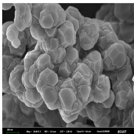
Figure S2. SEM image of pristine UiO-66.
