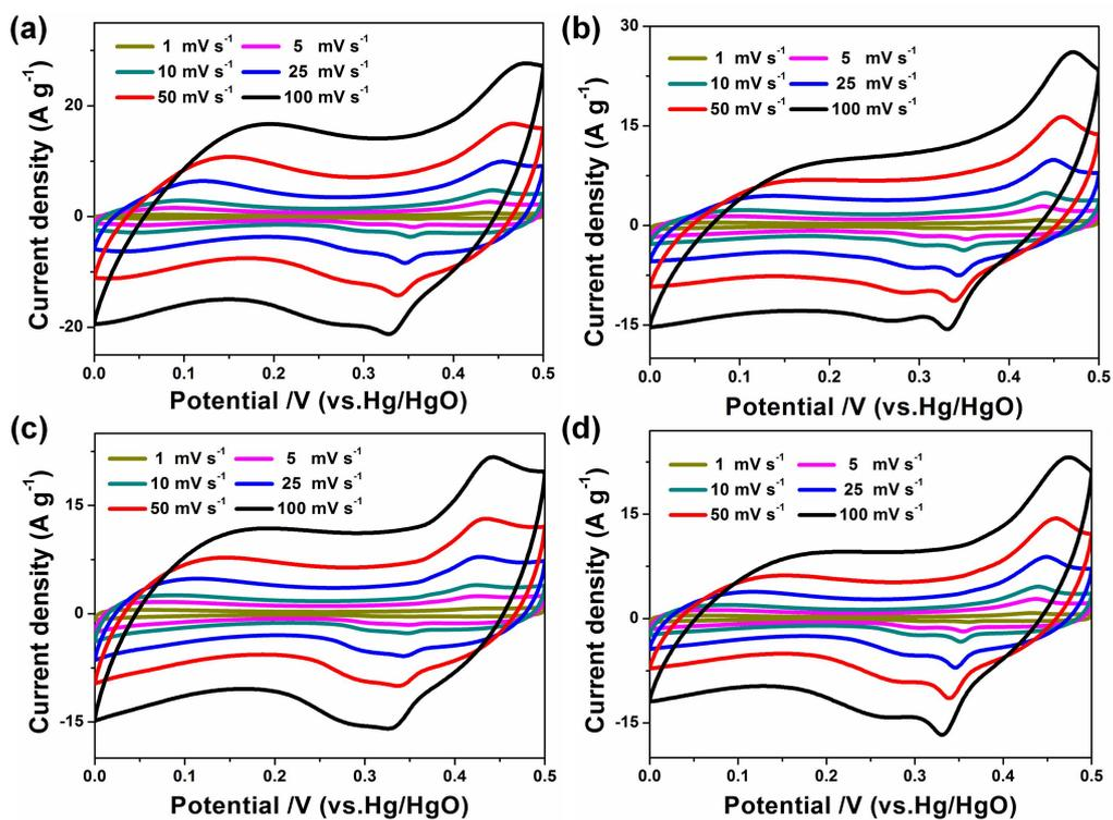
**Figure S9.** The CV curves of the Co<sub>2</sub>P<sub>2</sub>O<sub>7</sub>/C-600 (a), -700 (b), -800 (c) and -1000 (d) within the potential of 0-0.5 V (vs. Hg/HgO) at various scan rates.
