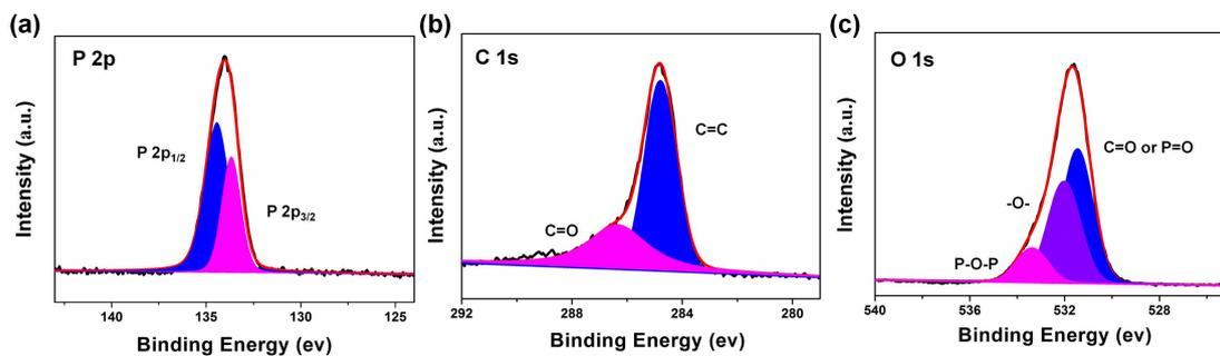
Figure S2. The P 2p spectra (a), C 1s spectra (b) and O 1s spectra (c) of  $\text{Co}_2\text{P}_2\text{O}_7/\text{C-900}$ .
