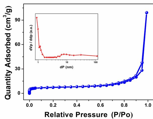
**Figure S5.** The  $\text{N}_2$  adsorption and desorption isotherms and pore size distribution curve of  $\text{Co}_2\text{P}_2\text{O}_7/\text{C-900}$ .
