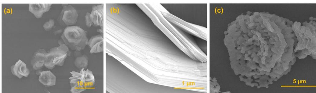
**Figure S3.** The SEM images of (a, b)  $\text{Co}(\text{PhPO}_3)$  and (c)  $\text{Co}_2\text{P}_2\text{O}_7\text{-900}$ .
