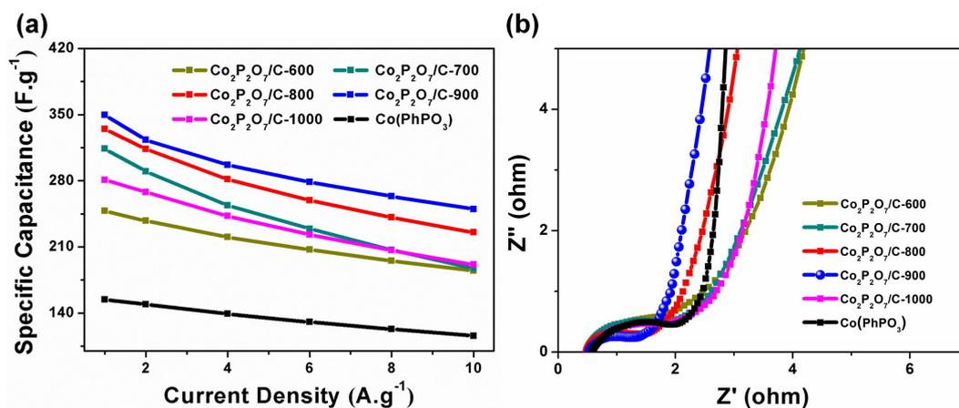
**Figure S11.** The specific capacitance (a) and the Nyquist plots (b) of  $\text{Co}_2\text{P}_2\text{O}_7/\text{C}-\text{X}$  and  $\text{Co}(\text{PhPO}_3)$ .
