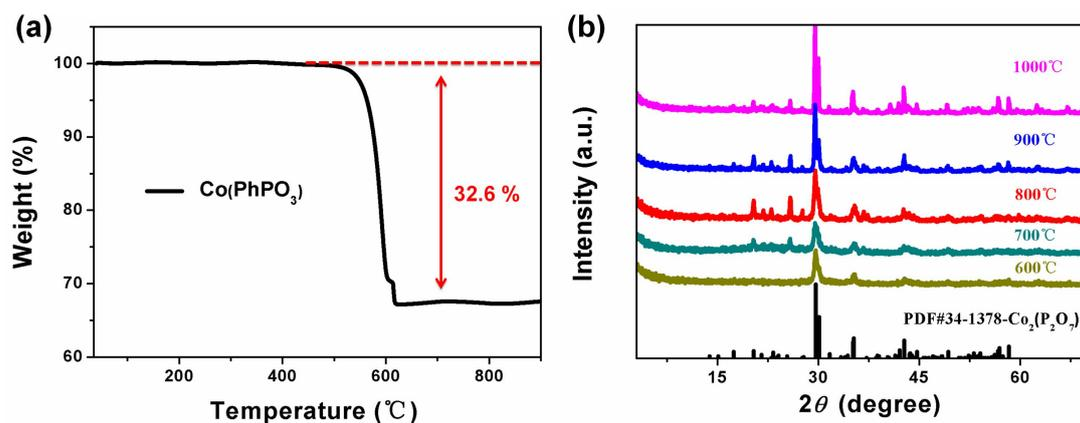
**Figure S6.** (a) The Thermogravimetric analysis of  $\text{Co(PhPO}_3\text{)}$  precursor. (b) The PXRD patterns of  $\text{Co}_2\text{P}_2\text{O}_7/\text{C}$ -600,  $\text{Co}_2\text{P}_2\text{O}_7/\text{C}$ -700,  $\text{Co}_2\text{P}_2\text{O}_7/\text{C}$ -800,  $\text{Co}_2\text{P}_2\text{O}_7/\text{C}$ -900 and  $\text{Co}_2\text{P}_2\text{O}_7/\text{C}$ -1000.
