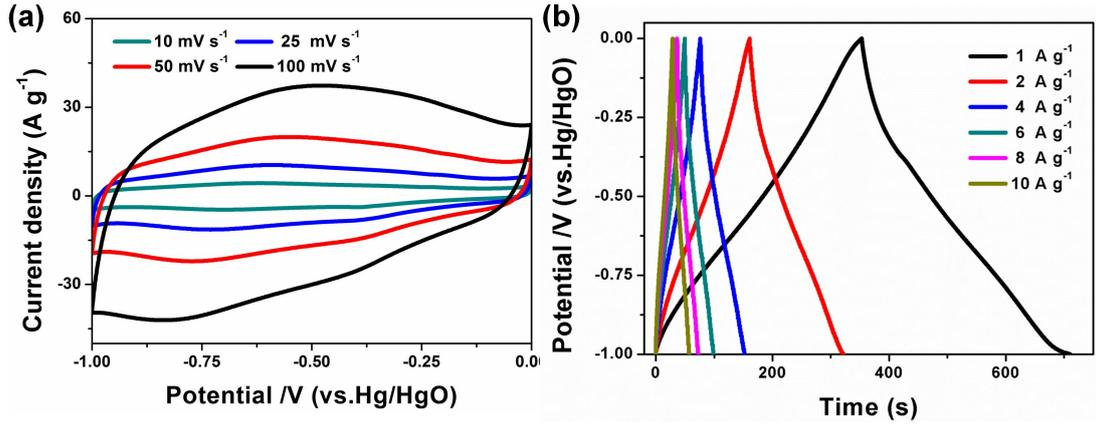
**Figure S12.** The CV (a) and GCD (b) curves of the 3DPG anode.
