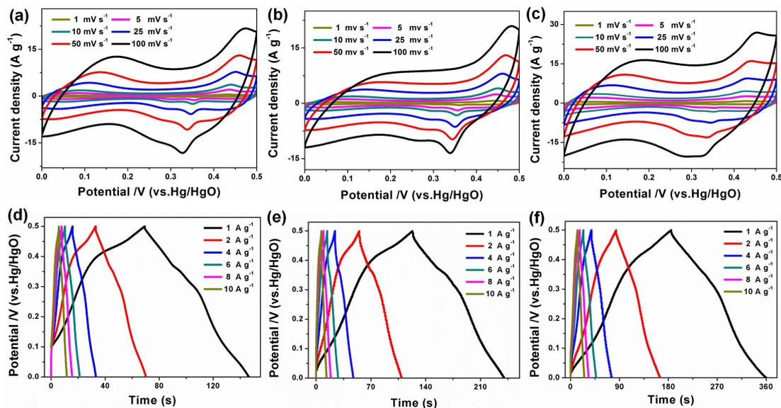
**Figure S7.** The CV curves (a), (b), (c) and GCD curves (d),(e), (f) of the  $\text{Co(PhPO}_3\text{)}$ ,  $\text{Co}_2\text{P}_2\text{O}_7$ -900 and  $\text{Co}_2\text{P}_2\text{O}_7/\text{C}$ -900.
