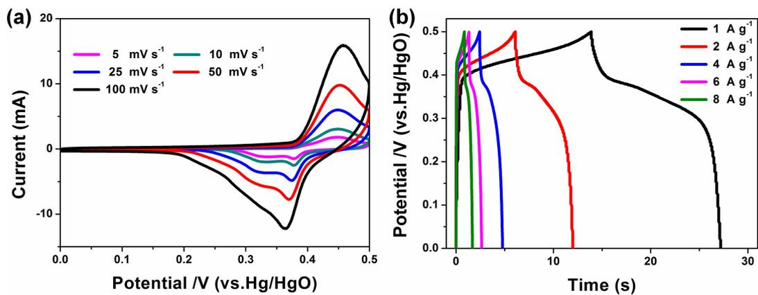
**Figure S8.** The electrochemical performance of Ni foam: (a) the CV curves (b) the GCD curves.
