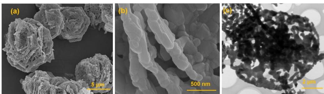
**Figure S4.** The SEM images (a, b) and TEM image (c) of  $\text{Co}_2\text{P}_2\text{O}_7/\text{C-900}$ .
