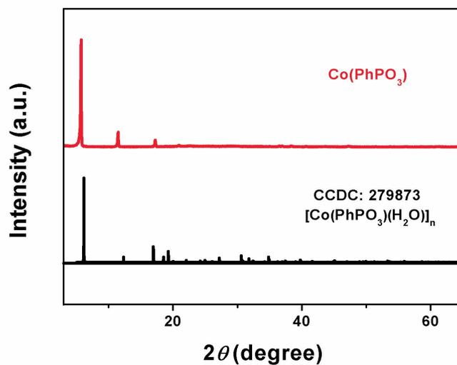
Figure S1. The PXRD patterns of  $\text{Co}(\text{PhPO}_3)$  and  $[\text{Co}(\text{PhPO}_3)(\text{H}_2\text{O})]_n$ .
