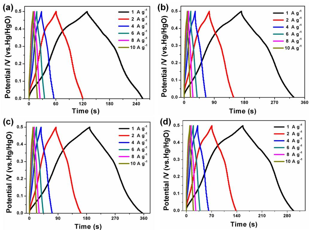
**Figure S10.** The GCD curves of the  $\text{Co}_2\text{P}_2\text{O}_7/\text{C}-600$  (a),  $-700$  (b),  $-800$  (c) and  $-1000$  (d) at various current densities.
