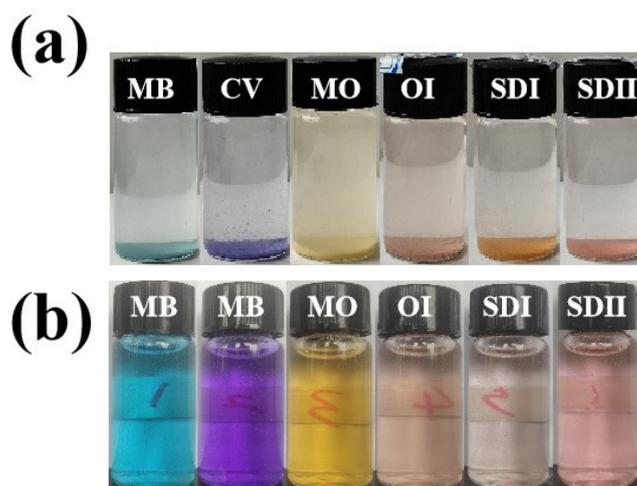
**Figure S26** (a) The adsorption separation of various organic dyes by NT; (b) The adsorption separation of various organic dyes by NBP5.
