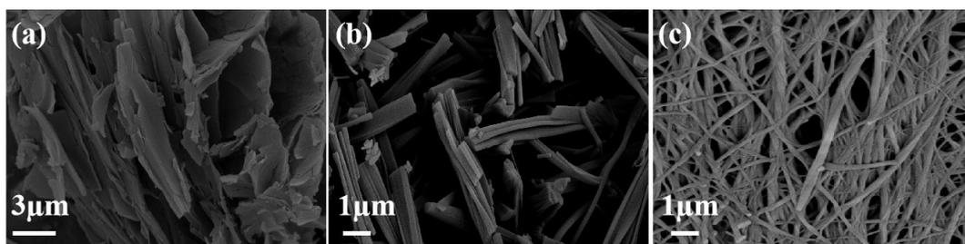
**Figure S19** SEM images of xerogel (a) NBP5; (b) TG; (c) NT
